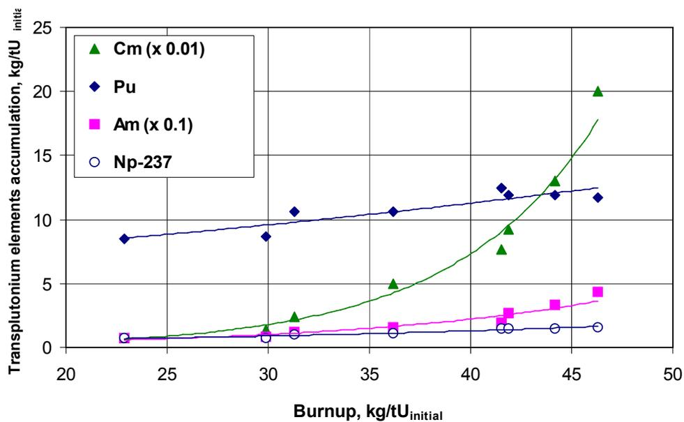
Fig. 1.9 Transplutonium elements accumulation as a function of fuel burnup.
