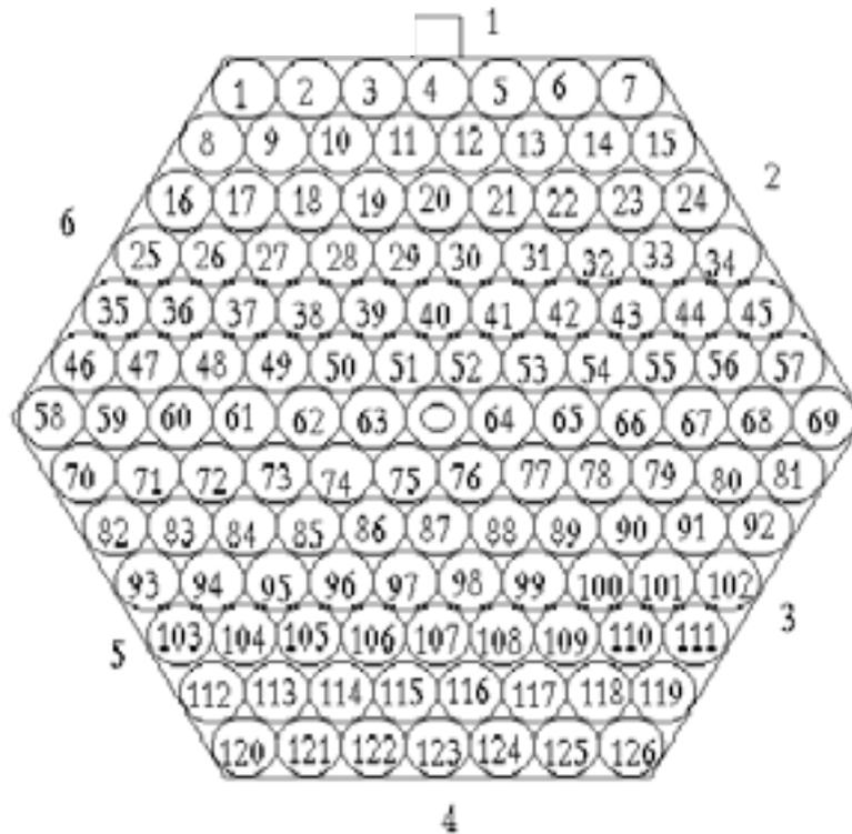
*Fig. 1.1 Schematic arrangement of fuel rods in FA No. 135.*
