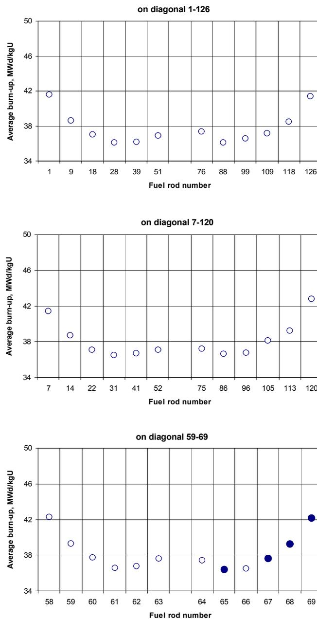
Fig. 1.3. Distribution of the average burnup in diagonal directions of FA No.13626135 fuel rods.
