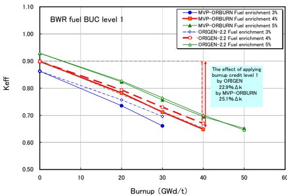
FIG. 12. Differences between the initial enrichment and the burnup credit level 1 calculation for BWR fuel.
