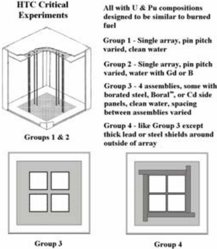
FIG. 2. French HTC critical experiments.
