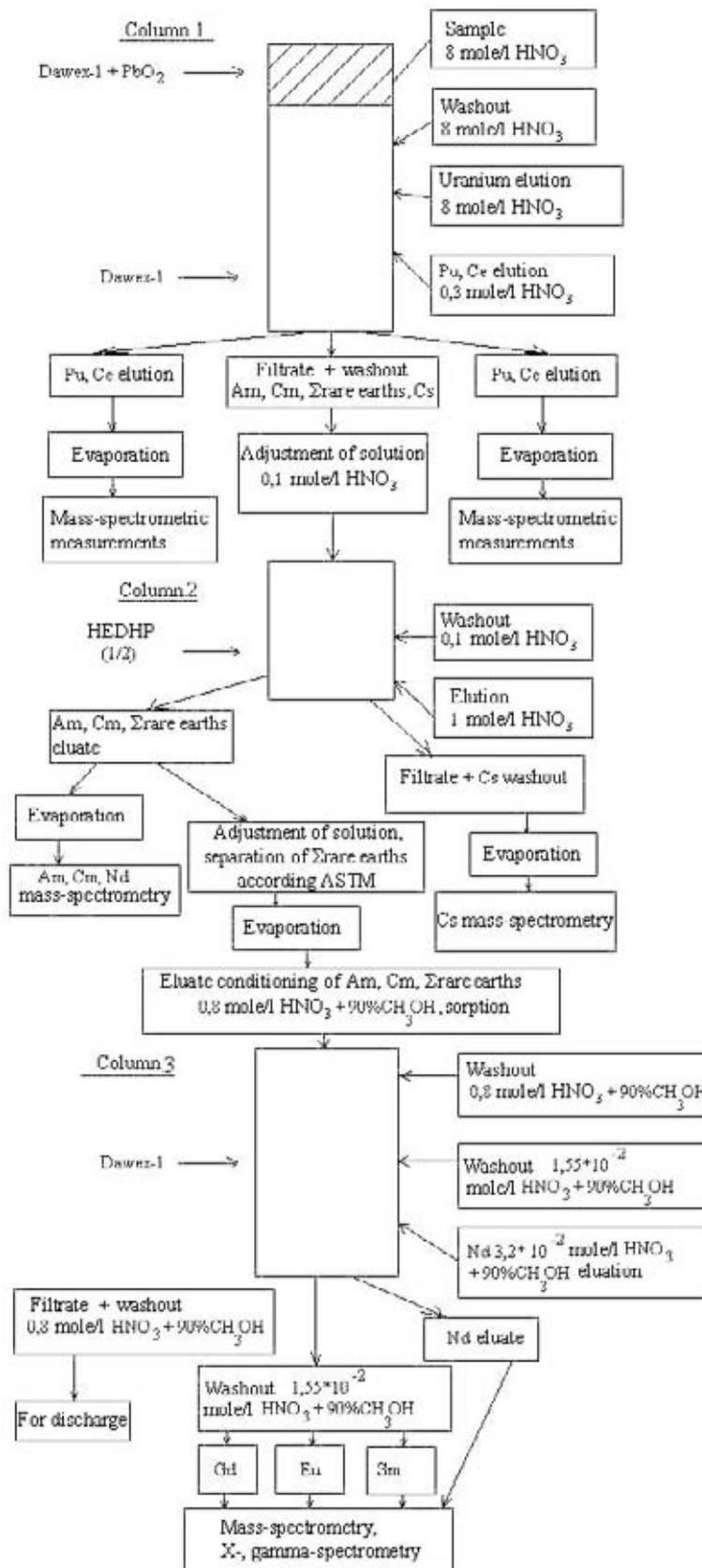
Fig. 1.7 Scheme of radiochemical extraction.
