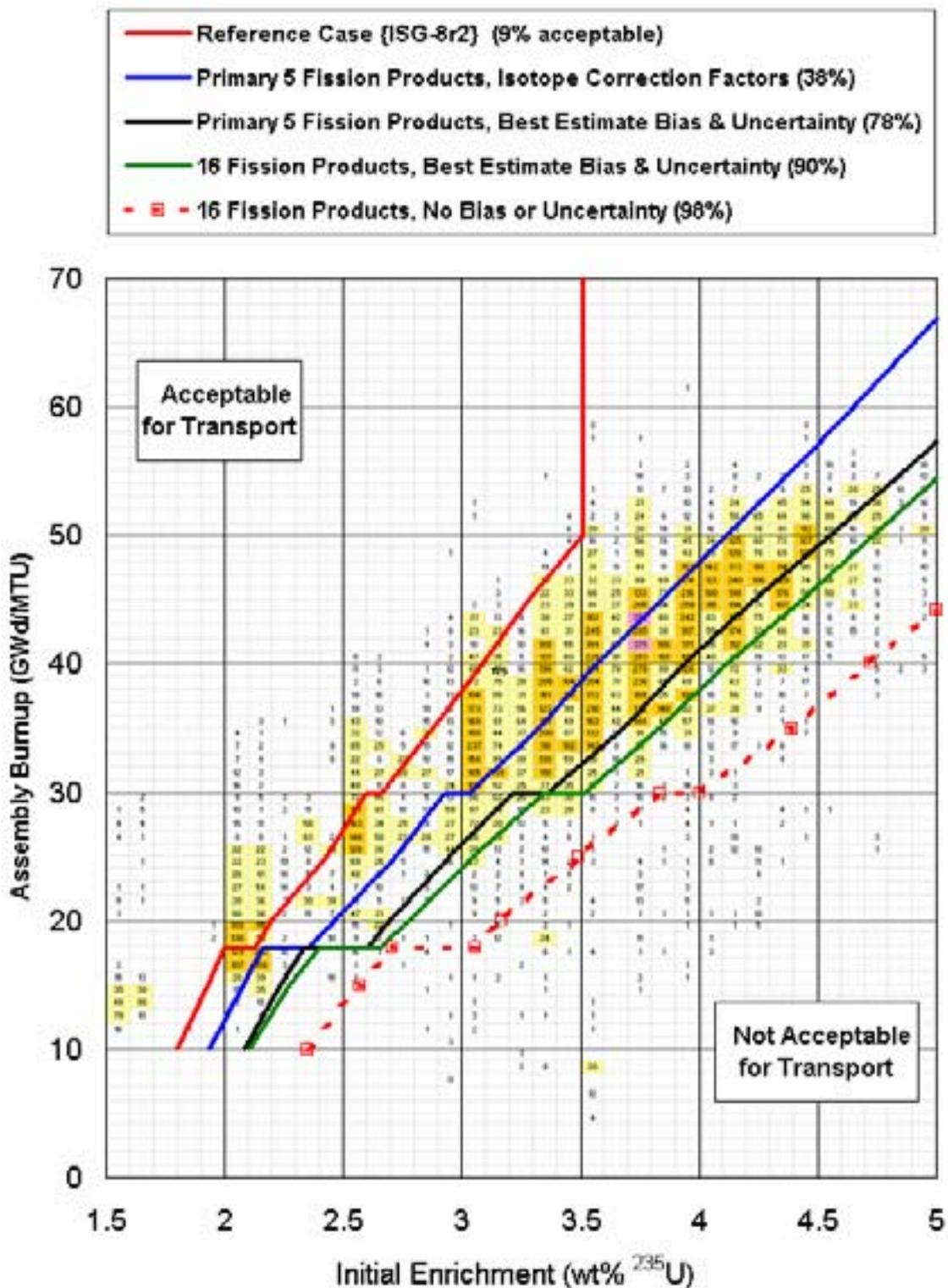
FIG. 4. Comparison of calculational assumptions for WE  $17 \times 17$  fuel assemblies. Percentages of inventory acceptable for the GBC-32 cask are shown in parentheses.
