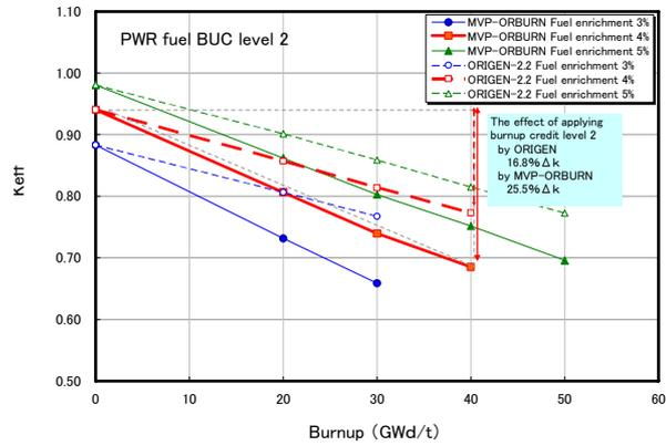
FIG. 11. Difference between the initial enrichment and the burnup credit level 2 calculations for PWR fuel.
