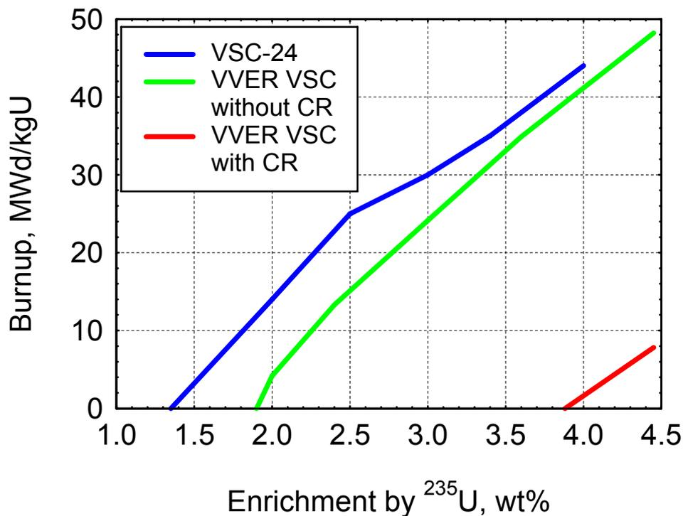
FIG. 3. Loading curve for VSC.
