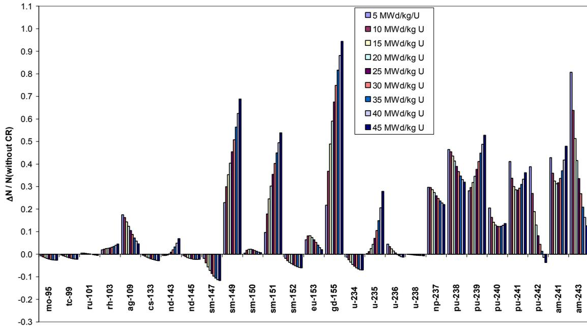
FIG. 7. Relative change of isotopic number densities due to CR insertion (Zero cooling time).
