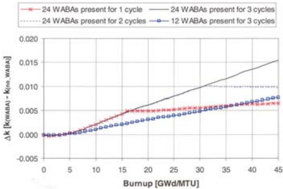
FIG. 3. Comparison of  $\Delta k$  values, as a function of burnup, for assemblies exposed to wet annular burnable assembly (WABA) rods. Results correspond to Westinghouse  $17 \times 17$  assemblies with 4.0 wt %  $^{235}\text{U}$  initial enrichment[11].
