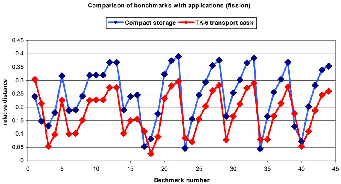
Fig. 4. Relative distance of homogeneous MOX benchmarks from applications for 5 group fission.
