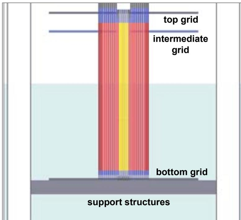
Fig. 3: Vertical cut of the REBUS PWR core.
