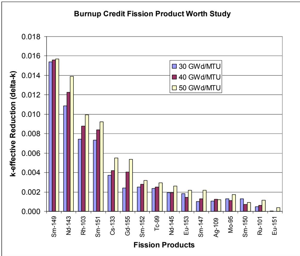
FIG. 5. Fission product worth calculated for WE  $17 \times 17$  SNF assemblies with 4 wt % initial enrichment and loaded in the GBC-32 after a 5-year cooling time.
