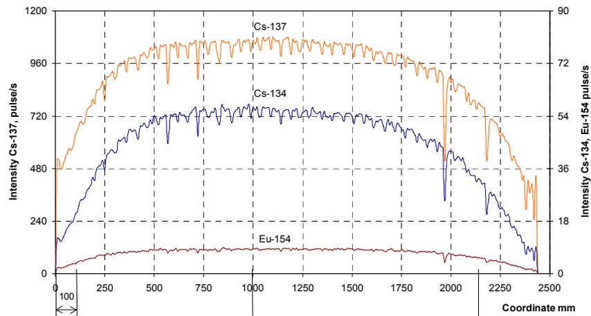
Fig. 1.5 Distribution of fission product throughout the height of fuel rod No. 69, FA No. 135 (Internal collimator– 3 mm, outer one – 5 mm, pitch – 10 mm).
