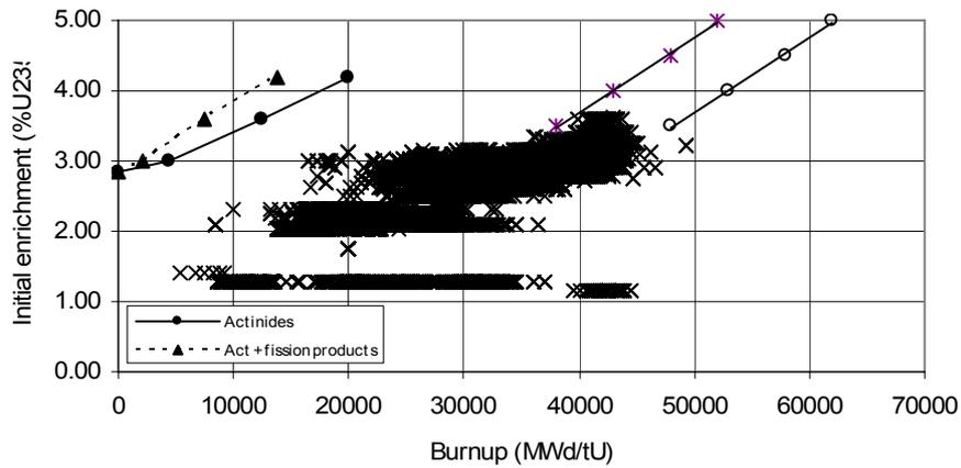
FIG. 3. Limit curves for BUC in final storage canister compared to 17512 BWR assemblies.
