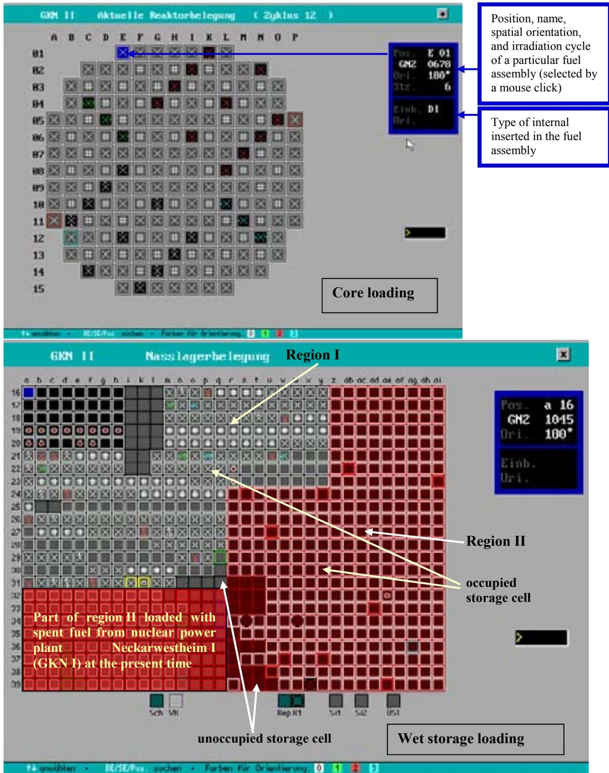
FIG. 5. Examples for the identification and documentation of the locations of fuel assemblies and internals within the nuclear power plant Neckarwestheim II (GKN II) with the aid of the code system ALFA.
