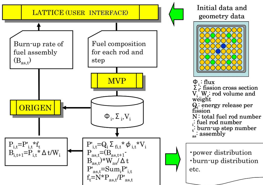
FIG.1. Calculation flow of MVP-ORBURN.
