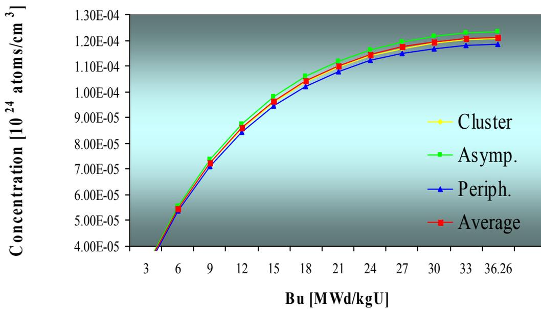
FIG. 6. Concentration of  $^{239}\text{Pu}$ , WWER-1000 spent fuel assembly.
