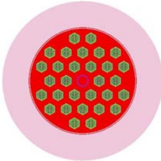
*FIG. 7. WWER-440 spent fuel cask with 30 assemblies. Visualization by KENO VI (x-y plane).*
