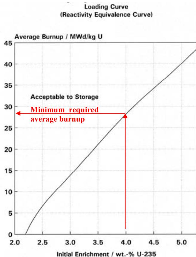
FIG. 6. Example for a loading curve. A loading curve indicates the minimum average burnup necessary for a fuel assembly with a specific initial enrichment to be loaded in the spent fuel management system of interest.
