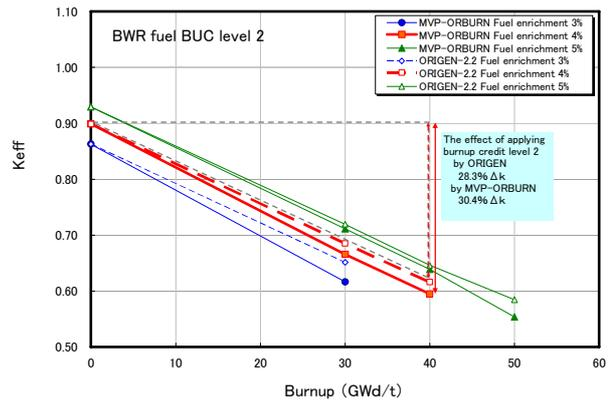
FIG. 13. Differences between the initial enrichment and the burnup credit level 2 calculation for BWR fuel.
