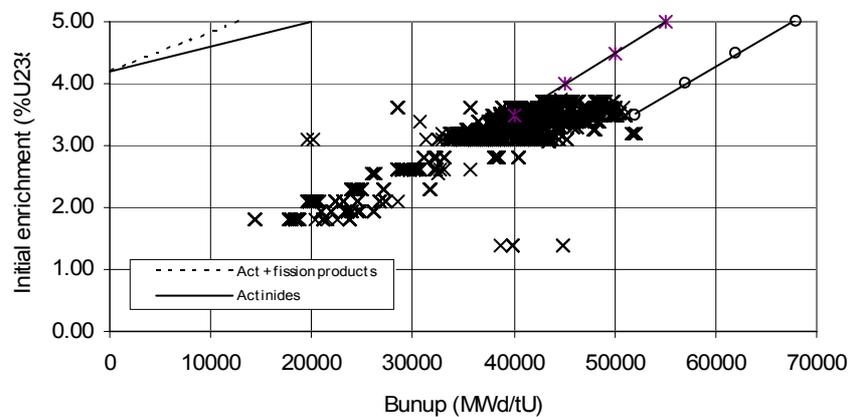
FIG.2. Limit curves for BUC in CLAB compared to 2021 PWR assemblies.
