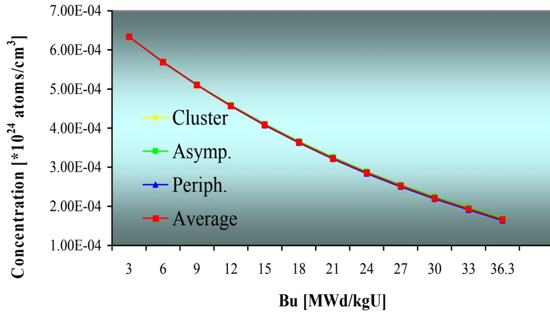
FIG. 5. Concentration of  $^{235}\text{U}$ , WWER -1000 spent fuel assembly.
