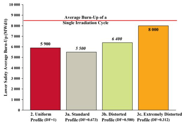
FIG. 6. Lower safety average burnup of fuel assemblies for calculation sequence 3.
