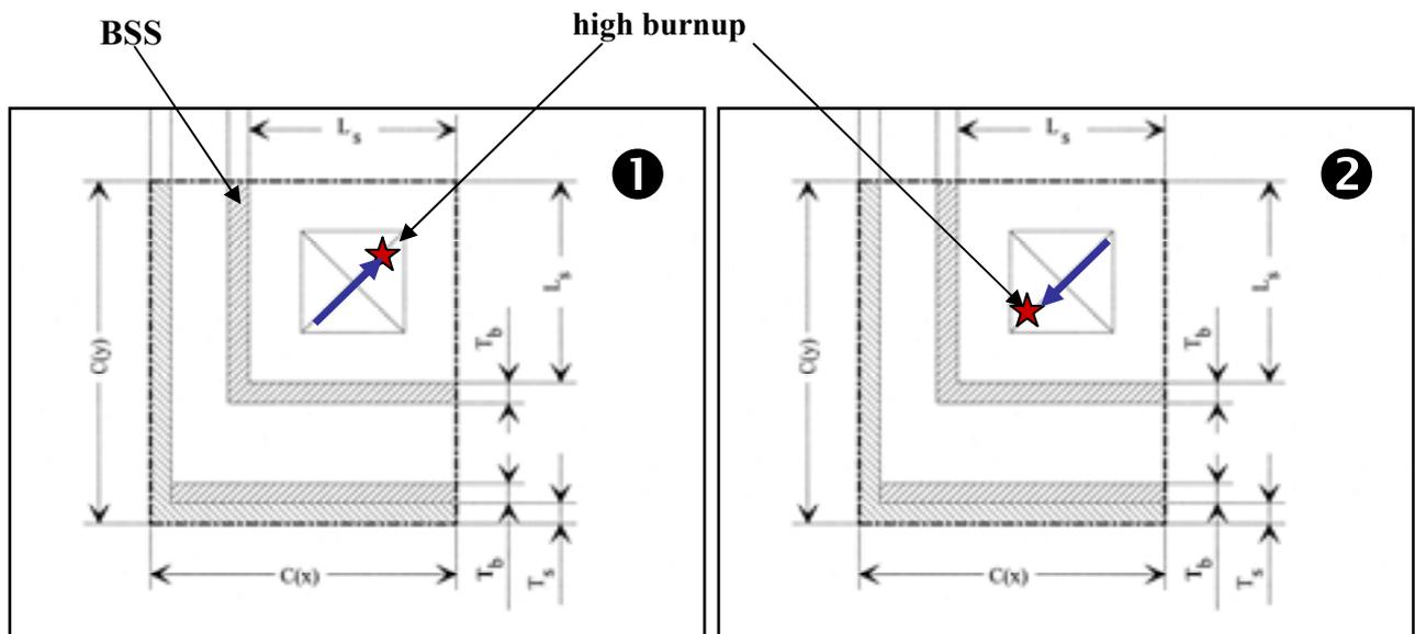
FIG. 28. Storage cell with non-isotropic arrangement of neutron absorbing panels.
