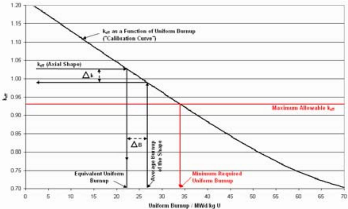
FIG. 2. The end effect  $\Delta k$  is the difference between the spent nuclear fuel system's neutron multiplication factor obtained with an axial burnup profile (axial shape) and the neutron multiplication factor obtained for the system by assuming the average burnup of the profile uniformly distributed over the active zone of the spent fuel.
