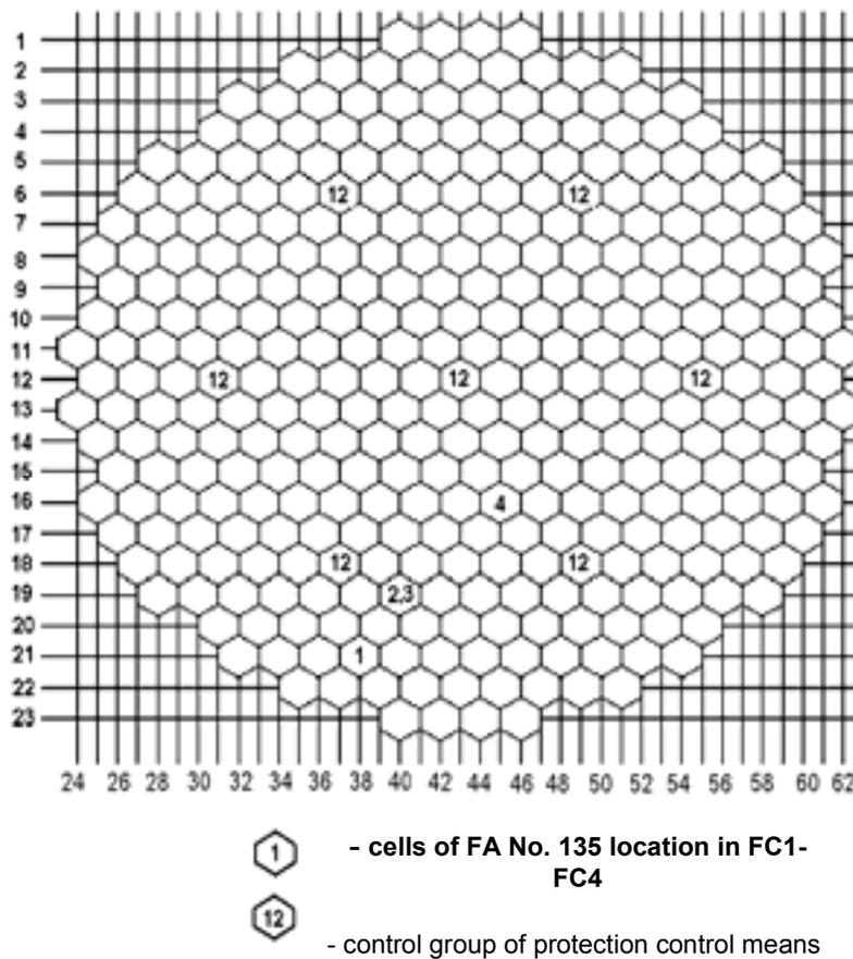
Fig. 1.2 Location of FA No. 135 in the core of the 4<sup>th</sup> power unit Novovoronezh NPP.
