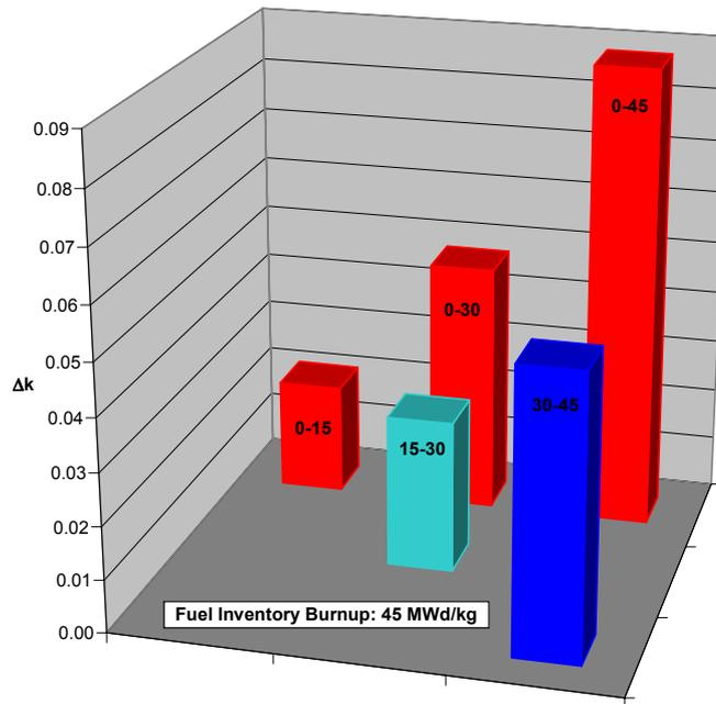
FIG. 5. Example for the Increase  $\Delta k$  in the neutron multiplication factor due to the use of fixed neutron absorbers.
