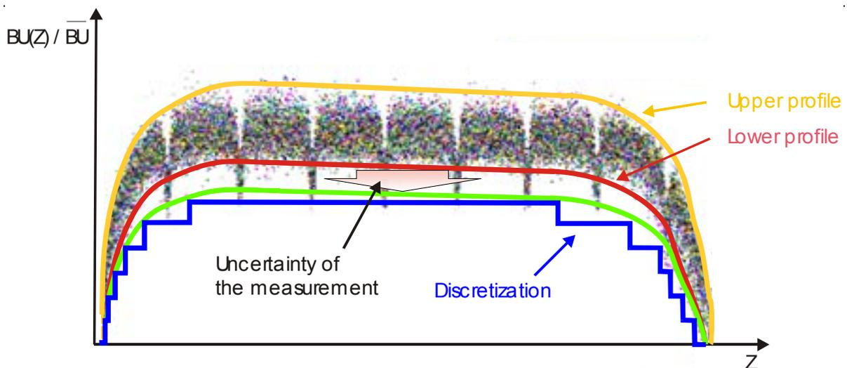
FIG. 1. Example of a conservative axial profile determination.
