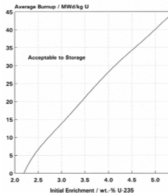
FIG. 1. Example for a loading curve of a spent fuel management system.
