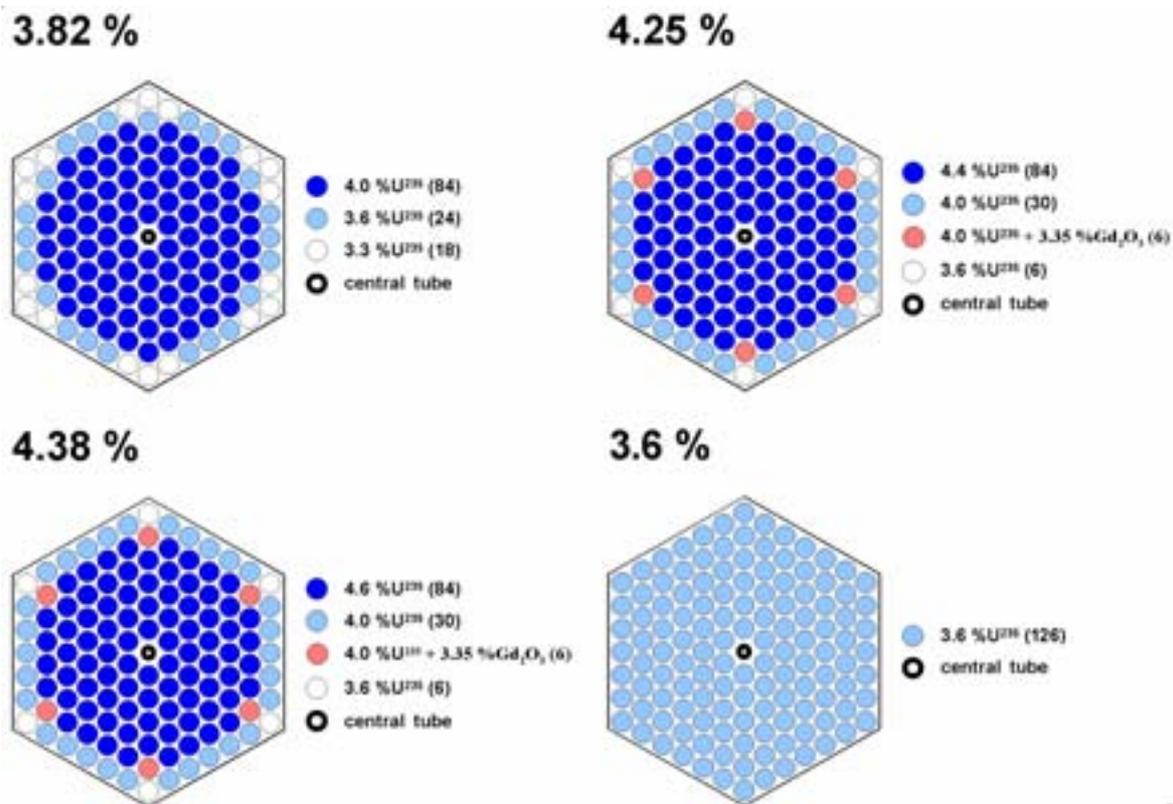
FIG. 1. Working FAs of horizontally uniform or profiled enrichment (3.6 wt. % or average 3.82/4.25/4.38 wt.%, respectively) used in Dukovany NPP.
