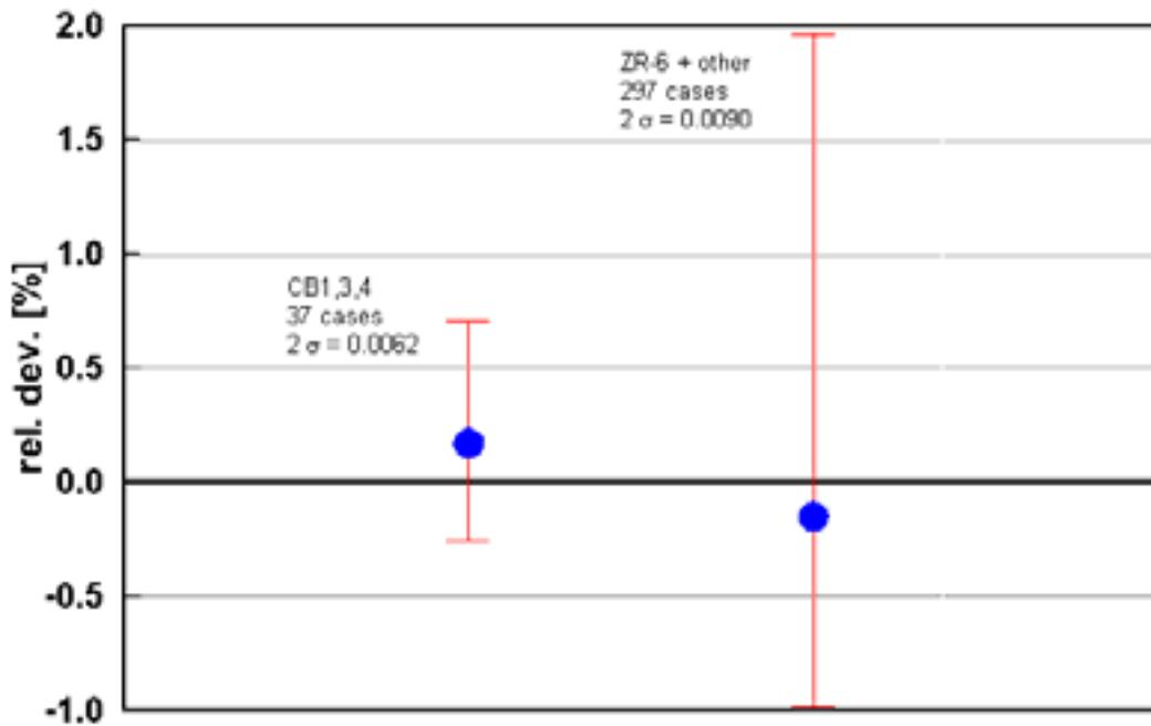
Fig.1.3 Kef deviation for KENO VI (minimal, average and maximal).
