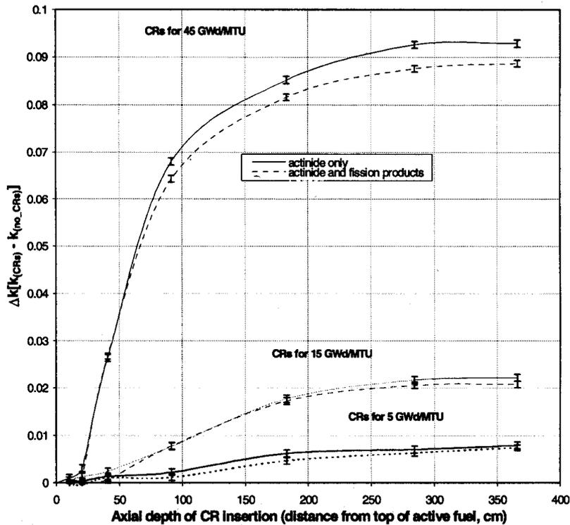
FIG. 4. Impact of CR insertion during irradiation on SNF in the GBC-32 cask [13].
