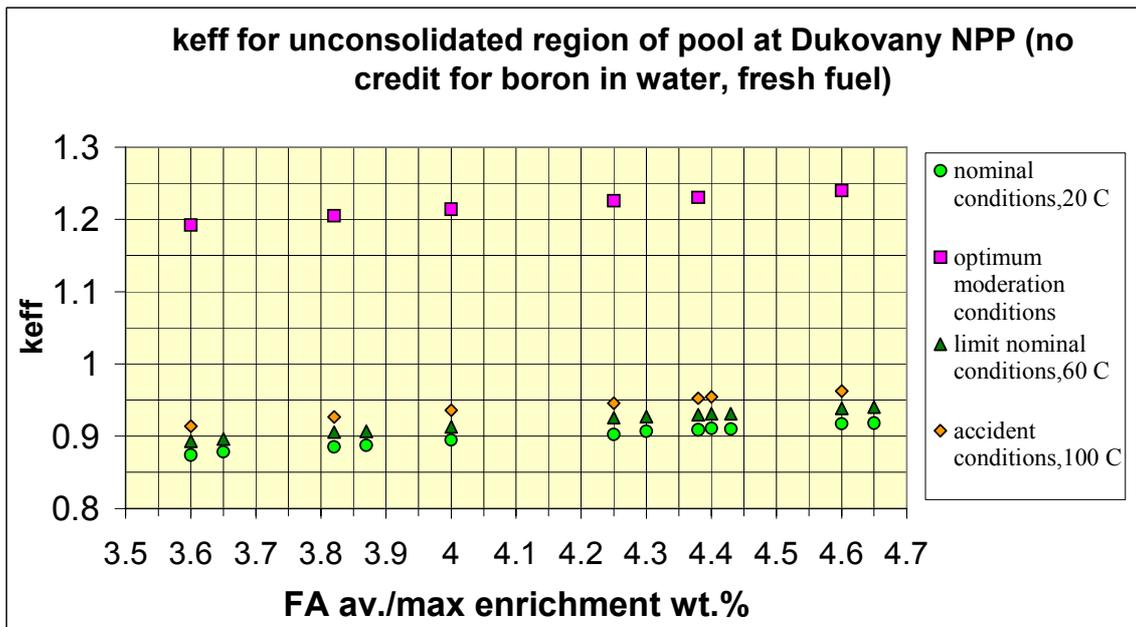
FIG. 5. Criticality calculations for upper non-reracked region of pool at Dukovany NPP (no credit for boron in water, fresh fuel).
