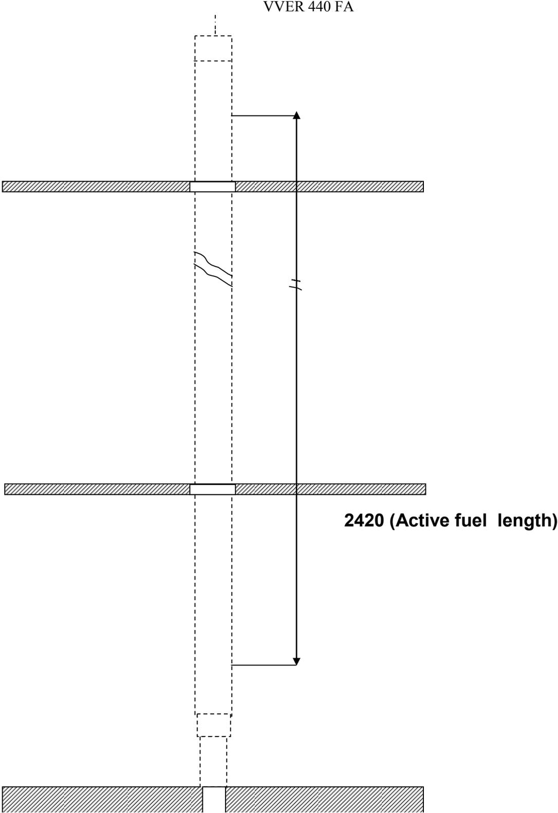
FIG. 2. Vertical section through storage rack.
