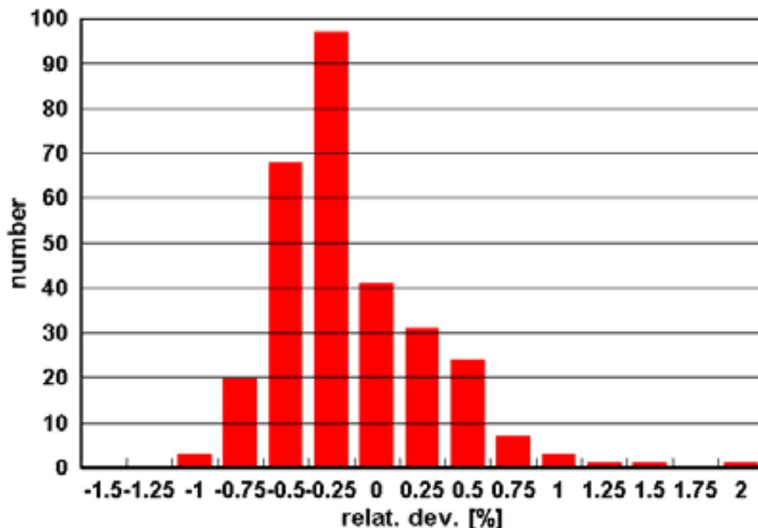
Fig.1.1 Histogram of  $K_{ef}$  deviation for KENO VI, 297 experiments.  $2\sigma = 0.0090$ .
