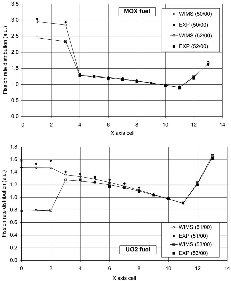
Figure 2. Comparison between the calculated and measured fission rate distributions.
