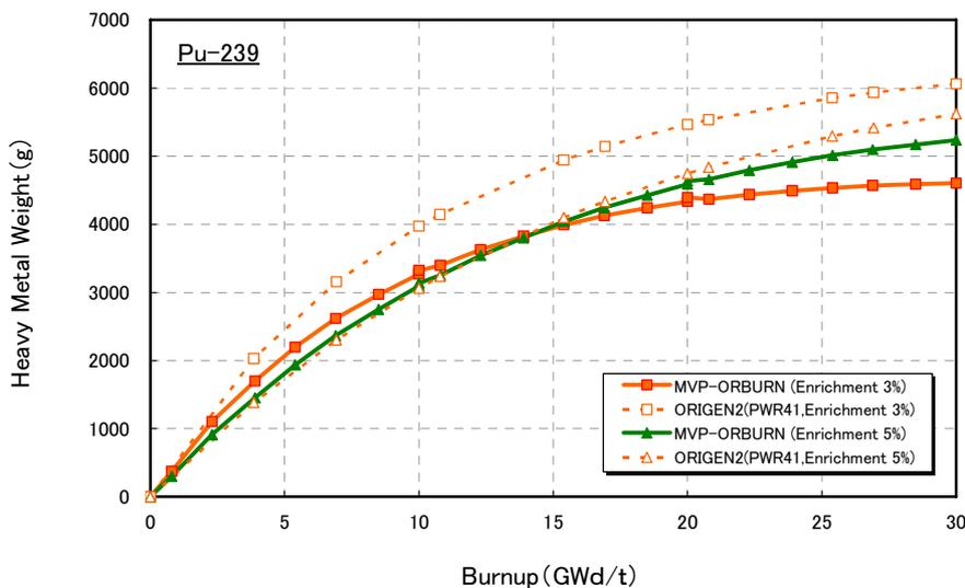
FIG.9 Comparison of MVP-ORBURN and ORIGEN (depletion characteristics for Pu-239).
