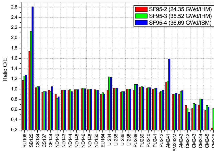
Fig. 4: Ratio of calculated (C) and measured (E) nuclide fractions for the SF95 sample series of spent fuel samples from Takahama-3 reactor.
