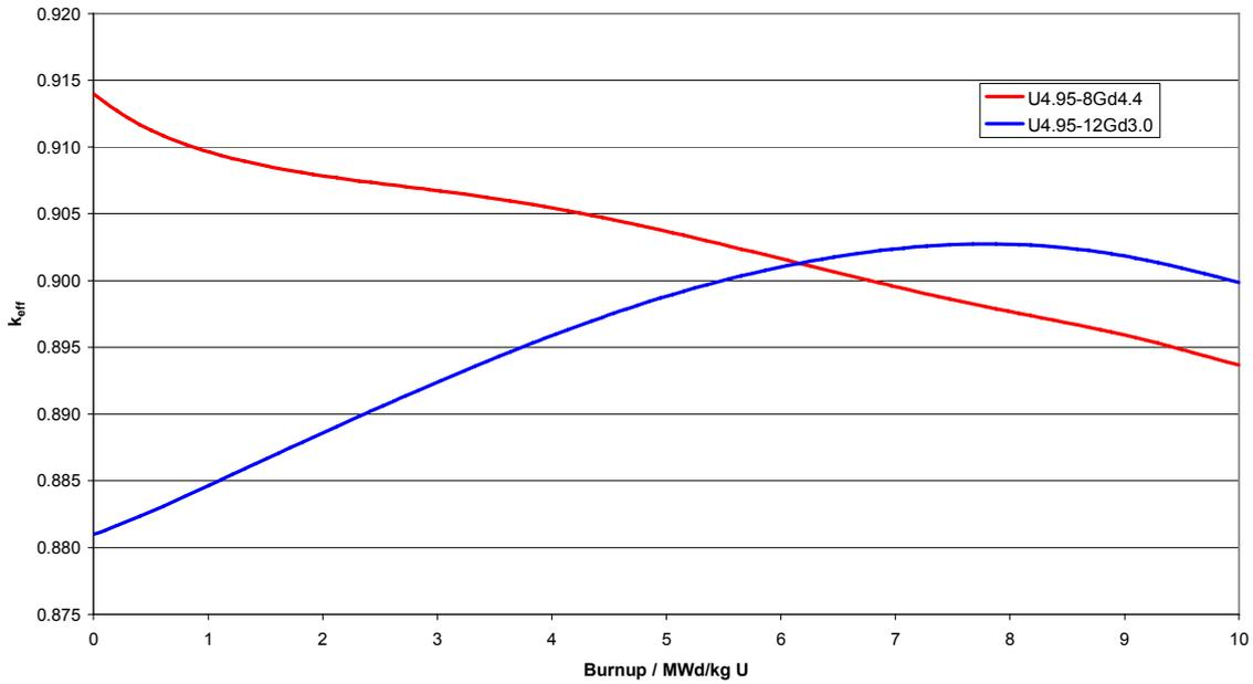
*FIG. 6. Examples for the reactivity impact due to the usage of integral burnable absorbers.*
