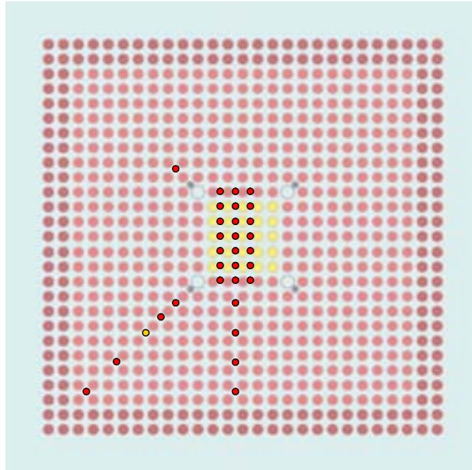
Fig. 4: Horizontal cut of the REBUS PWR core with Sc wire positions.
