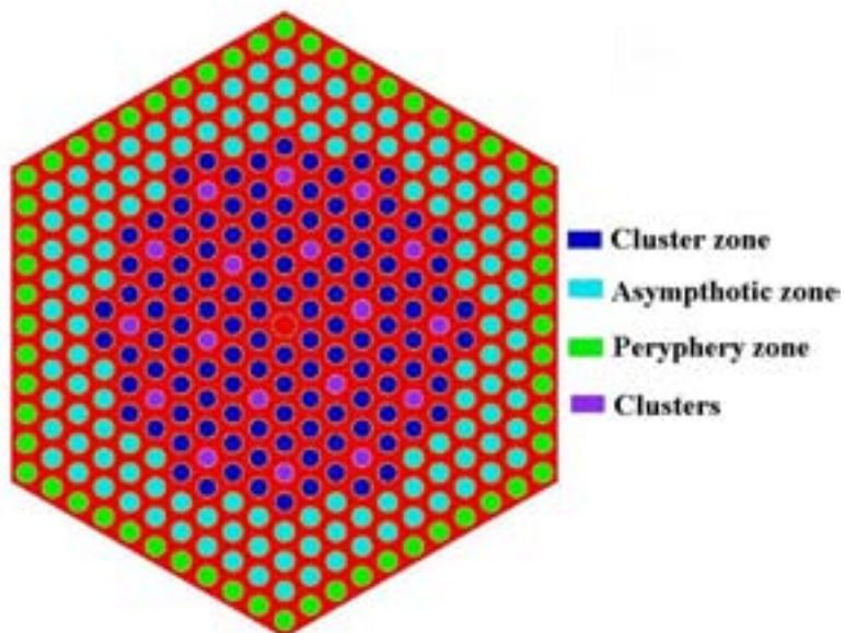
FIG. 2. WWER-1000 spent fuel assembly (x-y plane). Visualization by KENO VI.
