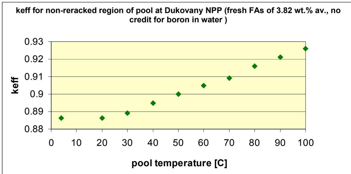
FIG. 4. Criticality calculations for upper non-racked region of pool at Dukovany NPP with FAs of 3.82 wt.% av. (no credit for boron in water, fresh fuel).
