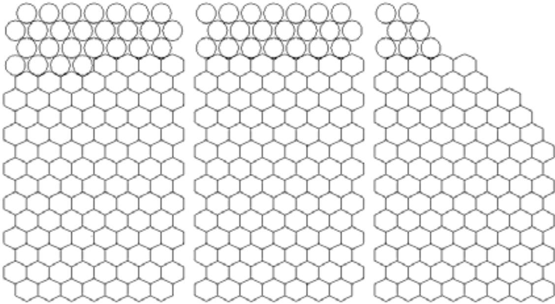
FIG. 3. Array of positions of FAs in non-racked region of pool at Dukovany NPP.
