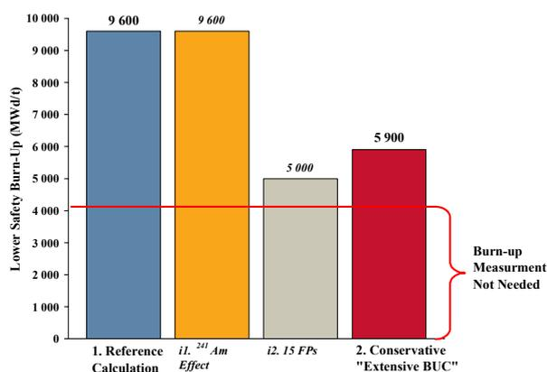
FIG. 3. Lower safety burnup of fuel assemblies for calculation sequences 1 and 2.
