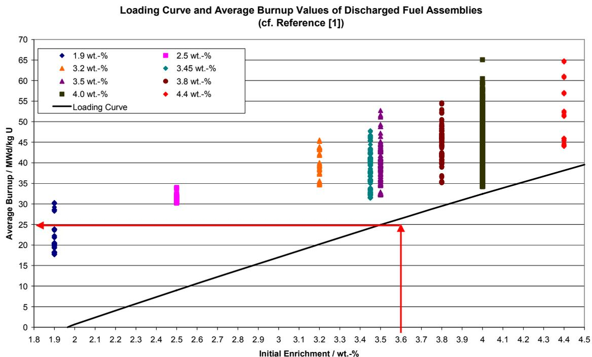
FIG. 1. Example for a Loading Curve (LC) and for average burnup values of spent fuel assemblies to be loaded in the spent fuel system for which the LC is determined.
