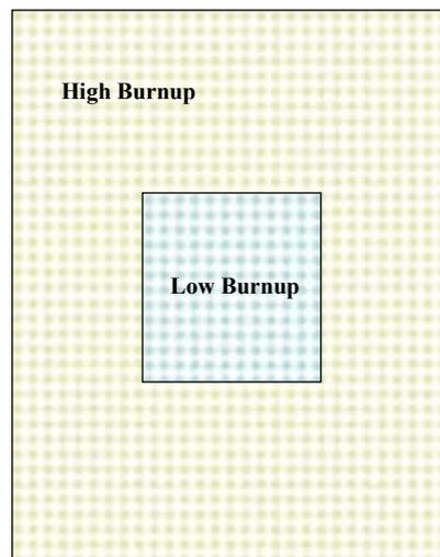
Fig. 2. Schematic of original 2-zone model for BWR fuel in dissolver (side view).
