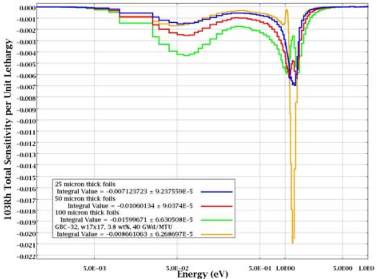
FIG. 7. GBC-32 and SNL experiment  $^{103}\text{Rh}$  sensitivity profiles.
