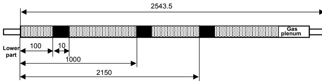
Fig. 1.4 Cutting procedure of specimens from fuel rods No. 69 in FA No. 135.
