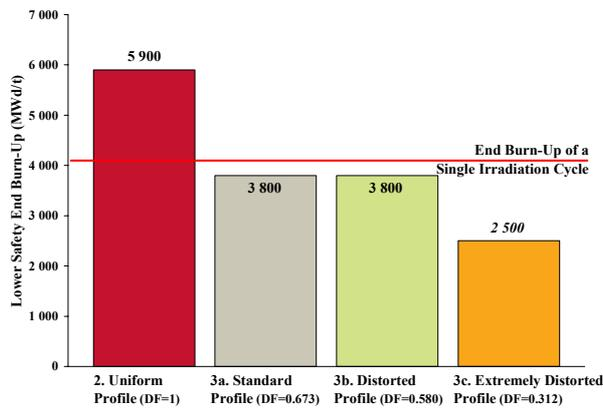
FIG. 4. Lower safety end burnup of fuel assemblies for calculation sequence 3.
