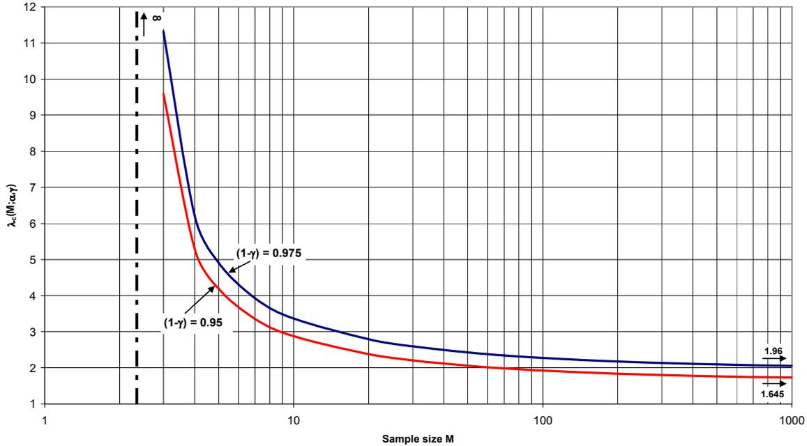
FIG. 3. Factor  $\lambda_c(M; \alpha, \gamma)$  for one-sided  $(1-\gamma)/(1-\alpha)$  tolerance limits with  $(1-\alpha) = 0.95$  (cf. equation (3.29)).
