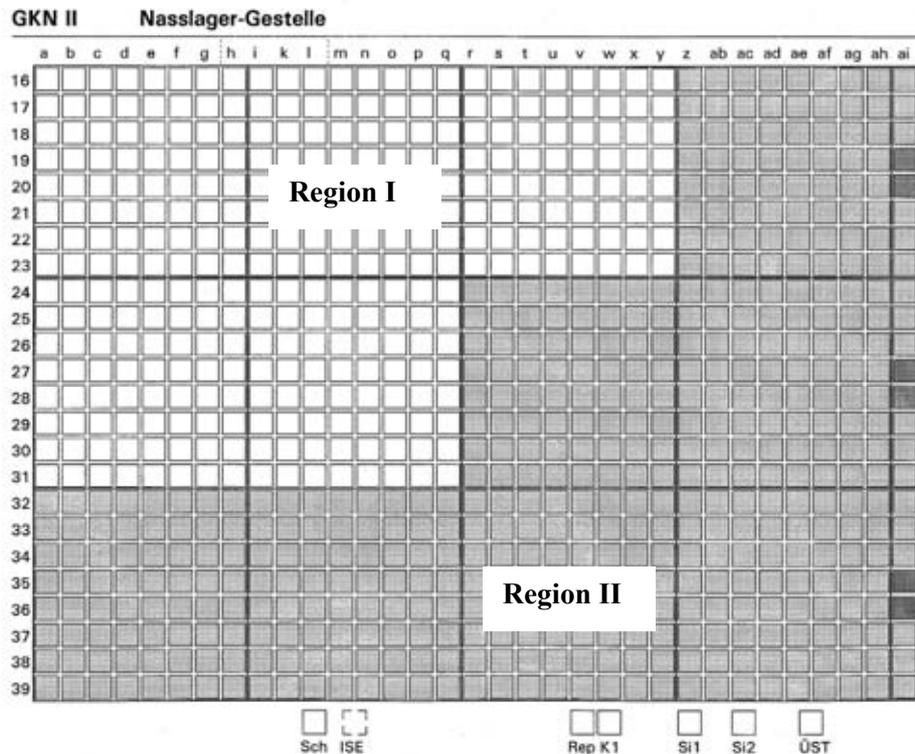
FIG. 2. Neckarwestheim wet storage pond: Application of burnup credit has made it necessary to divide the storage pool into two storage regions [1].
