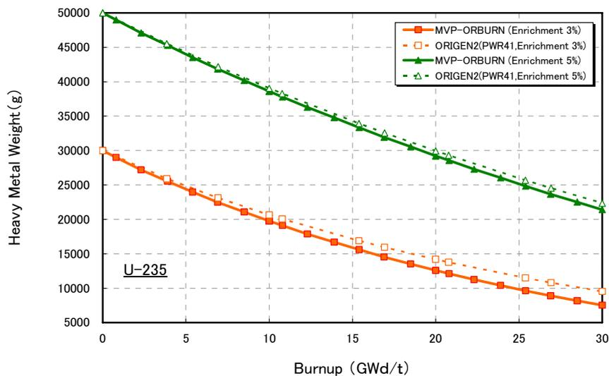
FIG. 8. Comparison of MVP-ORBURN and ORIGEN (depletion characteristics for U-235).
