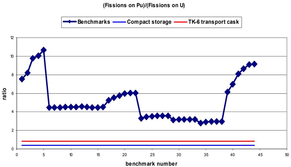
Fig. 7 Ratio of fissions happening on plutonium to the fission happening on uranium for homogeneous MOX benchmarks.
