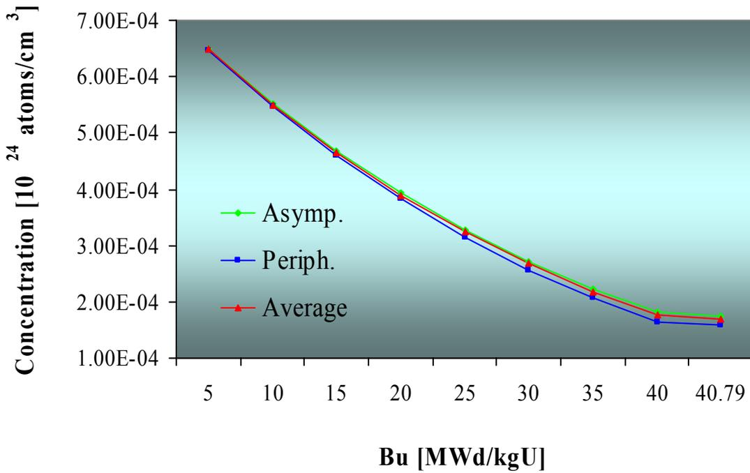
FIG. 3. Concentration of  $^{235}\text{U}$ , WWER-440 spent fuel assembly.
