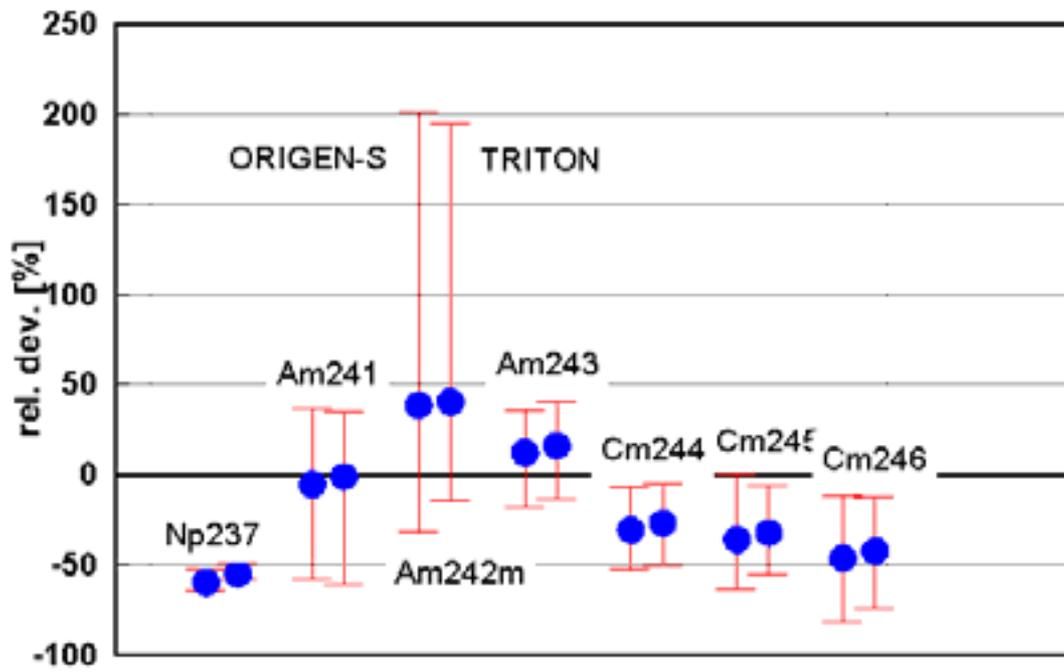
Fig.2.2a Deviation of nuclide concentration, experiment Novovoronezh 2 (8 samples).
