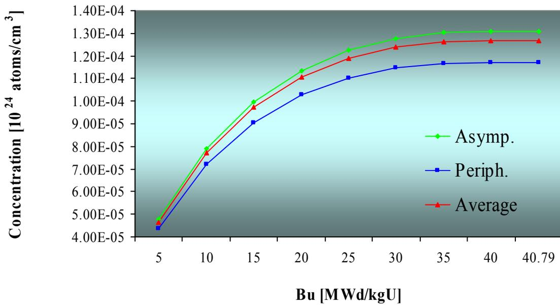
FIG. 4. Concentration of  $^{239}\text{Pu}$ , WWER-440 spent fuel assembly.
