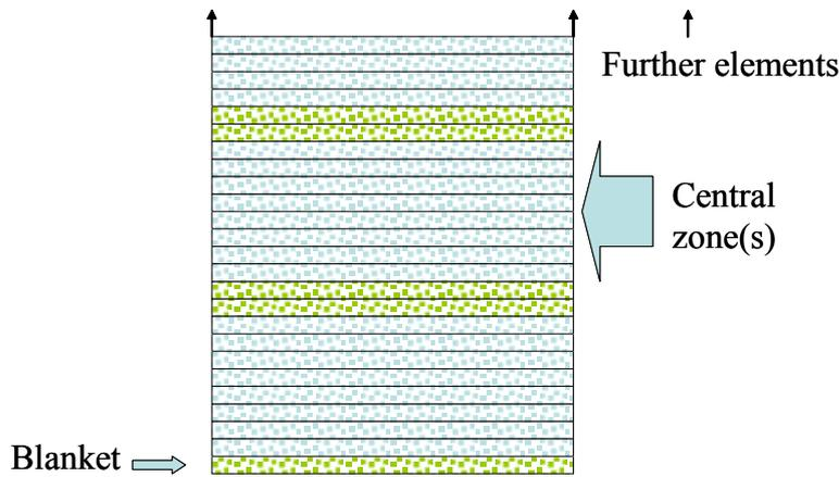
Fig. 4. Schematic of Refined Model for BWR Fuel in Dissolver (side view).
