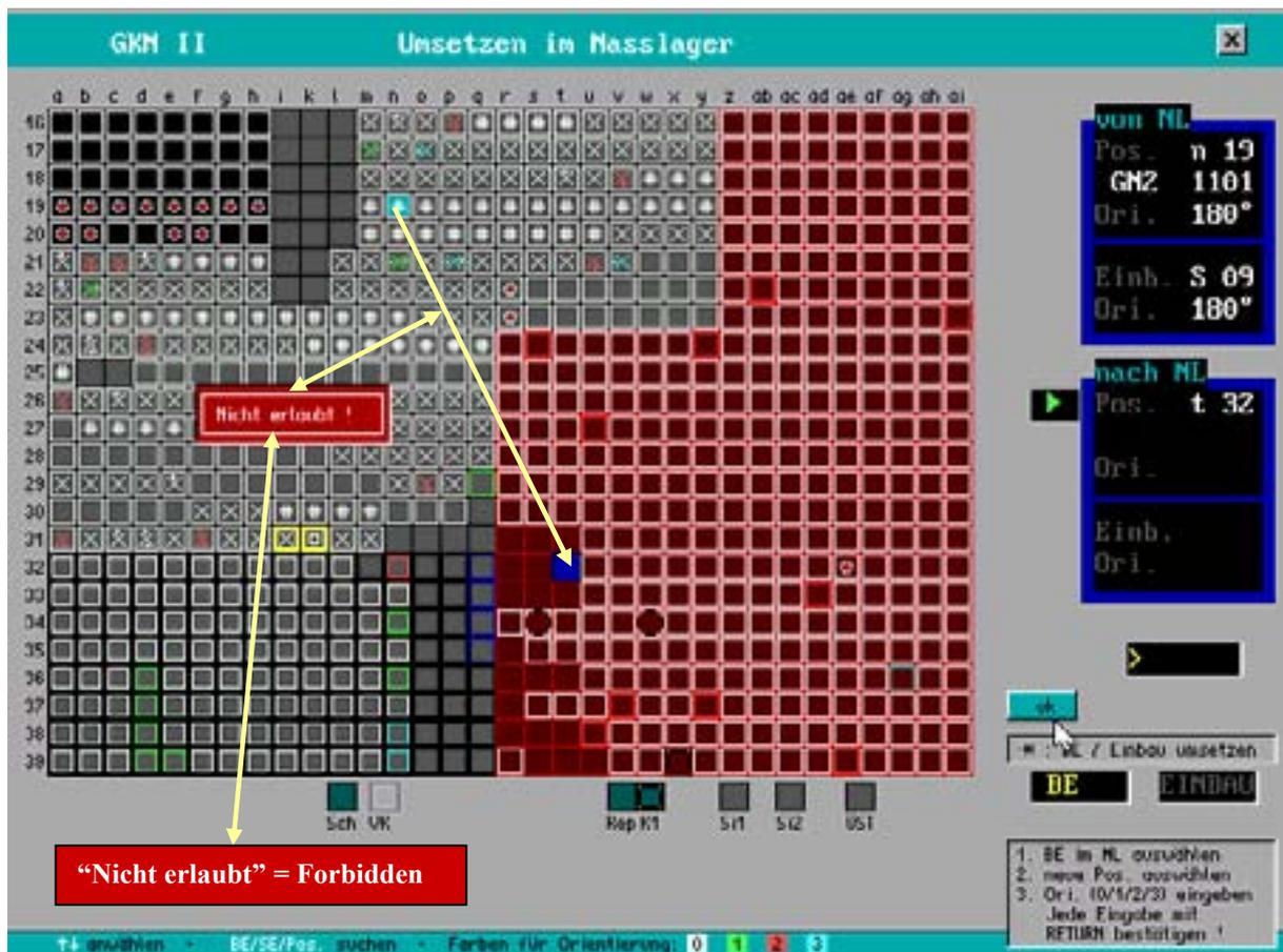
FIG 6. Example for the interlock logic schemes applied by ALFA to the planning of fuel handling operations.
