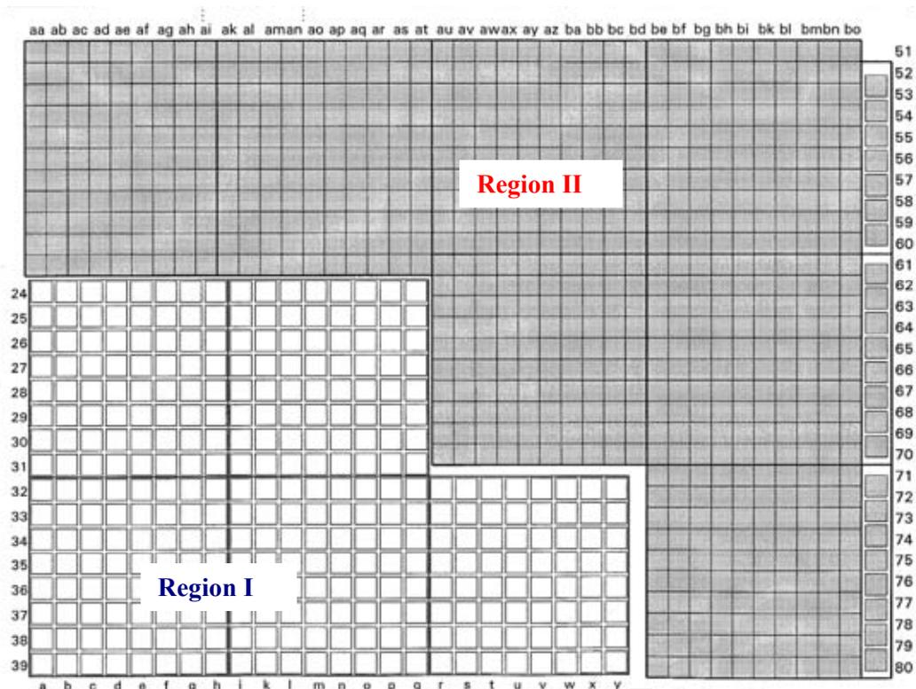
FIG. 7. Application of burnup credit to wet storage facilities results in dividing the storage pool into two regions at least [1][10].
