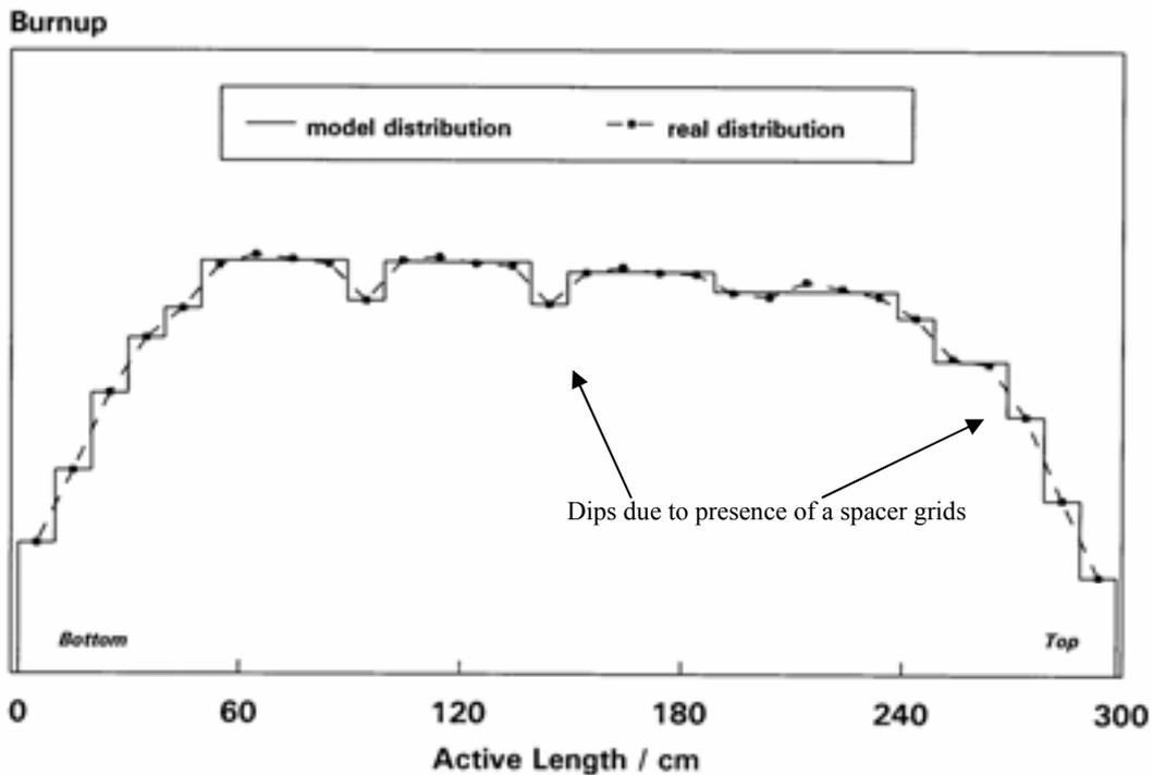
FIG. 1. Comparison of a burnup model distribution (step function) as usually used in burnup criticality calculations to an actual end-of-cycle axial burnup profile received from the German nuclear power plant Neckarwestheim I.
