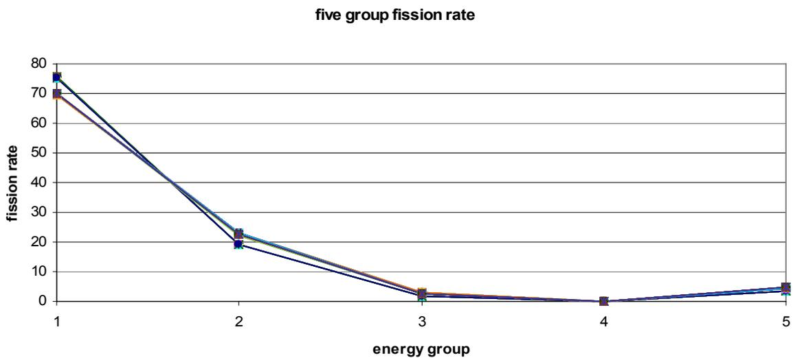
Fig. 9. Five group fission rates calculated for the MOX benchmark experiments with central absorber rod. In fact 88 curves are shown on this figure.
