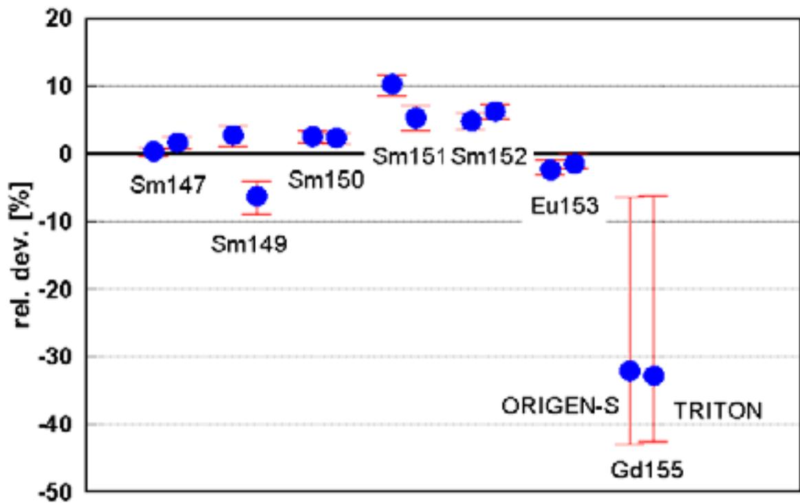
Fig.2.4b Deviation of nuclide concentration, numerical benchmark CB2 (6 samples).
