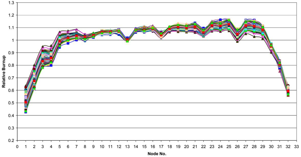
FIG. 3. Examples for axial burnup profiles obtained for fuel assemblies with 4.0 wt.-% initial enrichment.
