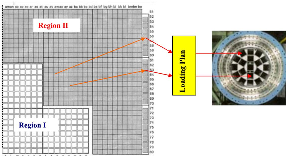
FIG. 8. A loading plan makes up a definite assignment of a storage position of the storage pit where a fuel assembly is coming from to the location inside a cask where the fuel is destined for. The first step in loading a cask is the transfer of the fuel to special positions in the pit each assigned to a particular location in the cask.
