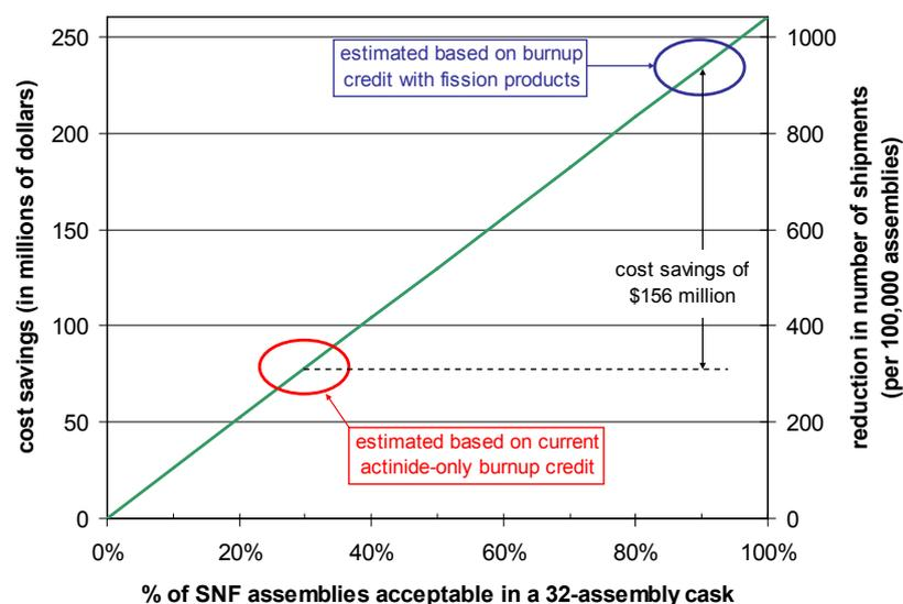
FIG. 6. Graphical representation of the potential cost savings associated with the use of 32-assembly casks, as opposed to the use of 24-assembly casks, assuming a cost of US \$250K per cask shipment. (Note that the cost savings scale linearly with the cost per shipment.)
