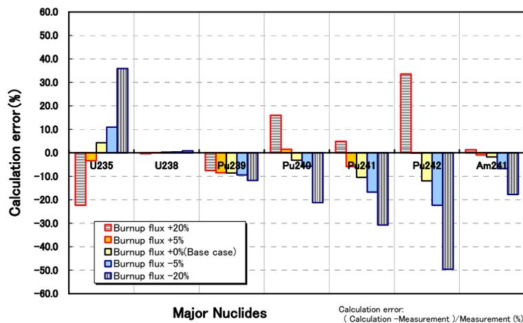
FIG.2. Influence of depletion flux level (PWR Fuel SF95-4).
