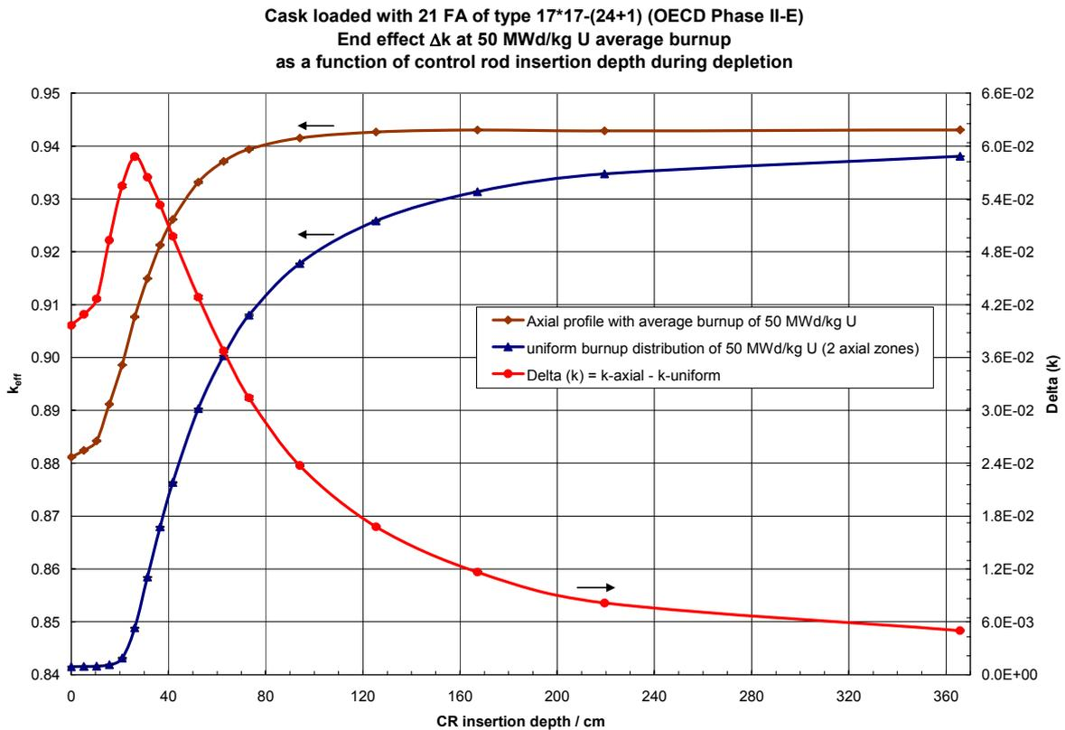
FIG 19. Cask loaded with 21 FA of type 17\*17-(24+1)(OECD Phase II-E) end effect  $\Delta k$  at 50 MW d/kg U average burnup as a function of control rod insertion depth during depletion.
