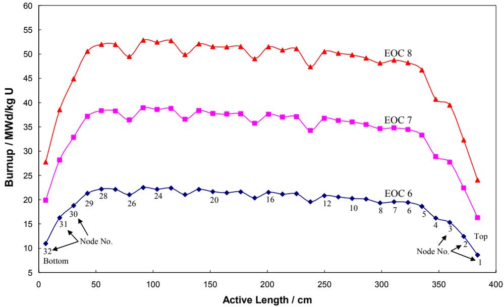
*FIG. 1. Typical PWR axial burnup profiles.*
