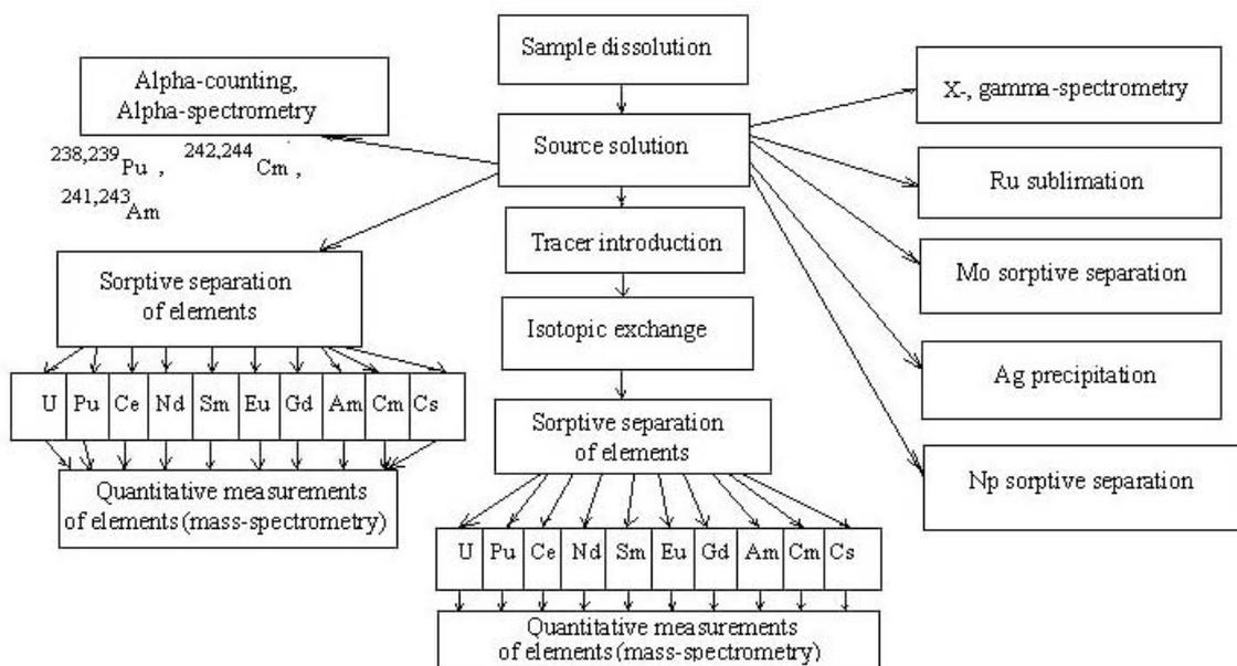
Fig. 1.6 General scheme of irradiated fuel analysis.
