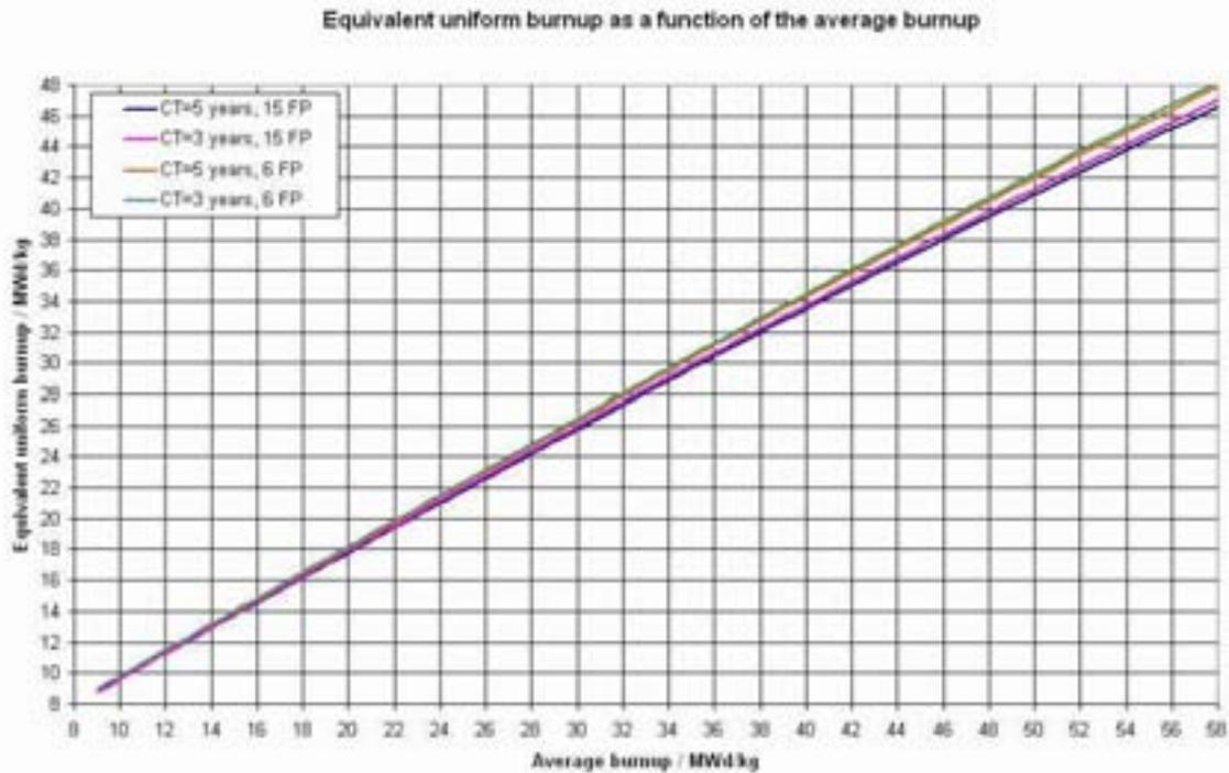
FIG. 4. Examples for cooling time effects on the end effect for different numbers of fission products included in the criticality calculation (CT:= cooling time, FP:= fission product).
