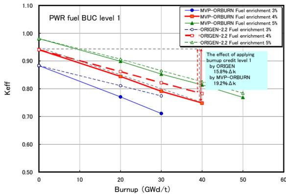
FIG. 10. Difference between the initial enrichment and the burnup credit level 1 calculations for PWR fuel.
