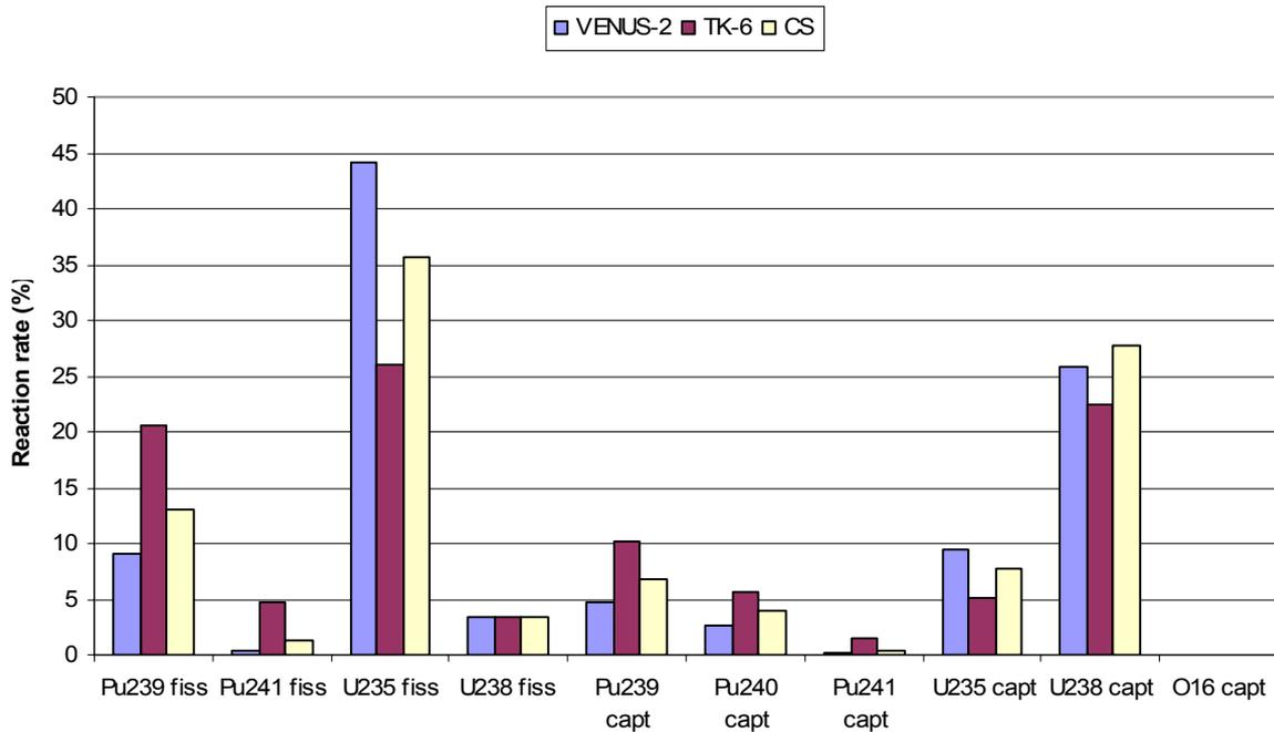
Fig.10. Comparison of reaction rate balance of compact storage pool and TK-6 cask with burnup credit and of VENUS-2 benchmark.
