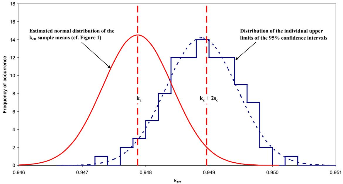
FIG. 2. Comparison of the distribution of the individual upper limits of the 95% confidence intervals given in Table 1 with the  $k_o + 2s_o$  value of the distribution of the  $k_{eff}$  sample means.
