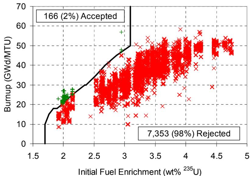
FIG. 2. B&W  $15 \times 15$  inventory shown with ISG-8 burnup credit limit curve.
