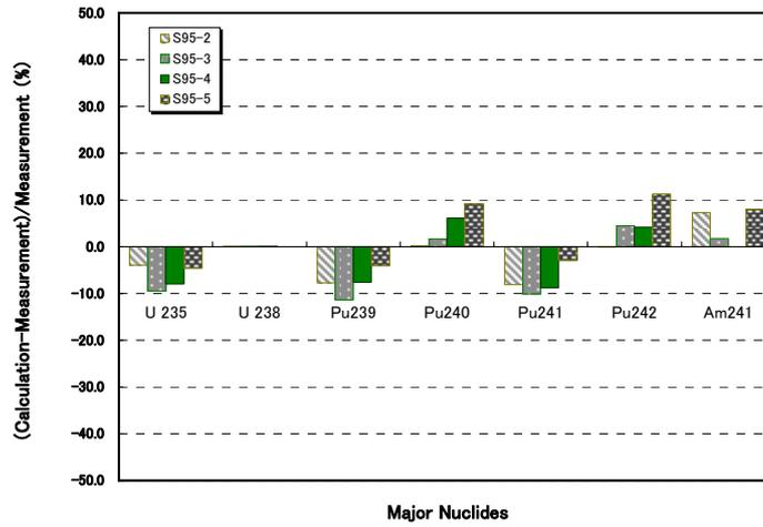
FIG. 5. Benchmark calculation results by MVP-ORBURN for JAERI PIE data (PWR spent fuel: SF-95).
