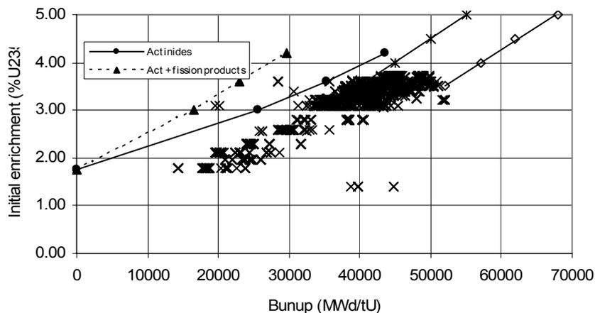
FIG. 4. Limit curves for BUC in final storage canister compared to 2021 PWR assemblies.
