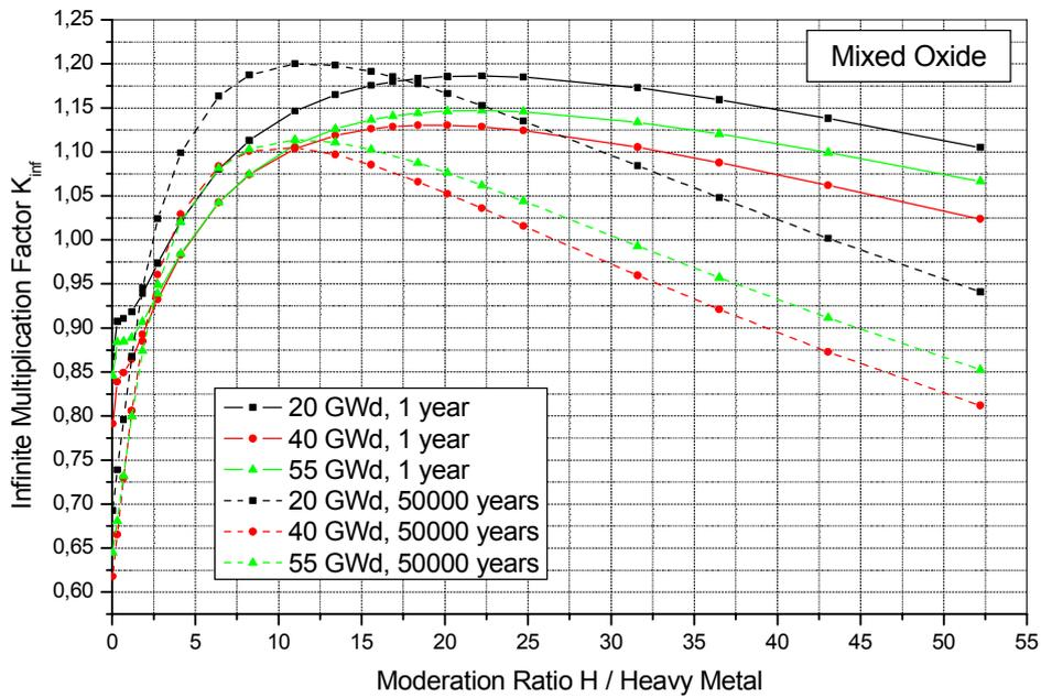
Fig. 3: Calculated  $k_{inf}$  of homogeneous spent MOX fuel-water-mixtures for various values of burnup and cooling time.
