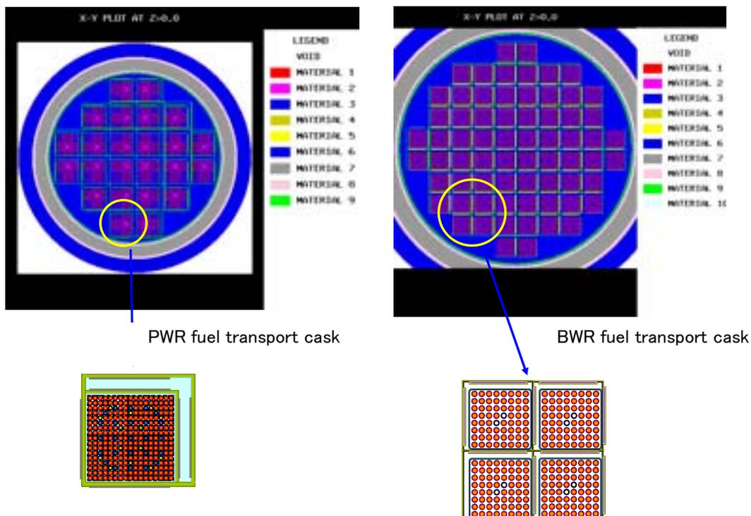
FIG. 7. Cross sectional view of criticality calculation model of transport cask for PWR and BWR fuels.
