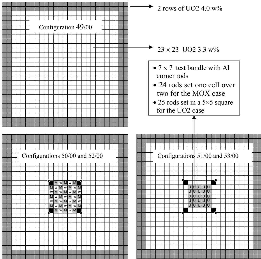
Figure 1. XY view of the critical configurations achieved in VENUS, in the frame of REBUS-PWR
