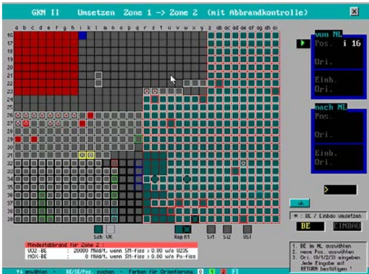
FIG. 7. Example for the interlock logic schemes applied by ALFA to the planning of fuel handling operations.
