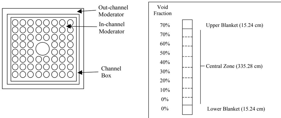
Fig. 3. Schematic of nominal BWR fuel element based on OECD-NEA BUC Phase III benchmark.
