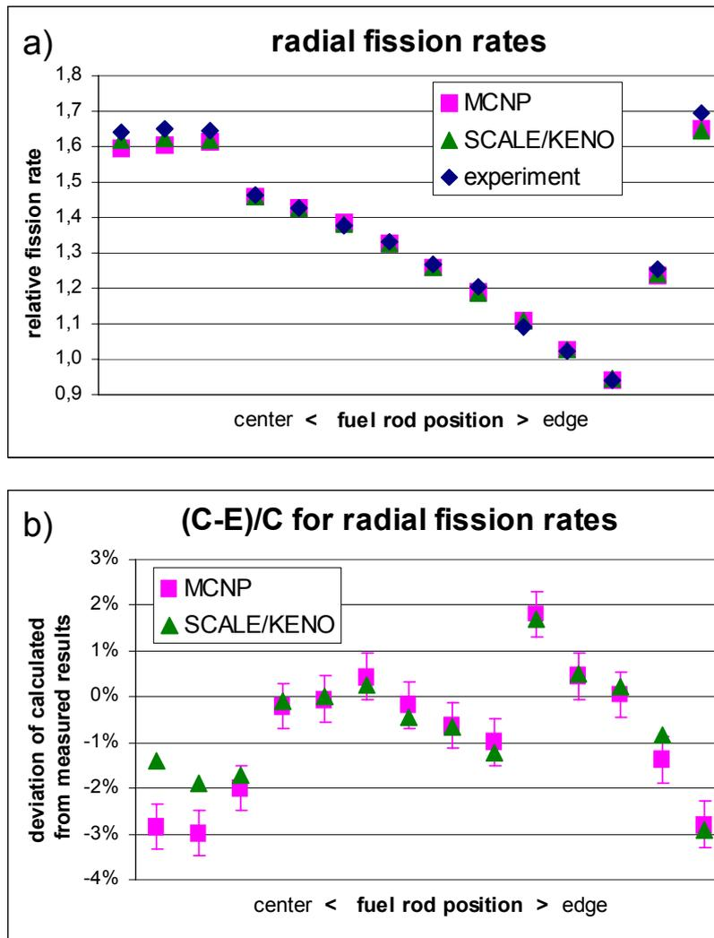
Fig. 5: Fission rates along the  $x=0$  axis: a) relative fission rates, b) comparison between measured and calculated values.
