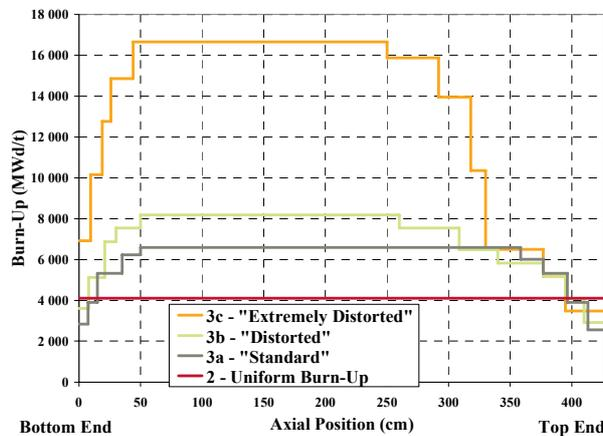
FIG. 5. Comparison of the three studied axial profiles normalized to an end burnup equal to 4 100 MWd/t.
