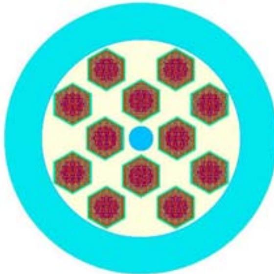
*FIG. 8. WWER-1000 spent fuel cask with 12 assemblies. Visualization by KENO VI (x-y plane).*
