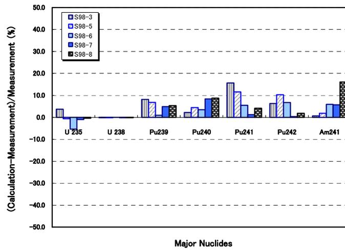
FIG. 6. Benchmark calculation results by MVP-ORBURN for JAERI PIE data (BWR spent fuel: SF-98)
