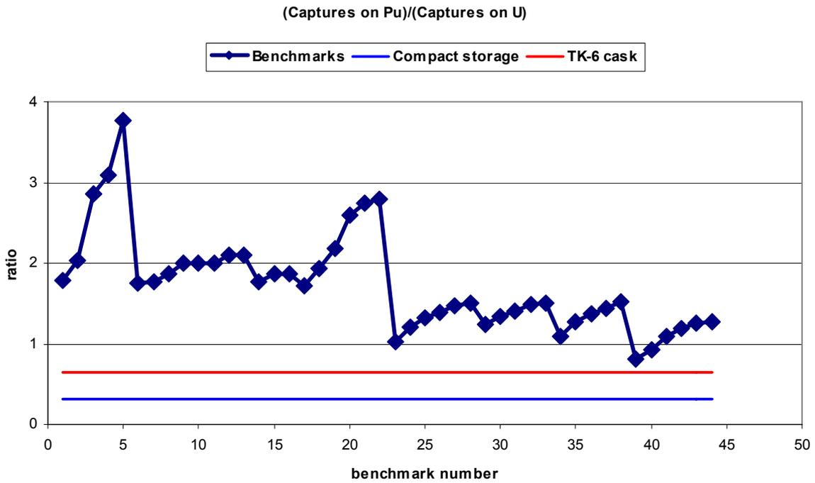
Fig. 8. Ratio of captures happening on plutonium to the fission happening on uranium homogeneous MOX benchmarks.
