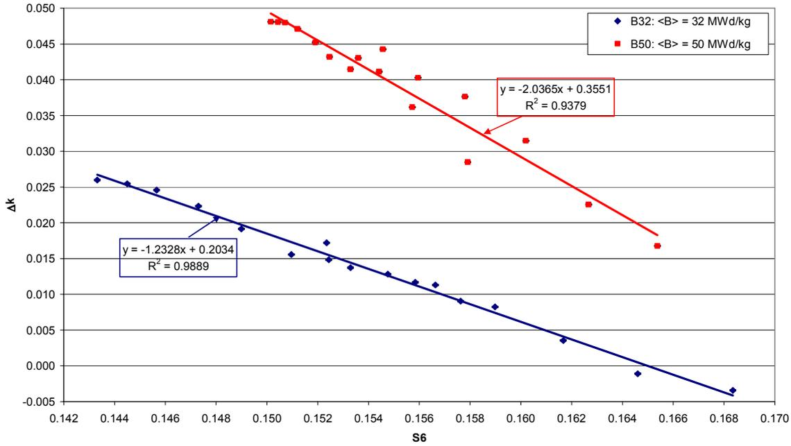
FIG. 17. End effect  $\Delta k$  as a function of the top end parameter  $S_6$  [4].
