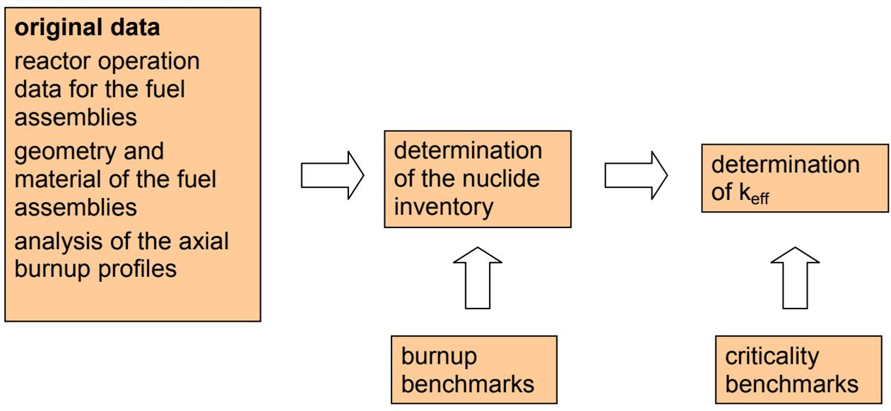
Fig. 2 Methodology for applying BUC in criticality analysis for PWR spent fuel casks.
