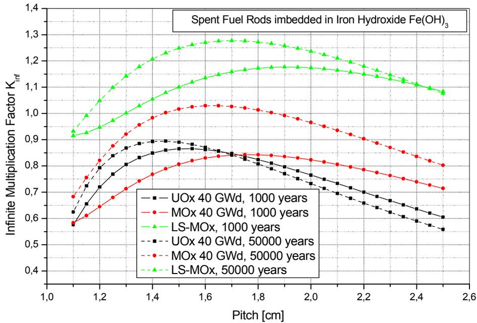
Fig. 4: Calculated  $k_{inf}$  for spent fuel rod lattice filled with Iron Hydroxide for various values of burnup and cooling time.
