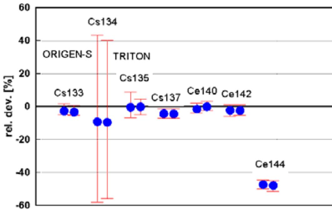
Fig.2.2b Deviation of nuclide concentration, experiment Novovoronezh 2 (8 samples).
