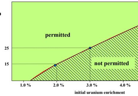
Fig. 3 Standard procedure – loading curve.
