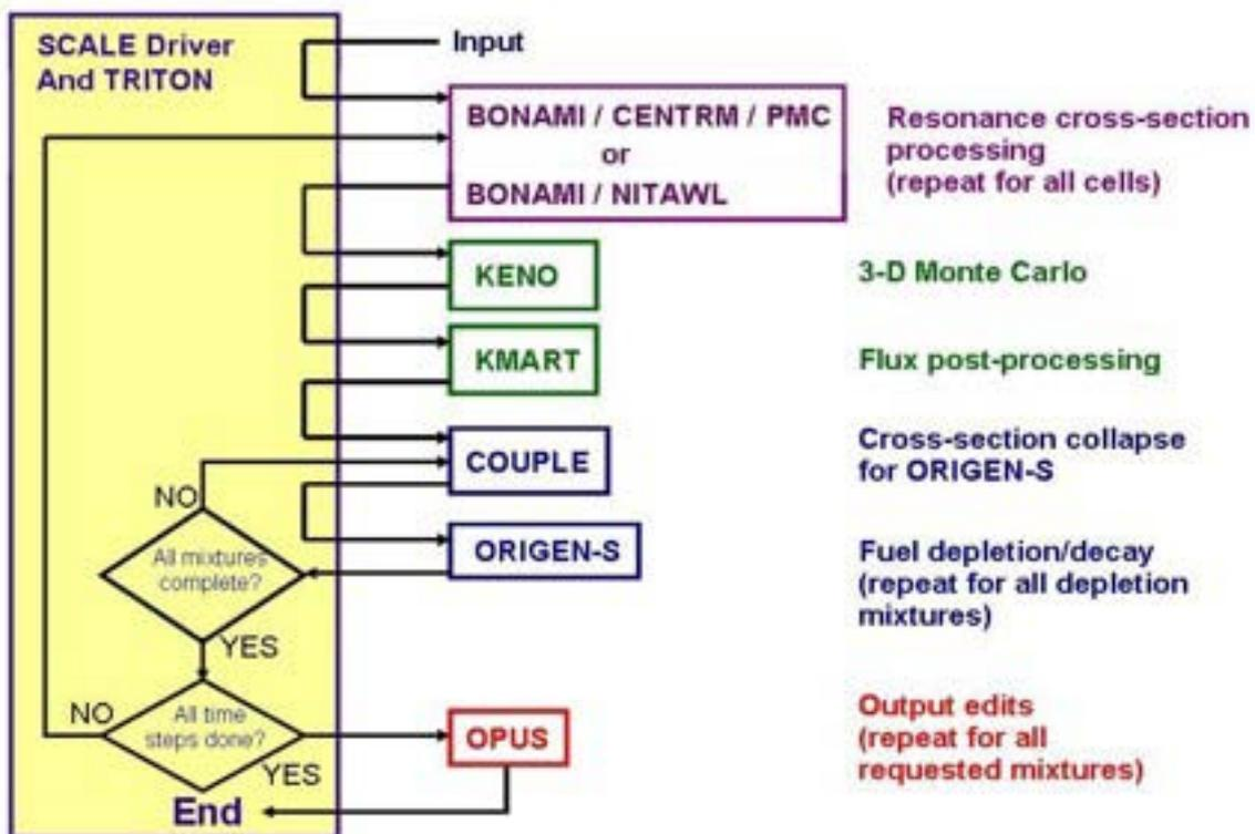
FIG. 2. TRITON sequence for KENO-based depletion.
