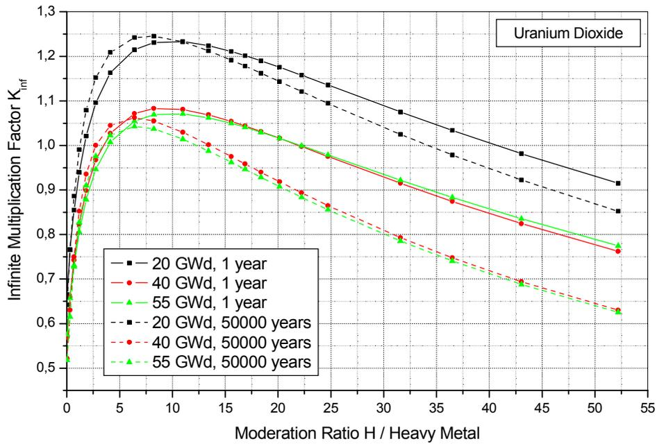
Fig. 2: Calculated  $k_{inf}$  of homogeneous spent  $UO_2$  fuel-water-mixtures for various values of burnup and cooling time.
