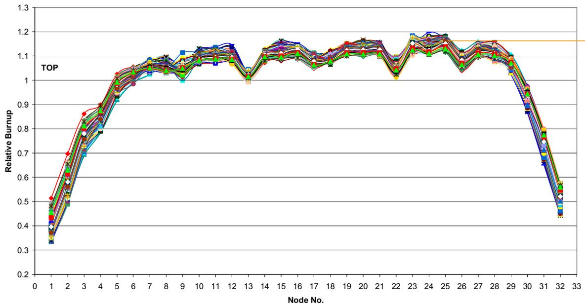
FIG. 2: Examples for axial burnup profiles obtained for fuel assemblies with 1.9 wt.-% initial enrichment.
