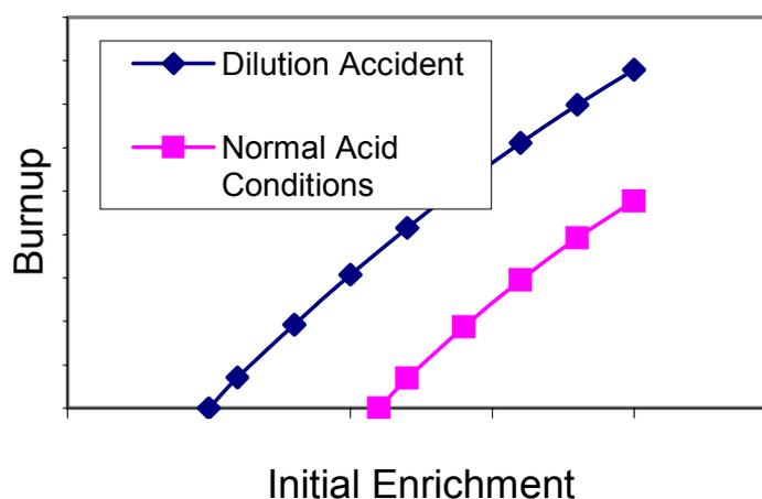
Fig. 1. Safe loading curve for normal and accident conditions.
