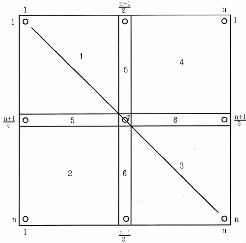
FIG. 27. Division of a  $n \times n$  fuel rod lattice in 7 zones (for odd numbers  $n$ ).
