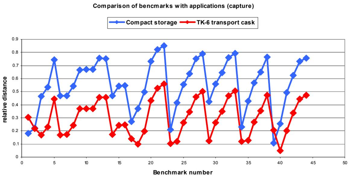
Fig. 5. Relative distance of homogeneous MOX benchmarks from applications for 5 group capture.
