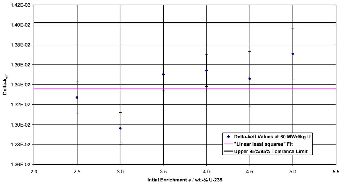
FIG. 11. Isotopic validation:  $\Delta k_{eff} (e | B_{max}) = f(e)$ .
