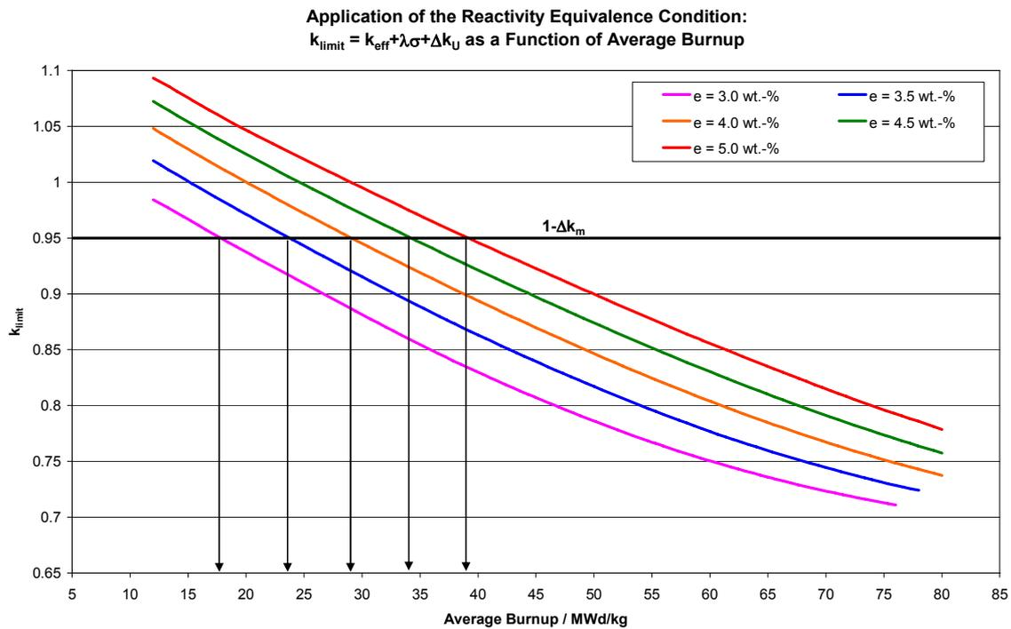
FIG 4. Illustration of the determination of a loading curve.
