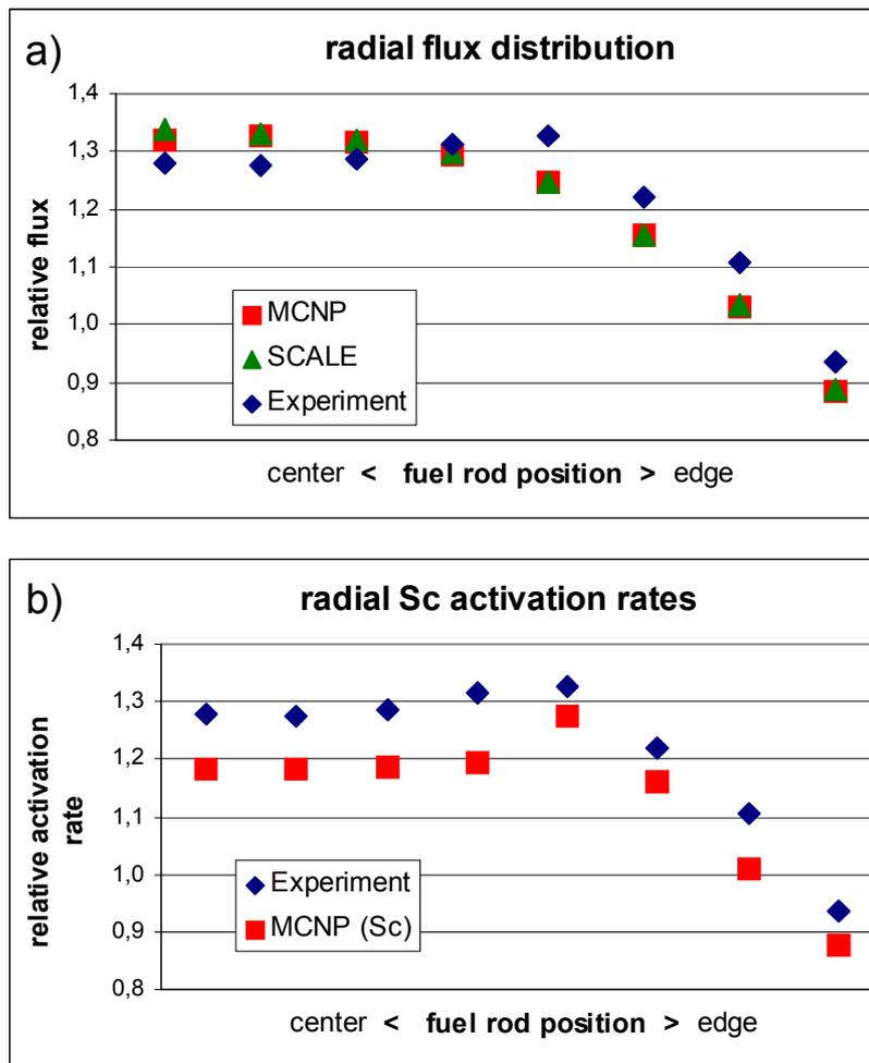
Fig. 6: Flux along the  $x=0$  axis: (a) calculation values for relative flux, (b) calculation values for relative Sc activation rates.
