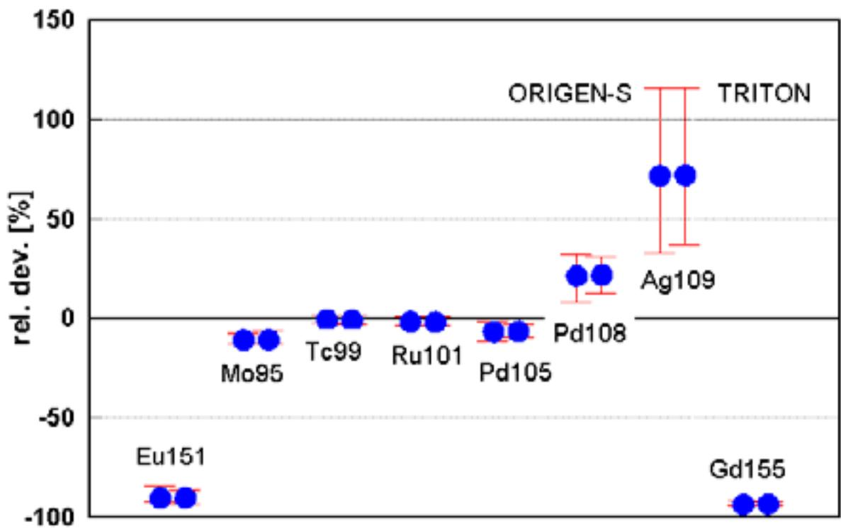
Fig.2.2c Deviation of nuclide concentration, experiment Novovoronezh 2 (8 samples).
