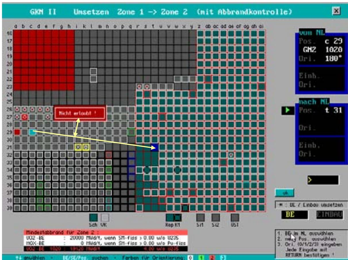
FIG. 8. Example for the interlock logic schemes applied by ALFA to the planning of fuel handling operations under the action “transfer to region II”.
