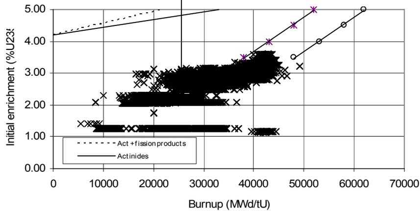
FIG. 1. Limit curves for BUC in CLAB compared to 17512 PWR assemblies.
