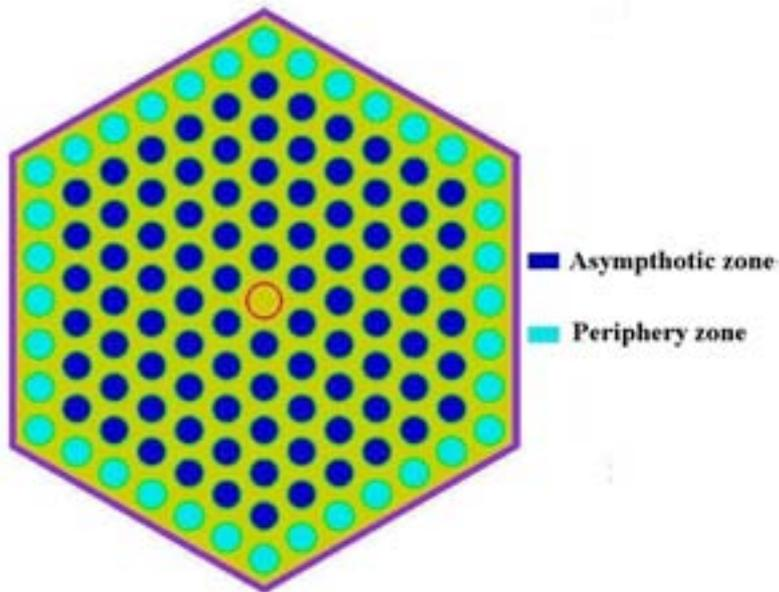
FIG. 1. WWER-440 spent fuel assembly (x-y plane). Visualization by KENO VI.
