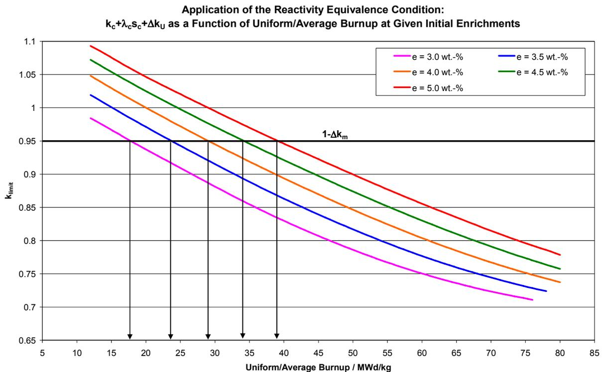
FIG. 5. Illustration of determining a loading curve (If the left-hand side of relation (2.1) is presented as a function of the uniform burnup then end effect and horizontal effect have still to be included according to section 2.3.).
