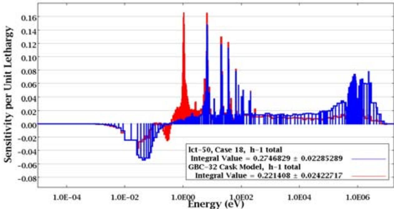
FIG. 1. The two curves show the sensitivity of  $k_{eff}$  to changes in the total hydrogen macroscopic cross sections for a burnup credit cask model (red curve) and for a critical experiment model (blue curve). “Coverage” is provided by the experiment wherever the blue curve bounds the red curve.
