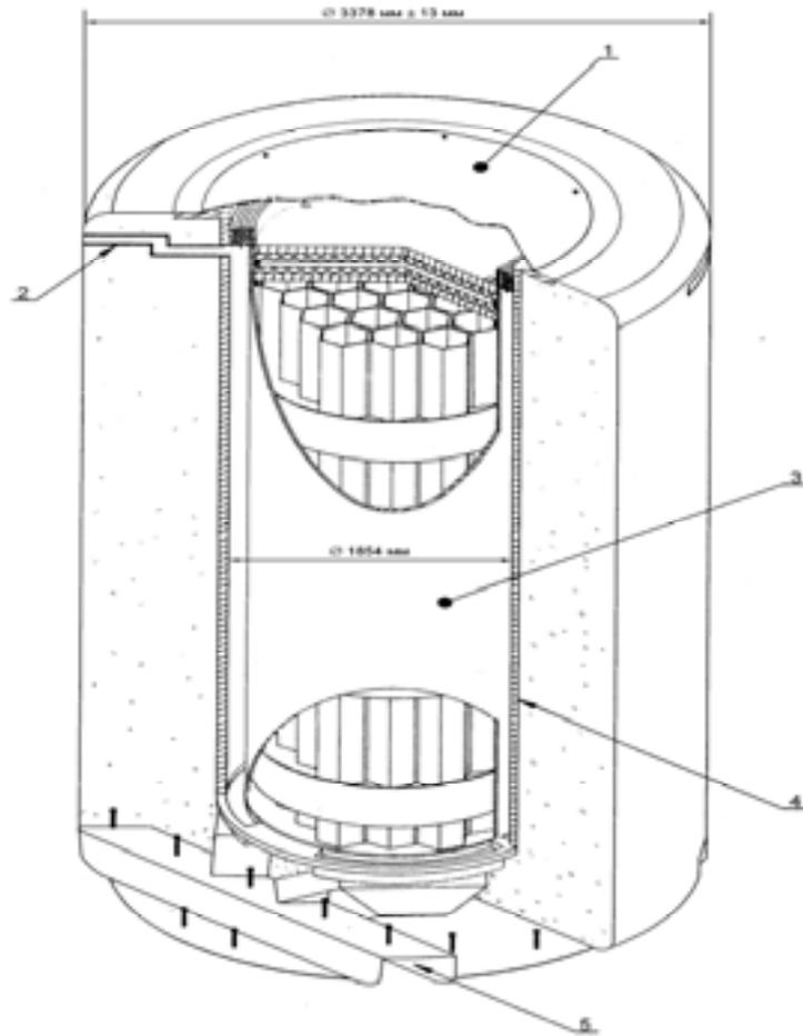
1 – cask lid; 2 – air outlet; 3 – sealed storage basket; 4 – coating; 5 – air inlet and guides for transportation
