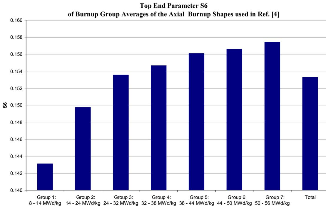
FIG. 16. Top end parameter  $S_6$  of burnup group averages of the axial burnup shapes used in Ref. [4].
