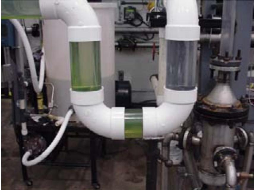
*FIG. 5. Flow visualization of injected coolant mixing with fluid in a transparent loop seal.*
