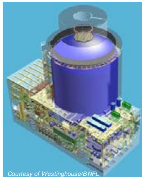
FIG. 3. AP1000 containment and passive containment cooling system (PCCS).
