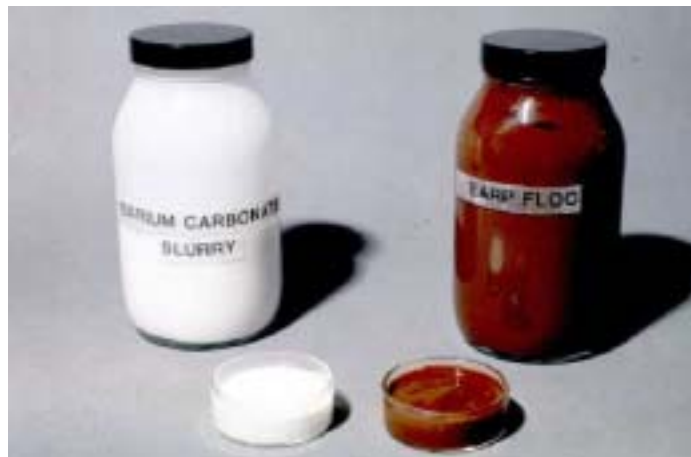
FIG. 4. Barium carbonate slurry from THORP and iron floc from the Enhanced Actinide Removal Plant.
