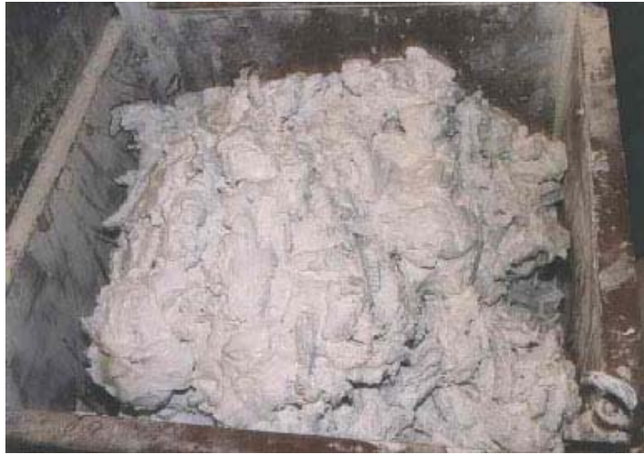
FIG. 9. Example of simulated corroded Magnox fuel element cladding waste, which has been stored underwater — containing large pieces.
