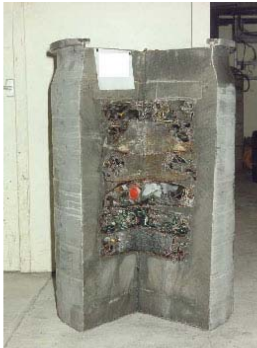
FIG. 7. Example of supercompacted plutonium contaminated waste encapsulated in the Waste Treatment Complex.
