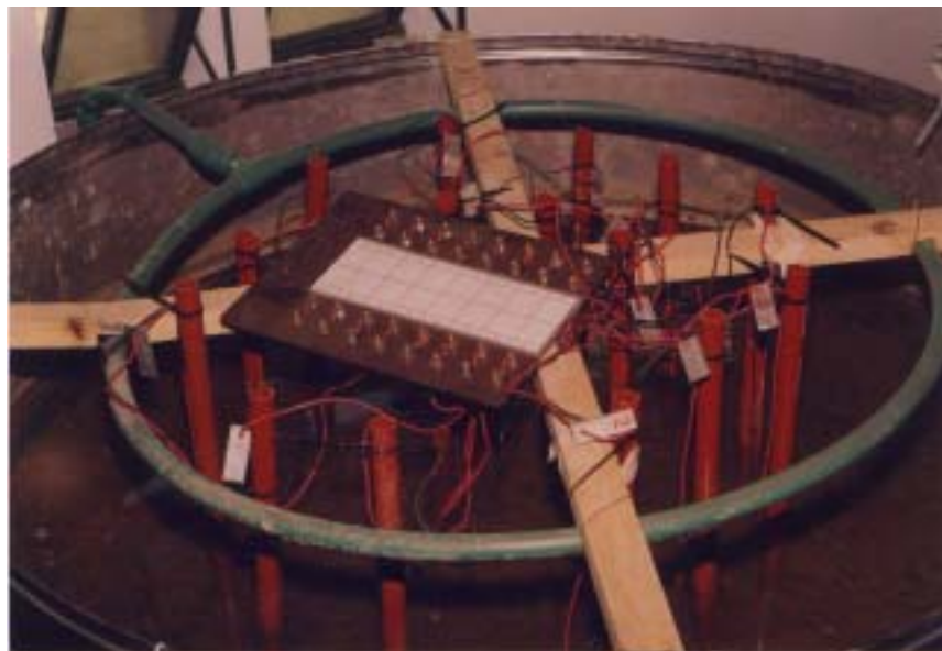
FIG. 4. Corrosion test electrodes array.
