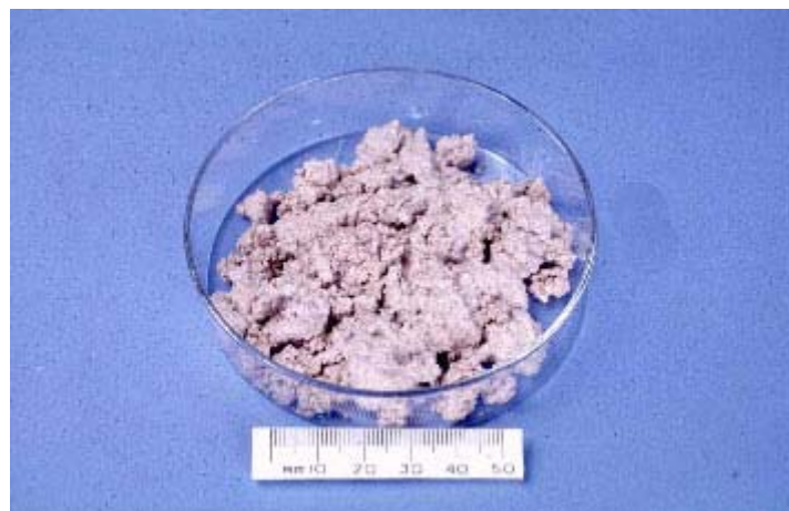
FIG. 8. Example of simulated corroded Magnox fuel element cladding waste, which has been stored underwater.
