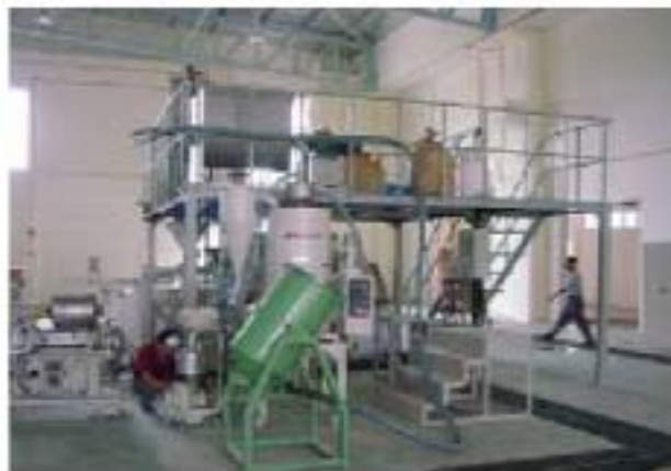
FIG. 9. A twin-screw compounder for polymer blend/composites processing.
