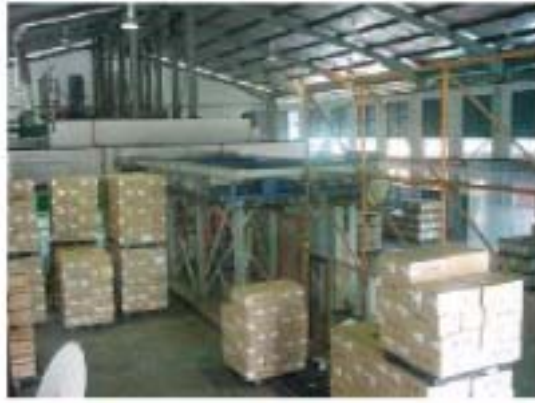
FIG. 4. SINAGAMA: Gamma Sterilization plant for sterilization of medical disposable items, food items and other products.
