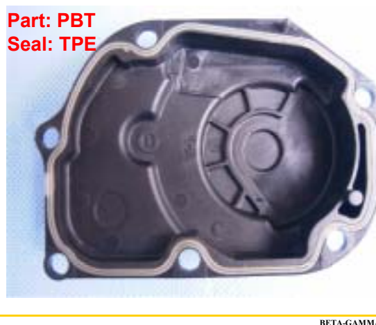
FIG. 8. Cross-linked seal produced from thermoplastic elastomer (TPE).
