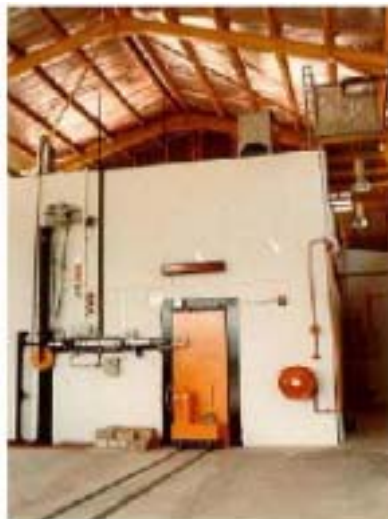
FIG. 6. RAYMINTEX – Radiation plant for prevulcanization of natural rubber latex.
