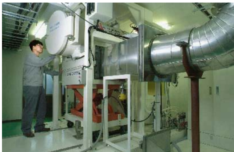
FIG. 8. Pilot plant of cleaning flue gas of municipal waste incineration plant.
