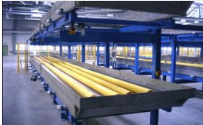
FIG. 4. Irradiation of tubes with a length of up to 12 meters.
