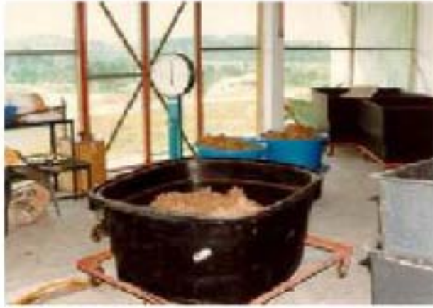
FIG. 7. STERIFEED. Animal feed plant for processing of oil palm fibers waste into animal feeds.
