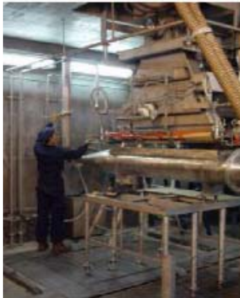
FIG. 8. Irradiation vessel for flue gas treatment using electron beam.
