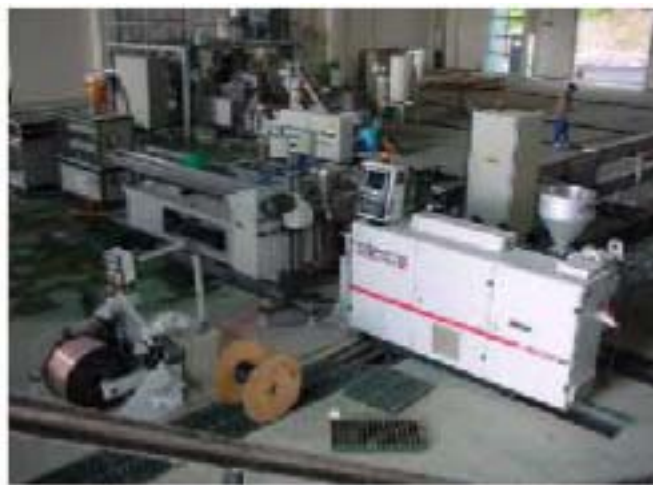
FIG. 10. Extrusion machine for profile and wire insulation.
