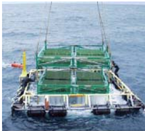
FIG. 1. Pilot plant of rare metal recovery from sea water using adsorbent produced by radiation processing.
