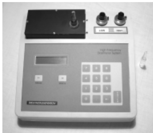
FIG. 3. Oscillometric reader for evaluation of ECB dosimeters
