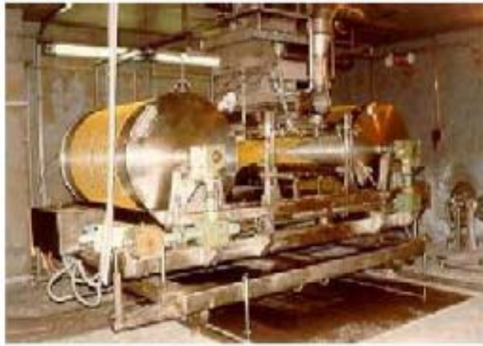
FIG. 5. ALURTRON: Electron beam accelerator, 3.0 MeV, 30mA, with handling facility for research and continuous irradiation of wire and tubes.
