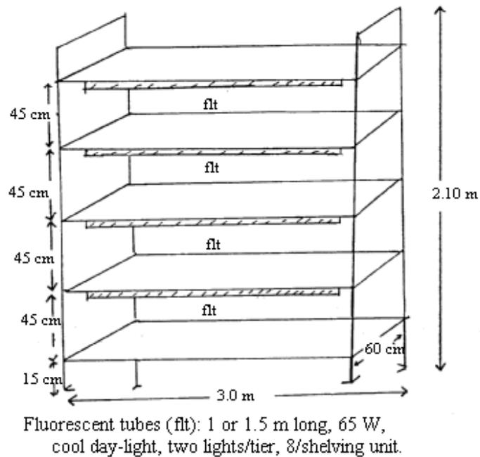
FIG. 2. Shelving unit made from angle iron.
