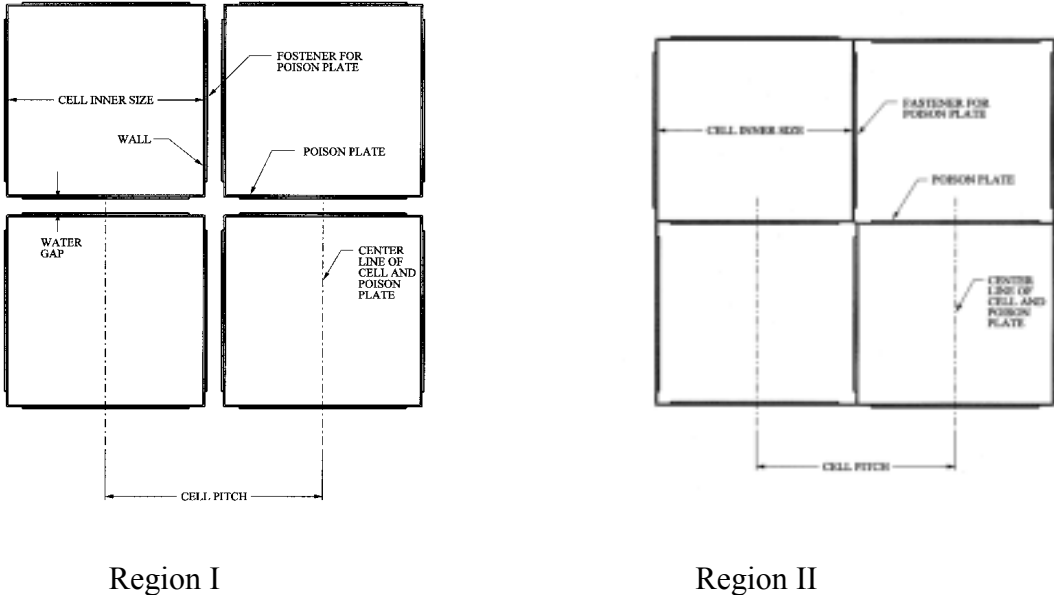
FIG. 1. The Geometry of the Spent Fuel Storage Cell
