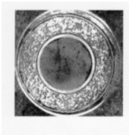
FIG. 4.13. Structure of tubular fuel element for BAES with U-9Mo alloy dispersed in Mg matrix. External diameter — 20 mm.
