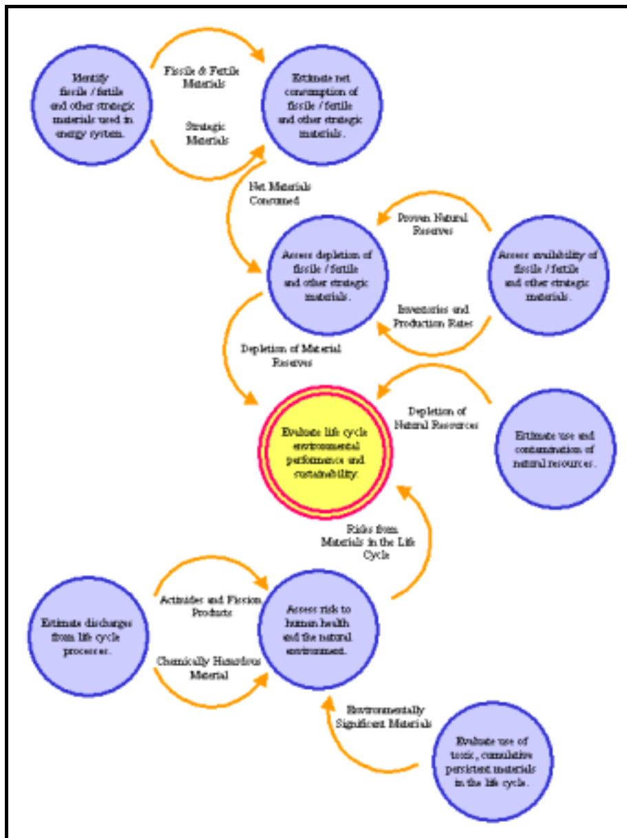
Figure 4.2.3. Information diagram for application of MFA/LCA to evaluation of environmental performance.
