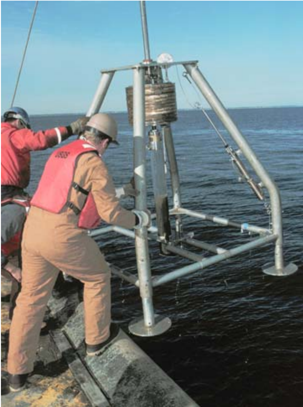
Fig 1. Hydraulically damped corer sampler.
