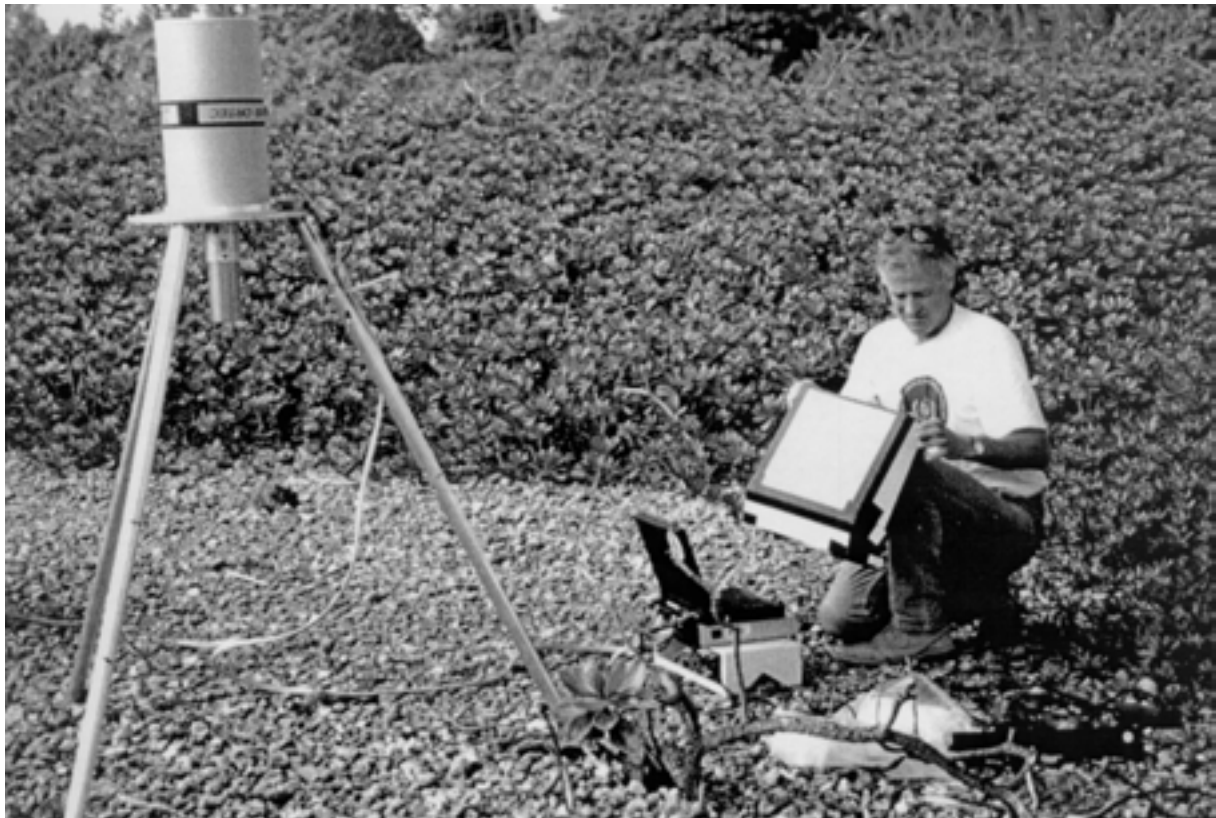
FIG 10: In-situ gamma measurements using high purity Ge detector.
