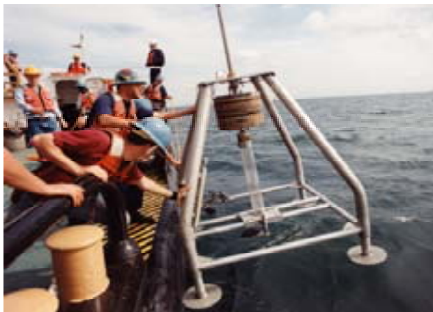
Figure 2. U.S.G.S. hydraulically damped gravity/piston corer. This instrument takes sediment cores up to 60 cm long with minimal disturbance of the water-sediment interface. Design plans are available from the author.
