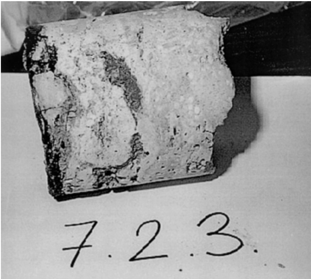
FIG 4: 10 cm Bedrock core with porous structure
