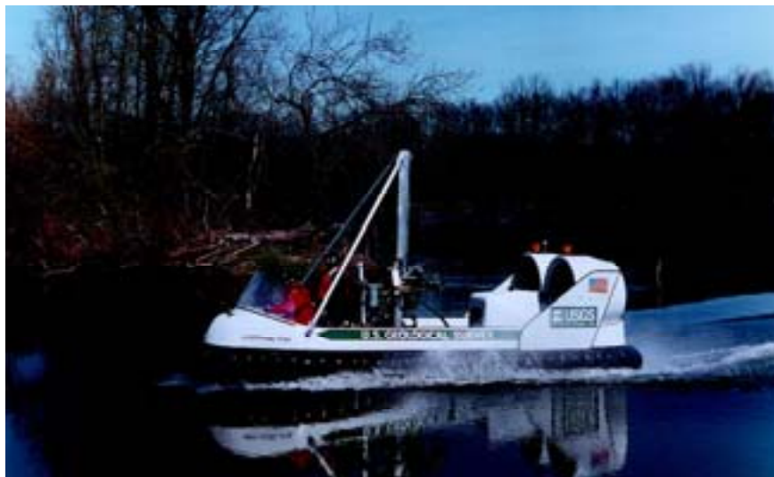
Figure 8. U.S.G.S. HoverProbe a coring platform designed on a hovercraft. This vessel is being used to collect piston and gravity cores in shallow water environments that are difficult or impossible to reach with conventional boats. Rotary drilling and vibra-coring is also possible from this platform. More information on this vessel can be obtained from Wayne Newell or Donald Queen, USGS, Reston VA.
