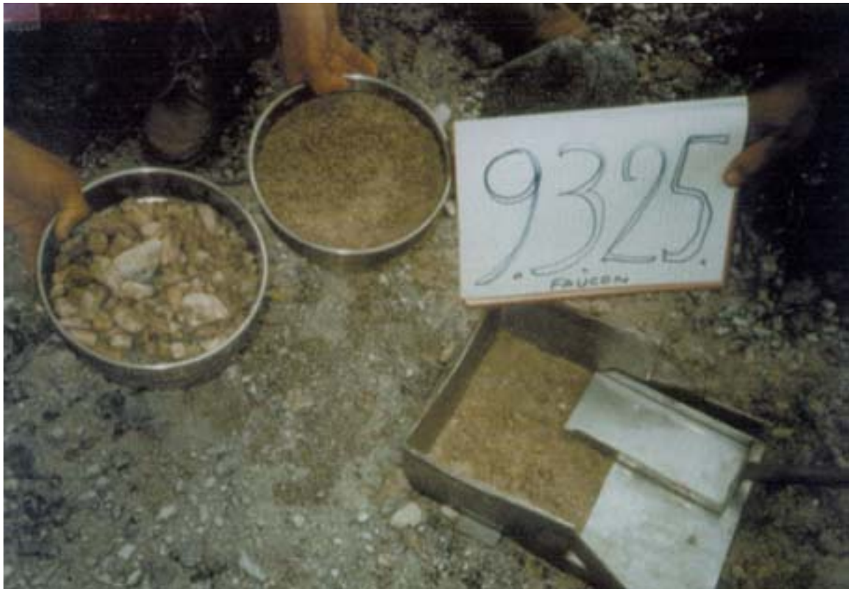
FIG 1: Template used for topsoil sample collection. The sample was sieved and big stones were discarded.
