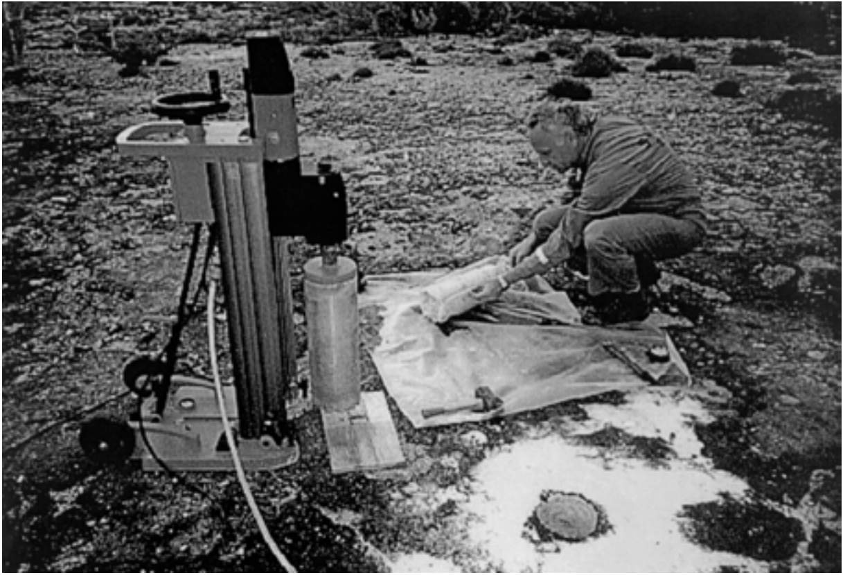
FIG 6: Bedrock sampling with core drilling equipment
