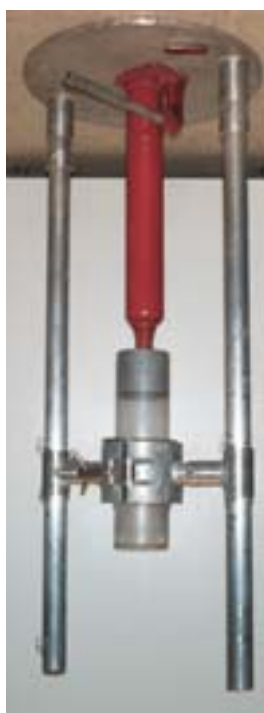
Figure 3. Core extrusion rack. An adjustable clamp held between uprights hold a core barrel vertically. A piston inserted at the bottom of the sediment core extrudes the sediment under controlled movement of the hydraulic jack. Sediments are sliced off the top of the core barrel with depth resolution of 0.5 cm.
