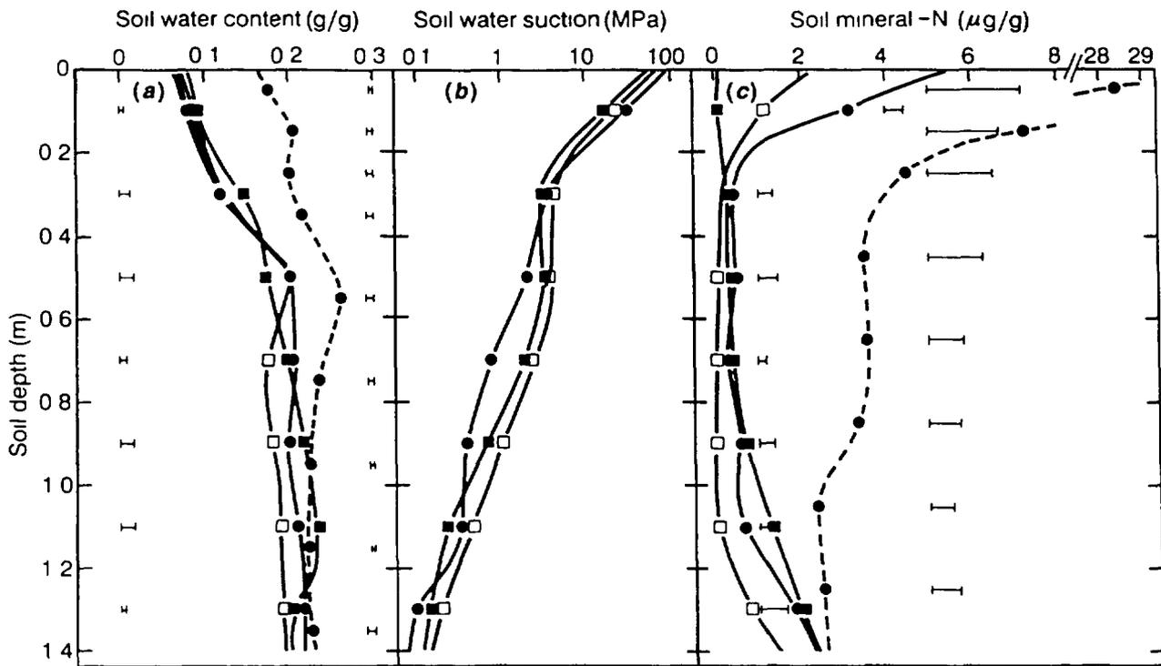
FIG 4 Soil profiles of (a) water content (b) water suction and (c) mineral-N concentration, sampled at maturity (solid lines) of wheat crops following canola (●), Indian mustard (□) and wheat (■) Water content and mineral N at sowing (dashed line) for the wheat following wheat are also presented. Horizontal bars represent standard errors of means [9]
