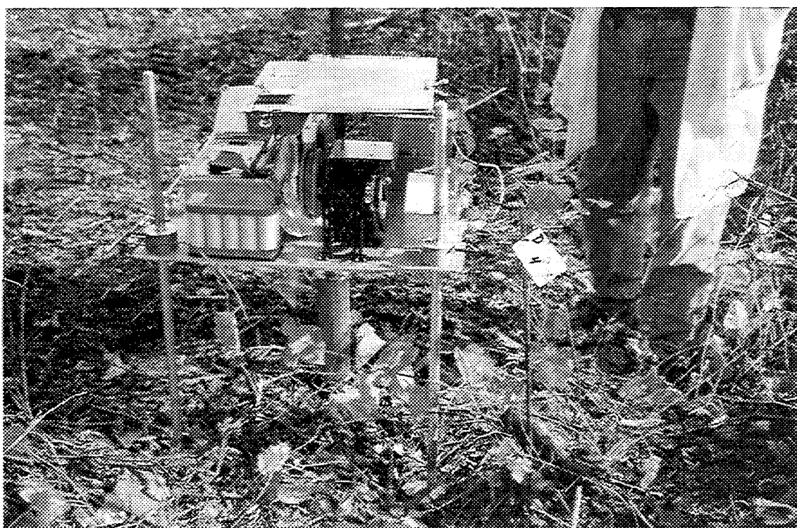
FIG. B-2. The field instrument used to log the depth profile of the dose rate in a borehole.
