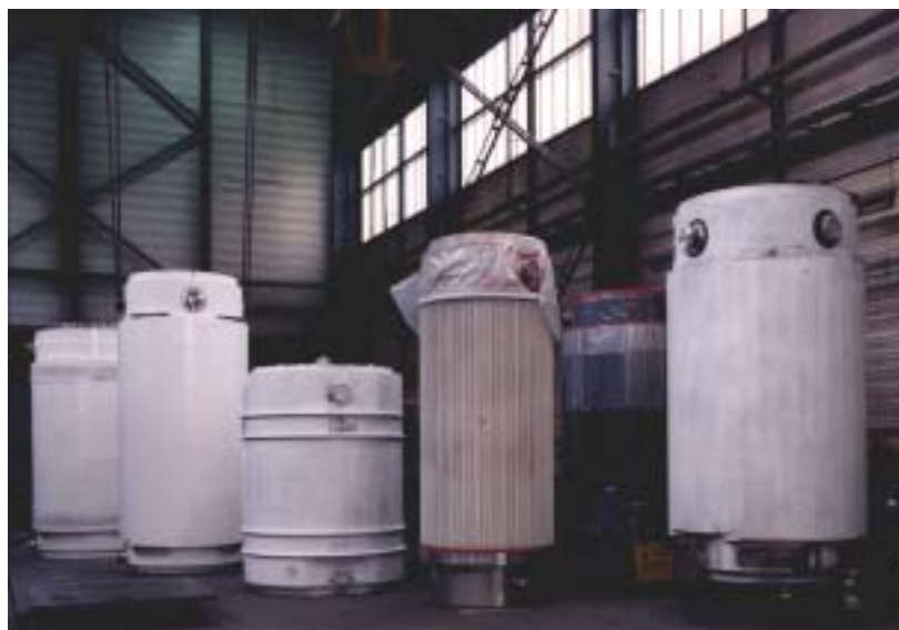
FIG. 5. Various designs of the TN TM 24 Family.
