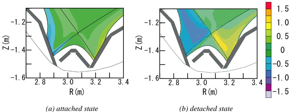
Fig.2 2D spatial profiles of parallel Mach number in the divertor region for the W-Div.
