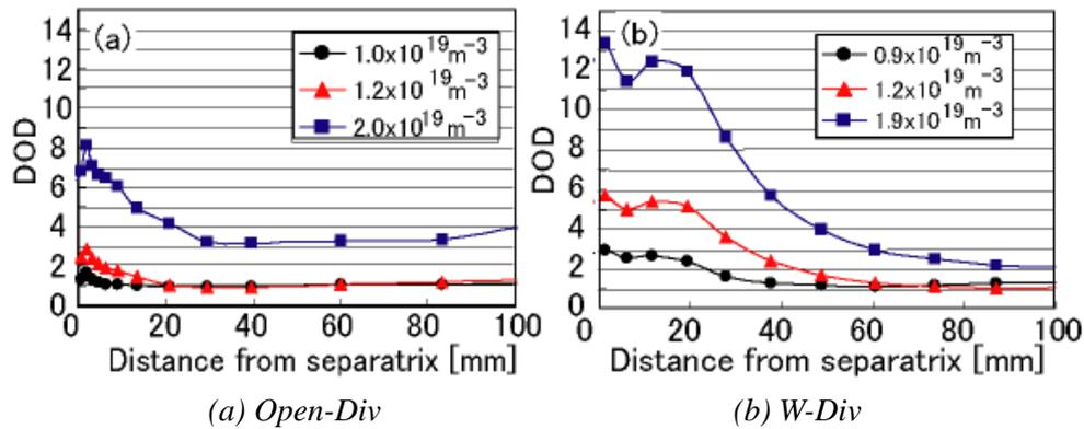
Fig.7 Radial profiles of the DOD (Degree of Detachment) at the outer target plate.
