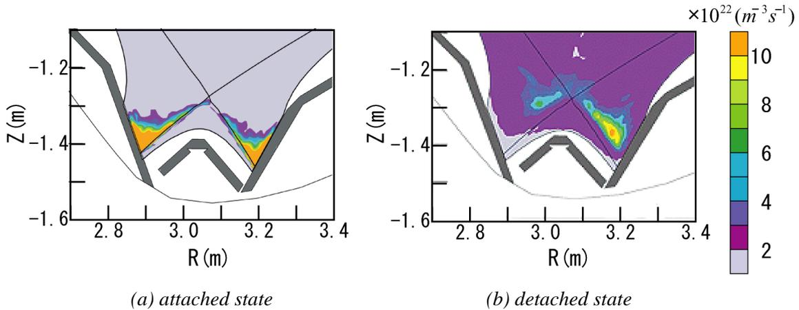
Fig.4 2D profiles of the ionization source density  $S_i$  in the divertor region for the W-Div.
