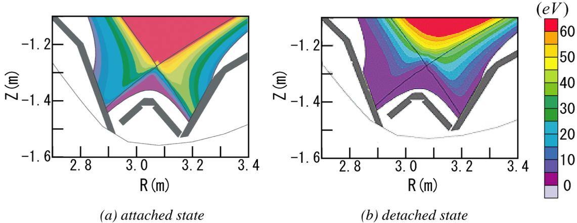
Fig.3 2D profiles of electron temperature  $T_e$  in the divertor region for the W-Div.
