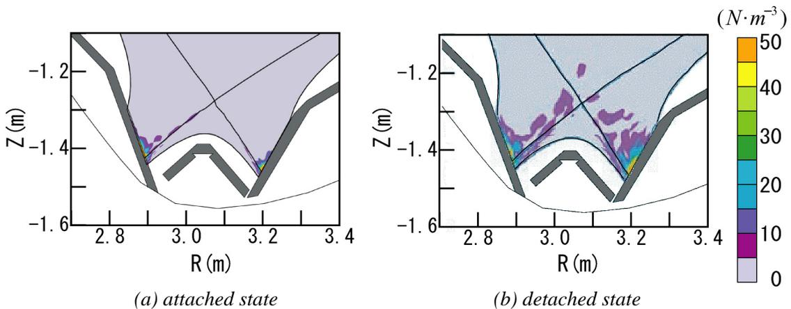
Fig.5 2D profiles of the momentum loss density  $S_m$  in the divertor region for the W-Div.
