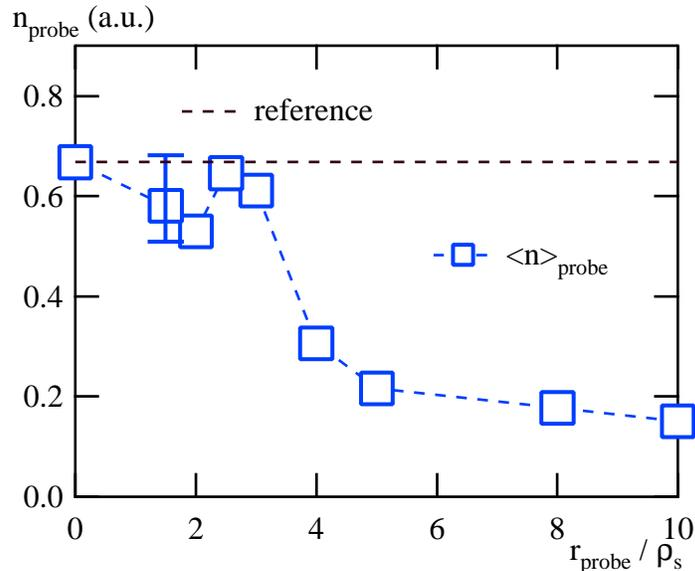
FIG. 2 : Change in the measured density versus the size of the probe tip. The error bars indicate the magnitude of the fluctuations during the averaging
