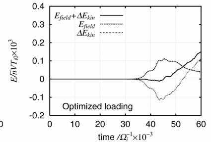
Fig.6: Time history of the field energy, the kinetic energy, and the total energy in the Cyclone base case with a Maxwellian particle loading (left) and an optimized particle loading (right). The energy conservation property is improved by using the optimized particle loading.
