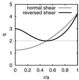
Fig.1: Safety factor profiles of normal and reversed shear configurations.
