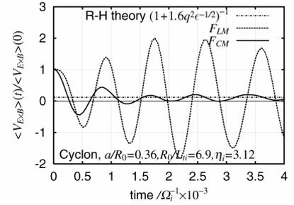
Fig.8: Time history of flux surface average zonal flows in zonal flow damping tests. Rosenbluth-Hinton theory is recovered by using  $F_{CM}$ .
