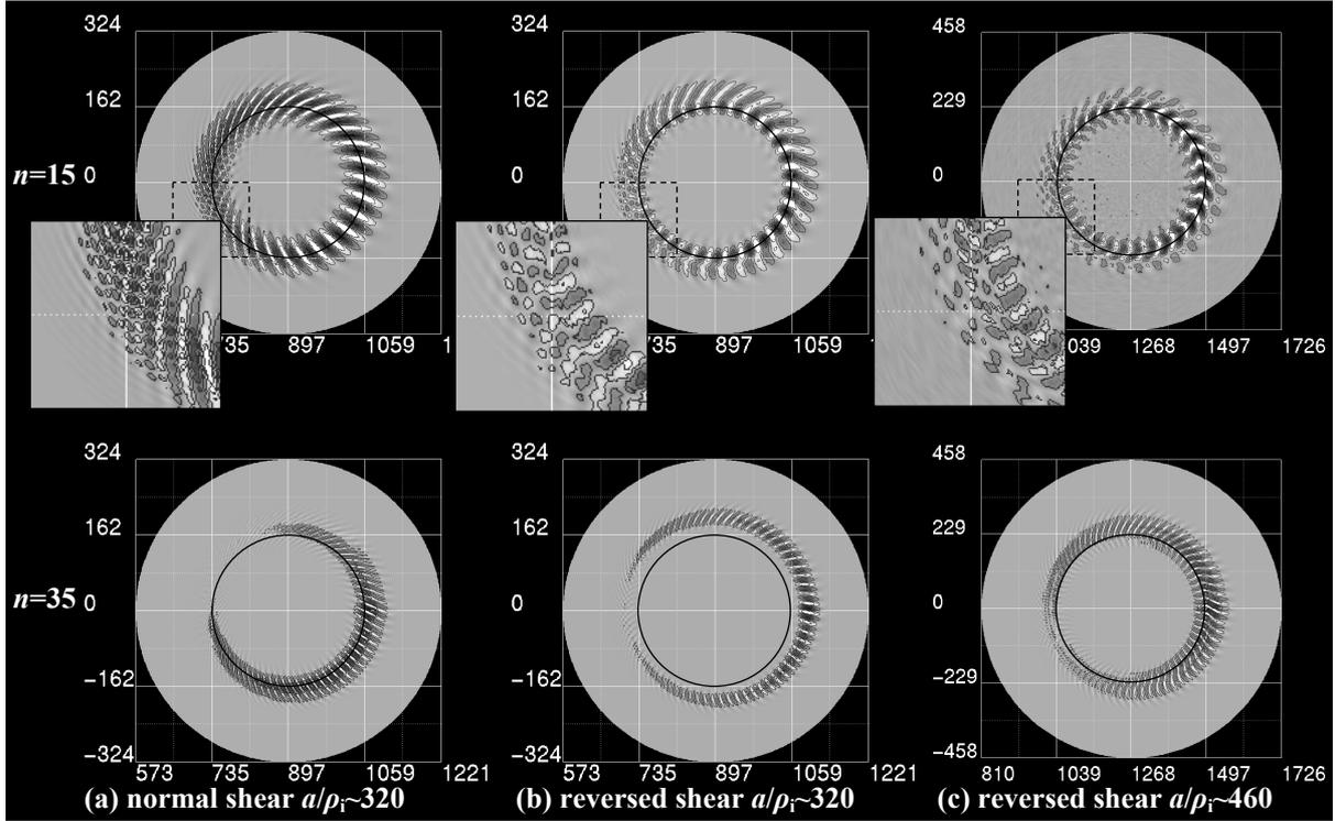
Fig.4: Typical eigenfunctions of the low-n and high-n modes in the normal and reversed shear configurations. In the  $q_{min}$  region, the low-n global mode shows a coupled mode structure between the slab and toroidal ITG modes. In the case (b), the high-n mode ( $n=35$ ) is excited in the outside of the  $q_{min}$  surface.
