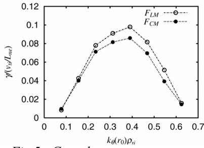
Fig.5: Growth rate spectrum plotted for the Cyclone base case;  $R_0/a=0.36$ ,  $a/\rho_{ti}\sim 152$ ,  $R_0/L_{ti}=6.9$ ,  $\eta_i=3.12$ , and  $q=1.4$  at  $r=0.5a$ .
