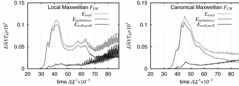
Fig.7: Time history of the fluctuation field energy in the Cyclone base case with the local Maxwellian  $F_{LM}$  (left) and the canonical Maxwellian  $F_{CM}$  (right). After the saturation of the ITG mode, spurious zonal flow oscillations grow in the case with  $F_{LM}$ .
