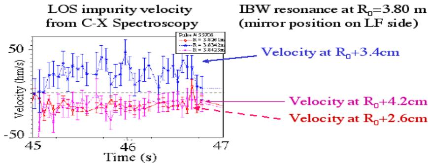
FIG.4. Time evolution of the line of sight (LOS) impurity velocity measured by charge-exchange spectroscopy (CXS) diagnostic in shot 55708. The velocity increases after the ICRF power switch-on (45.0 s). Saturation occurs during the ICRF power linear ramp-up (45.0s – 46.0 s) at a power level of about 2.5 MW.
