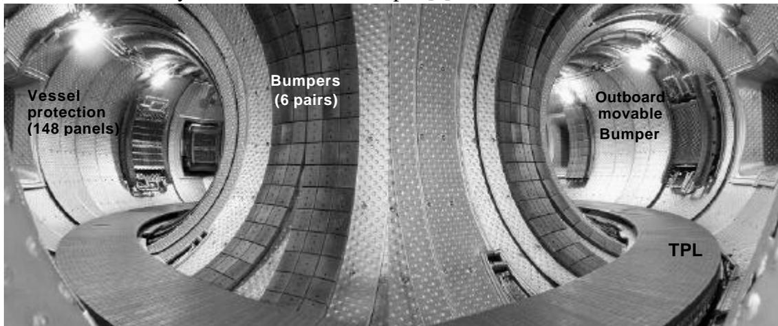
FIG. 2: Tore Supra in the CIEL configuration
