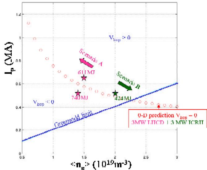
FIG. 11: Tore Supra operational domain for long pulses. The circles display the 0-D prediction of zero loop voltage at 3MW LHCD + 3MW ICRH. The stars represent actual 2002 Tore Supra discharges labelled with their total coupled energy.
