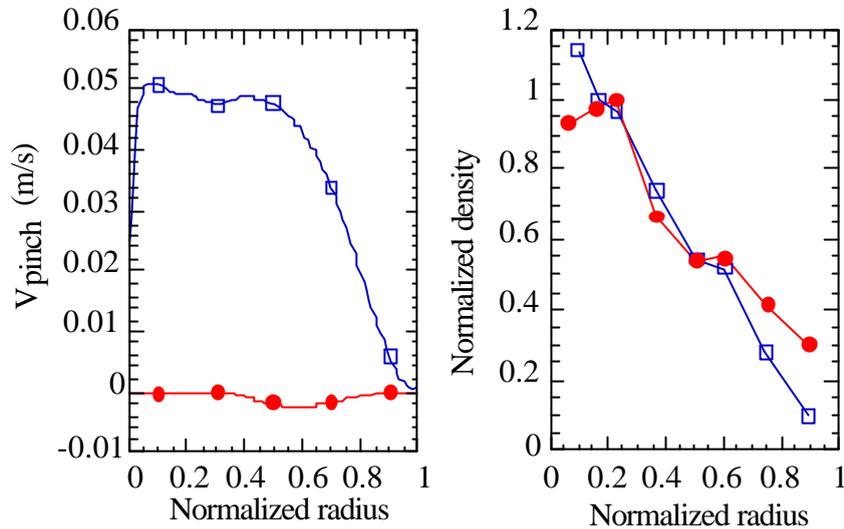
Fig. 13: Radial profile of neoclassical pinch (left) computed with NCLASS and normalized density (right), for ohmic (squares) and full LHCD phases (circles) in discharge shown in Fig. 14
