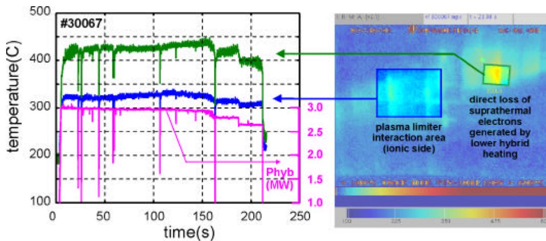
FIG 5 : Typical time evolution of the TPL surface temperature in the convective zone (blue) and in the hot spot zone (green). The lower hybrid power is also indicated [13].
