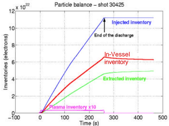
FIG 9 : Typical particle balance for a long discharge, showing the injected, extracted, plasma and wall inventories Note that the plasma inventory is multiplied by 10 to be seen on the figure.
