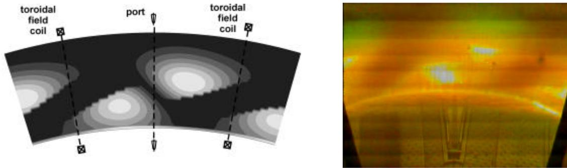
FIG. 4 : Comparison of heat flux pattern as calculated from simulations (left) and recycling pattern measured by a CCD camera (right). The main experimental features (loaded areas alternating with shadowed areas) are well reproduced by the simulations.
