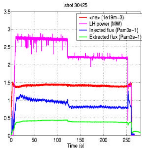
FIG. 8 : typical time evolution of the plasma volume averaged density during a long discharge. Also shown is the lower hybrid power and the fluxes injected by gas puff and extracted by the TPL
