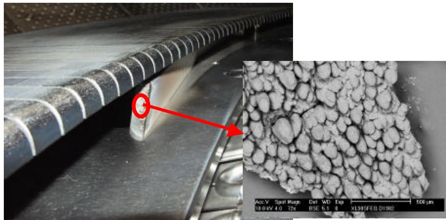
FIG.7 :View of the layer deposited on the neutralizer surface in the machine and imaging of this layer by electronic microscopy
