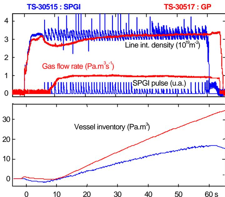
FIG. 10: Comparison of feedback gas injection from conventional gas puff (GP) and supersonic pulsed gas injection (SPGI) for the same plasma density target ( $I_p=0.67\text{MA}$  and  $P_{\text{LHCD}}=2.8\text{MW}$ ).
