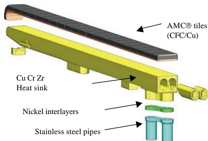
FIG. 1: Schematics of the high heat flux TPL finger element (length 0.5m, 2.5cm depth and width). The 21 AMC tiles (6mm thickness), 3 plugs and Ni/SS cooling pipes are EB welded to the heat sink
