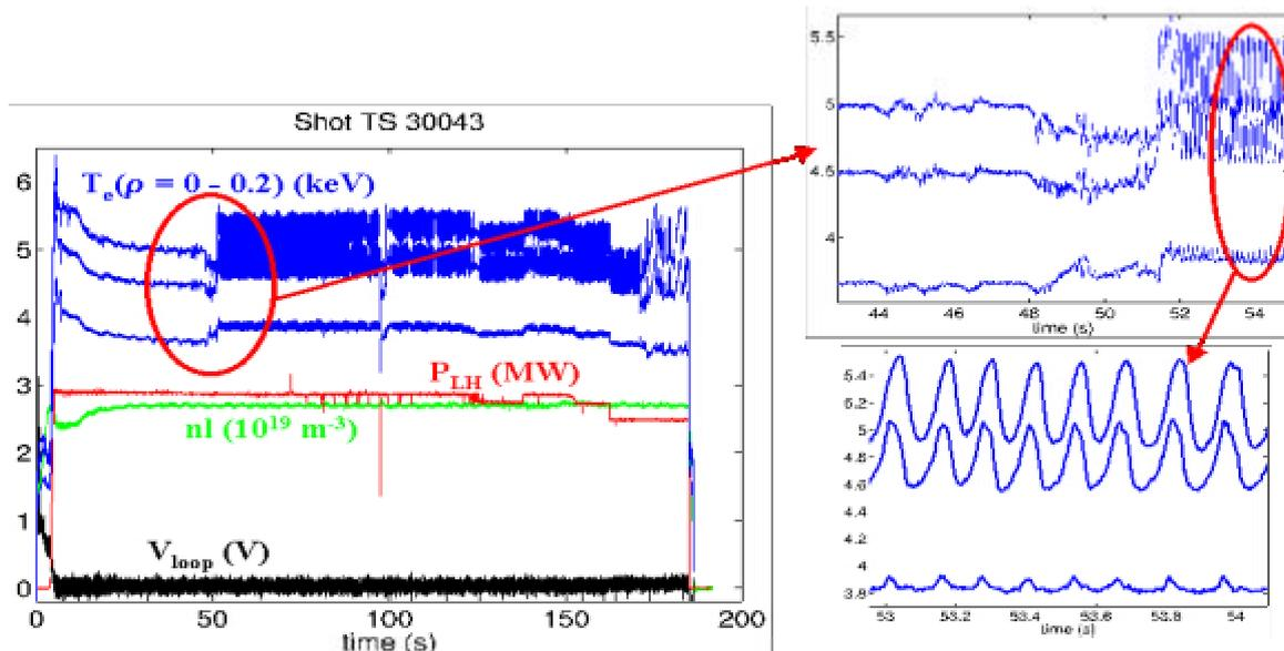
FIG. 12: Tore Supra #30043. Zoom on the central electron temperature behaviour.
