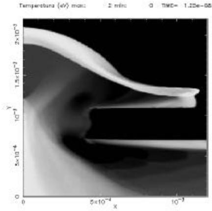
FIG. 2. Electron temperature at 12.5ns.
