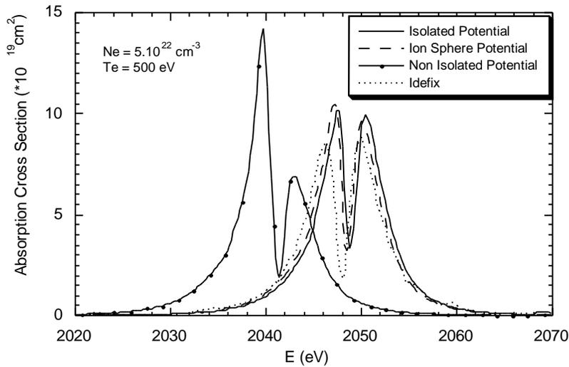
FIG. 1. Absorption cross section for the aluminum Lyman **b**.  $G = 1.1$ .
