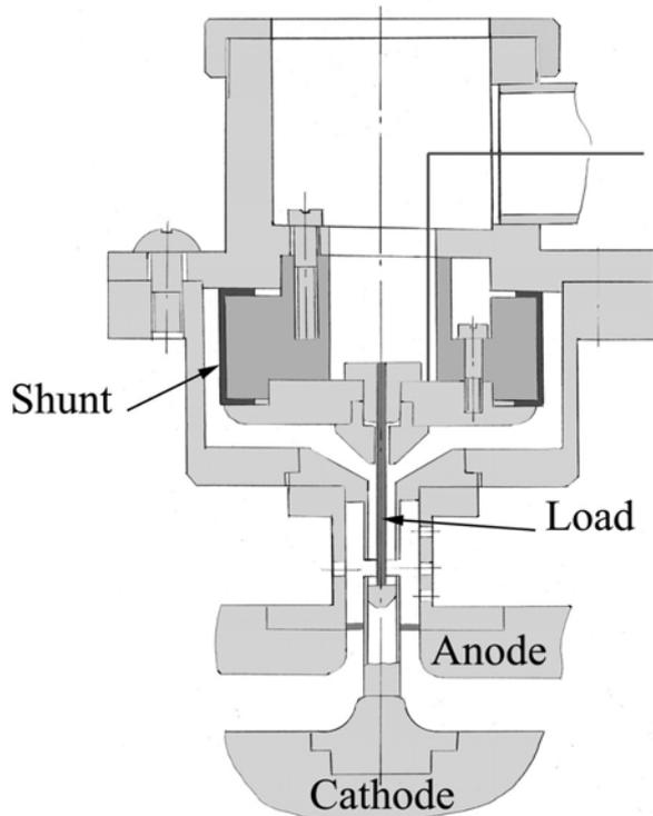
FIG. 1. The sketch of output device
