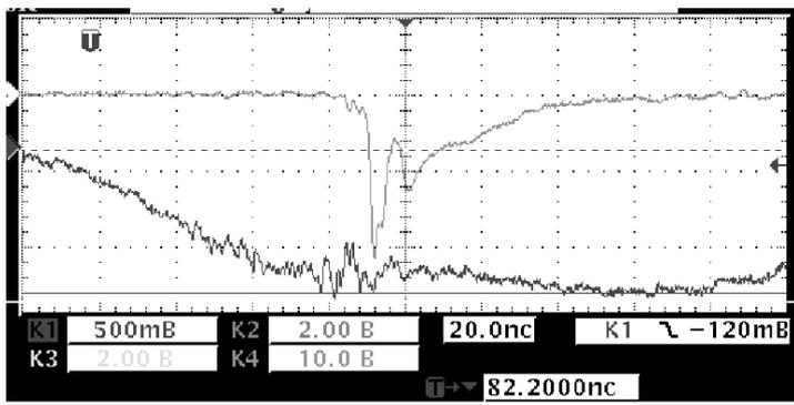
FIG. 2. The current on a load (top) and total current (bottom)
