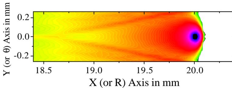
FIG.5. Mass density contours from a 2D simulation of one of 240 tungsten wires in an array on 'Z'
