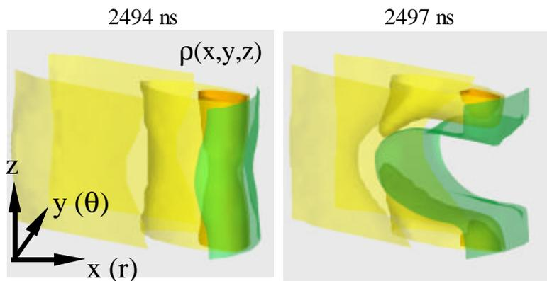
FIG.8. A 3D simulation of a 0.3mm long section of one of 300 11.5mm tungsten wires in a 20mm diameter array on 'Z', (the array axis is far away, to the left of the picture).
