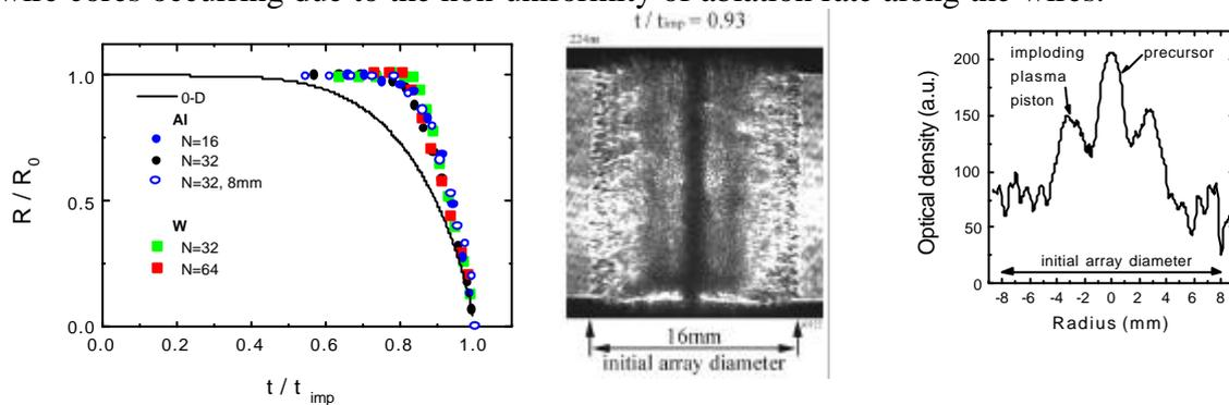
FIG.3. Normalized implosion trajectories for several Al and W arrays
