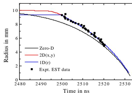
FIG.7. Comparison of simulated implosion trajectory with experimental optical streak data
