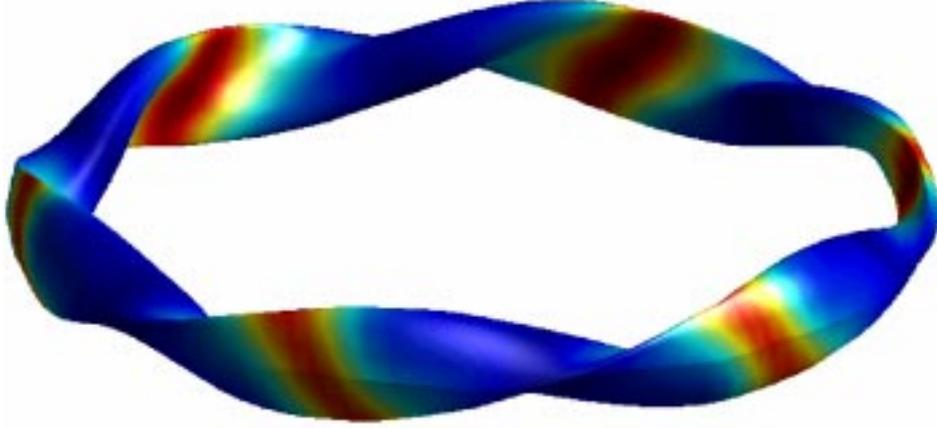
FIG. 1. Boundary magnetic surface of the optimized configuration also showing the magnetic topography. The colors define the range of the magnetic field strength (red - maximum, blue - minimum,  $(B_{\max}-B_{\min})/B \approx 0.5$ ). The characteristic feature of the configuration is the nearly vanishing curvature of the plasma column in the regions of the extrema of  $B$ .
