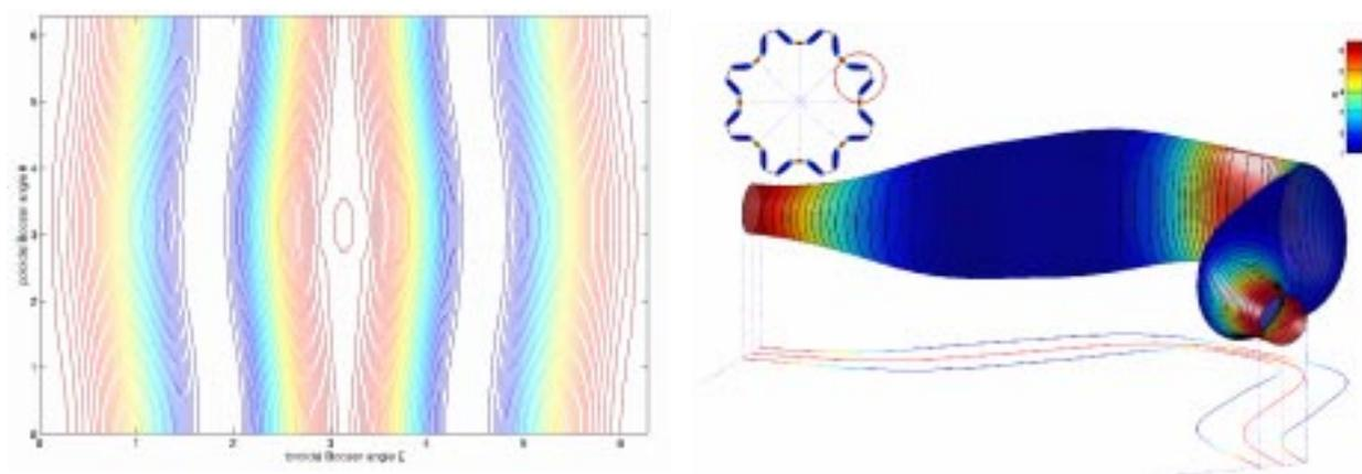
FIG. 5. Contours of  $B$  on a magnetic surface, and boundary as well as midplane field lines of one field period.
