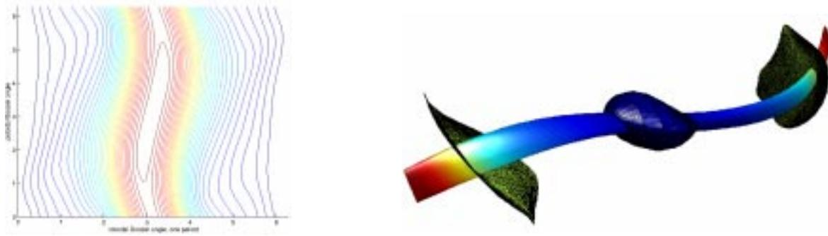
FIG. 2. Left: The contours of  $B$  on the magnetic surface at half of the minor plasma radius. It is seen that a small residual local maximum of  $B$  still exists.
