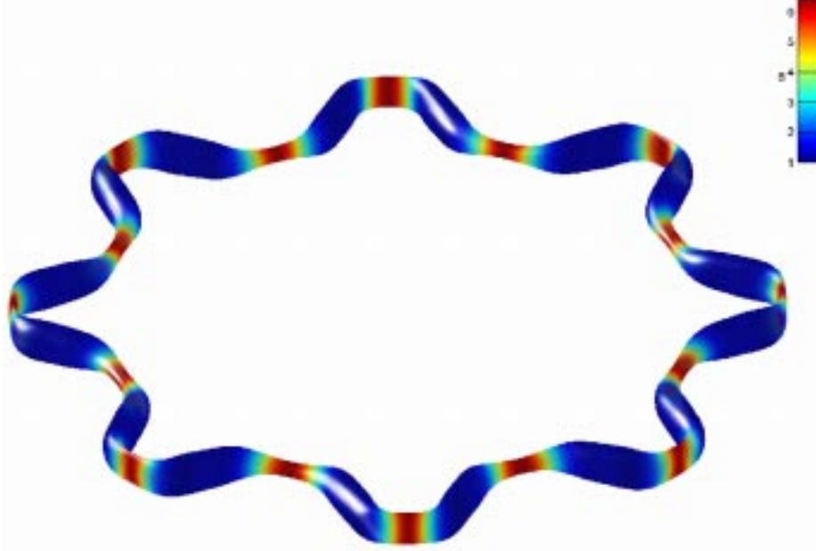
FIG. 4. Boundary magnetic surface of eight-period trap. Dimensionless parameters: aspect ratio 20.65, mirror ratio 5.84, major radius min/max 0.75,  $\langle \beta \rangle 0.1\%$ ; the  $\alpha$ -particle confinement (see Fig. 6) is assessed with device dimensions: plasma volume  $469.5\text{m}^3$  (corresponding to a volume-averaged minor radius 1.114m) and average magnetic field 5T.
