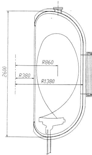
FIG. 1. KTM tokamak cross section.
