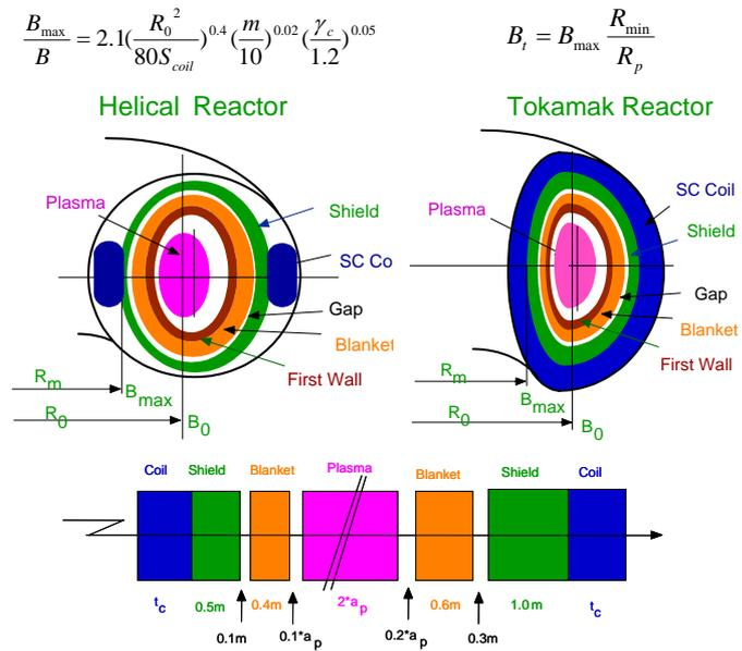
Fig. 2 Model of helical and tokamak reactor systems
