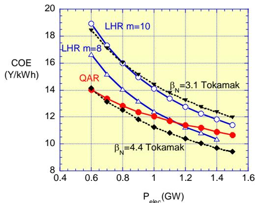
Fig.6 COE vs. electric power output
