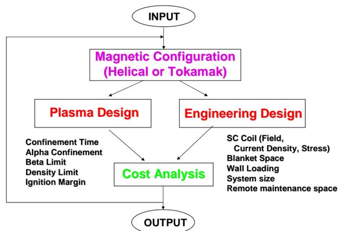
Fig.1 Flowchart of helical and tokamak system analysis
