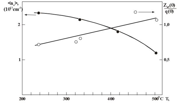
FIG. 2. Behaviour of  $\langle n_e \rangle$  and  $Z_{\text{eff}}(0)/q(0)$  during experiment with Li limiter heating.
