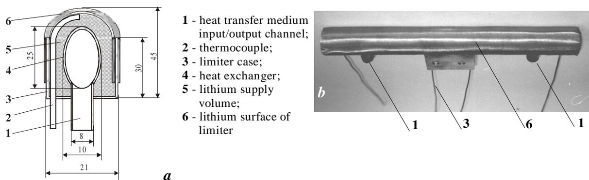
Fig. 3. Design (a) and general view (b) of the new version T-11M tokamak lithium limiter.
