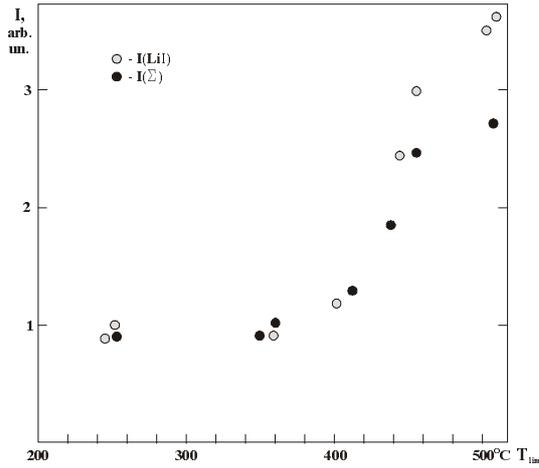
FIG. 1. Total light and LiI intensity as function of CPS temperature.
