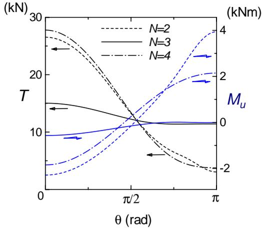
FIG. 2. Poloidal distributions of tension  $T$  and bending moment  $M_u$  in coils with circular cross section,  $R = 0.30$  m,  $a = 0.14$  m,  $B_\phi = 1.55$  T at  $r = R$ . A solid line of the winding pitch  $N = 3$  corresponds to VLC, while a dash-dotted line of  $N = 4$  corresponds to conventional FBC.
