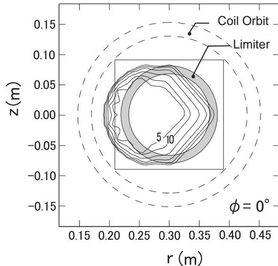
FIG. 6. Contour plot the poloidal field strength created by the helical coil with  $R = 0.30$  m,  $a = 0.14$  m,  $B_\phi = 1.55$  T at  $r = R$ . The difference of the contour level is 5 G.
