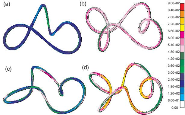
FIG. 3. Distributions of the von Mises stress in VLC ( $N = 3$ ) (a), FBC ( $N = 4$ ) (b), and normal helical coils with  $N = 3$  (c),  $N = 4$  (d).
