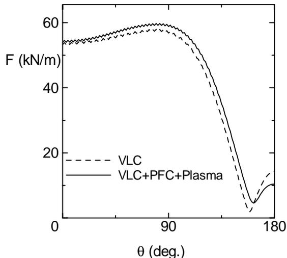
FIG. 5. Poloidal distributions of electromagnetic force acting on VLC with circular cross section,  $R = 0.30$  m,  $a = 0.14$  m,  $B_\phi = 1.55$  T at  $r = R$ . Forces due to only VLC and both VLC, PF coil and plasma are represented by dashed and solid lines, respectively.
