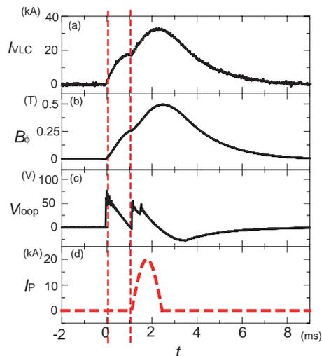
FIG. 7. Time evolutions of (a) VLC current, (b) toroidal field, (c) loop voltage, (d) expected plasma current in a two-step discharge of Todoroki-II without plasma.
