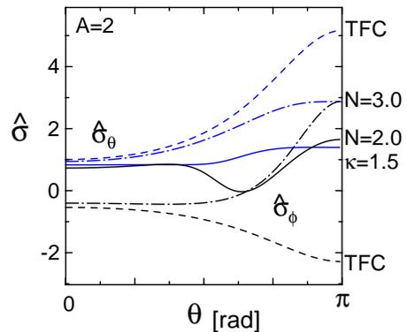
FIG. 1. Poloidal distribution of principal stress  $\hat{\sigma}$  normalized by toroidal magnetic field energy. Dashed, dot-dashed and solid lines are in the cases of conventional TF coils with circular cross section and VLCs with poloidal rotation number  $N = 3$  with circular cross section and  $N = 2$  with  $\kappa = 1.5$ , respectively.
