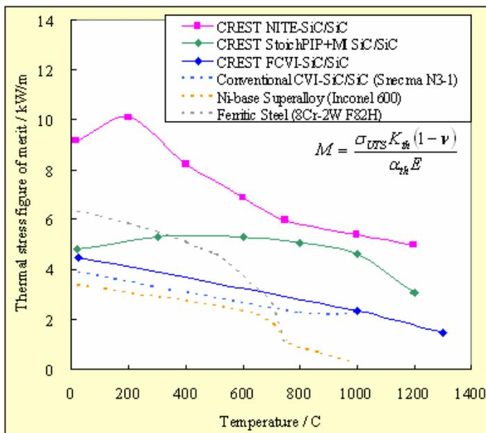
Fig. 3 Thermal stress tolerance of UD-SiC/SiC by NITE process comparing with other high temperature materials
