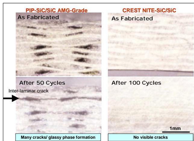
Fig.6 Microstructure change by combustion test
