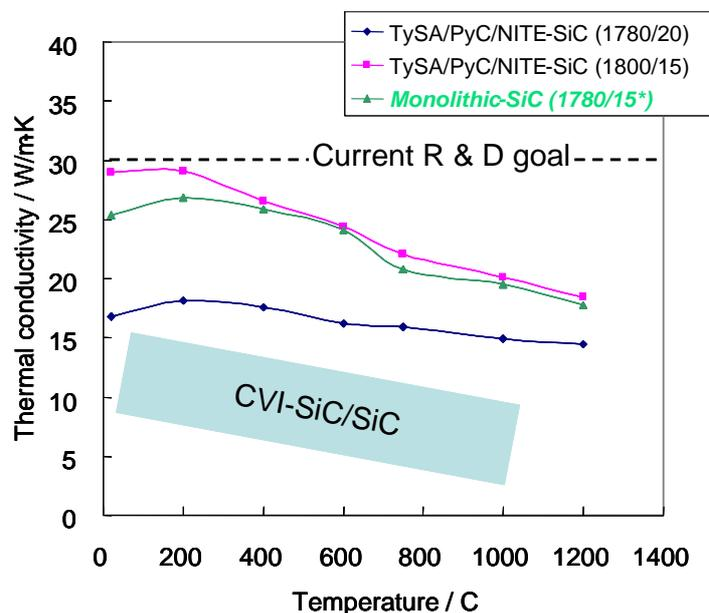
Fig. 2: Thermal conductivity of UD-SiC/SiC by NITE process
