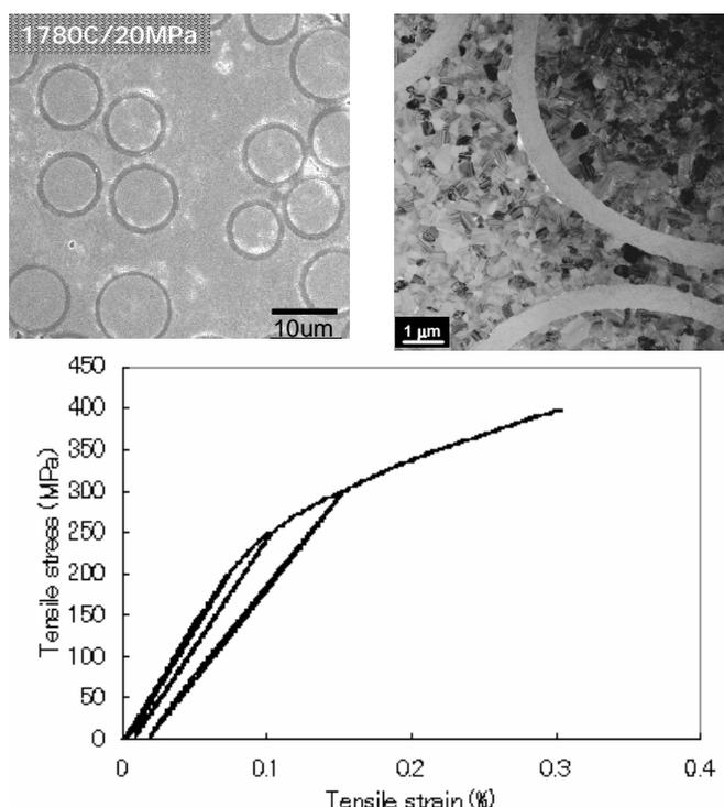
Fig.1 Representing microstructures and mechanical behavior of SiC/SiC composites fabricated through 'NITE' process.
