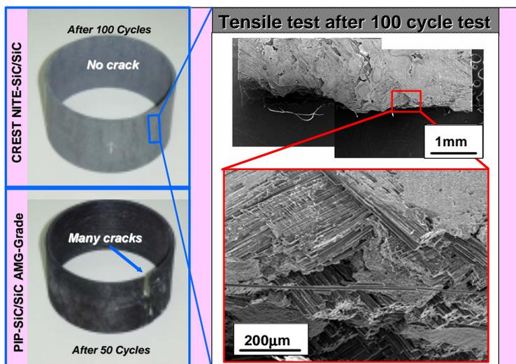
Fig. 5 Combustion test (between 1350C and 20C) results
