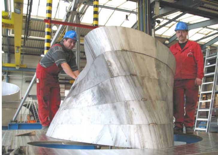
FIG. 4. Assembly of a sector of the plasma vessel (by courtesy of DWE).
