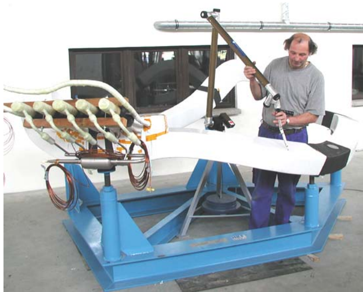
FIG. 2. Winding package of a non-planar coil (by courtesy of BNN).
