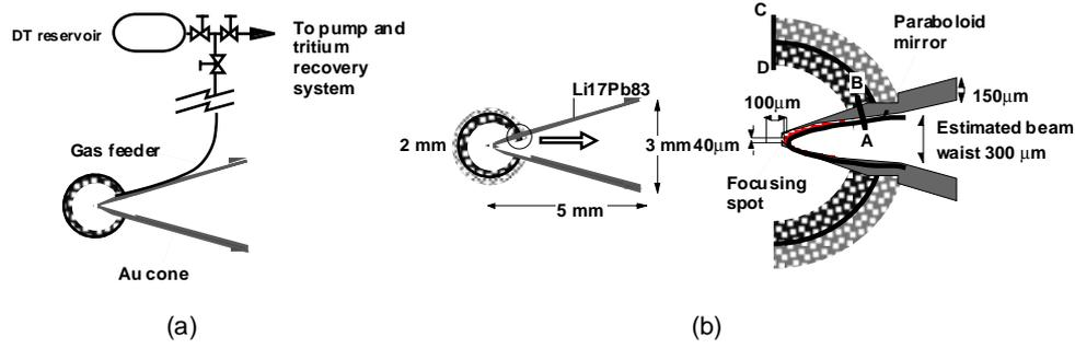
FIG. 4 Fast ignition target for FIREX experiment (a) and for reactor (b).
