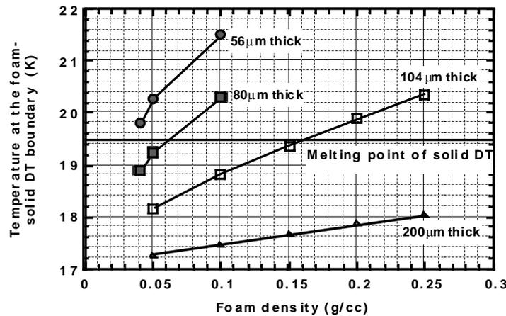
FIG. 2 Temperature at the foam- solid-DT boundary. The vapor pressure, the radius of chamber, and the injection speed are 0.05 Torr, 5 m and 300 m/s, respectively.
