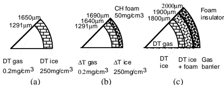
FIG. 1 Model cryogenic target (a), foam insulated target with the same mass (b) and reactor class target (c).
