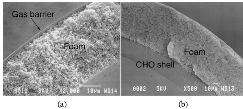
FIG. 6 Foam shell with gas barrier (a) and CHO shell coated with foam layer (b)
