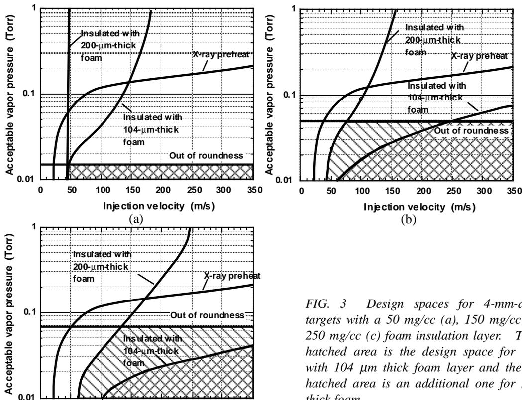
FIG. 3 Design spaces for 4-mm-diameter, targets with a  $50 \text{ mg/cc}$  (a),  $150 \text{ mg/cc}$  (b) and  $250 \text{ mg/cc}$  (c) foam insulation layer. The cross hatched area is the design space for a target with  $104 \mu\text{m}$  thick foam layer and the oblique hatched area is an additional one for  $200\text{-}\mu\text{m}$ -thick foam.
