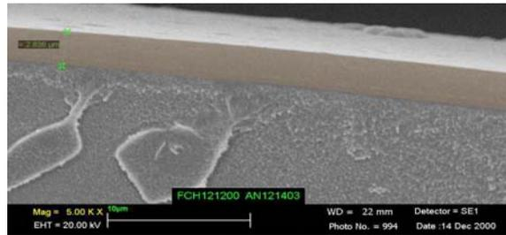
$\sim 3$   $\mu\text{m}$  thick polymer coating deposited on a mandrel using fluidized bed technology
