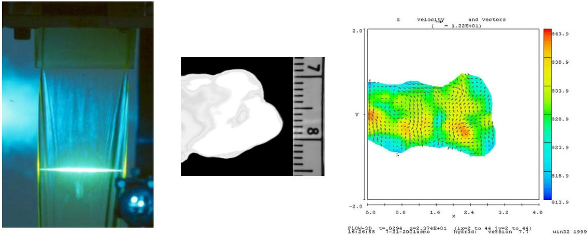
Fig. 1. Characterization of surface quality of turbulent 10 cm  $\times$  1 cm water jet: Laser induced fluorescence diagnostic at GT (left), resulting image of edge region (center), 3D simulation carried out by UCLA (right).
