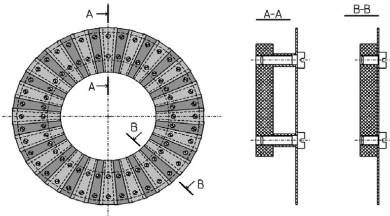
FIG. 2. Layout of segmented radial limiter.
