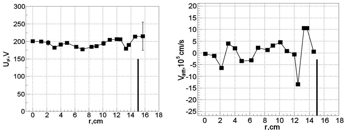
FIG. 4. Radial potentials (on the left) and the azimuthal rotation velocity profile derived from the potentials.
