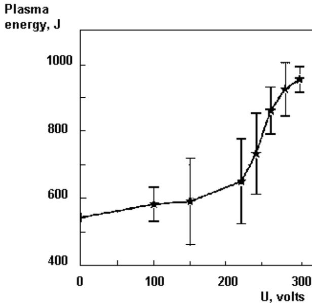
FIG. 3. Plasma energy vs potential on limiter.
