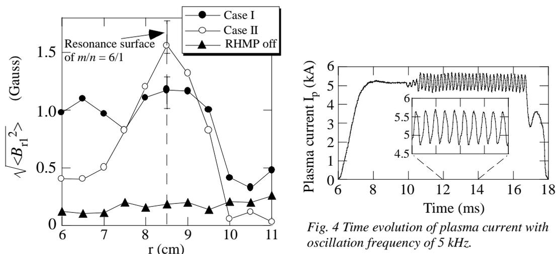
Fig. 3 Radial profiles of plasma response against the RHMP in Case I (closed circles) and Case II (open circles). Here, the closed triangles show the level of signal without RHMP. The driving frequency is 25 kHz.
