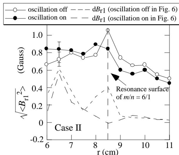
Fig. 7 Radial profiles of magnitude of plasma response against the RHMP with (closed circles) and without (open circles) the plasma current oscillation. The dashed lines indicate the differentials between the  $B_{r1}$  with and without the plasma. The driving frequency is 30 kHz.
