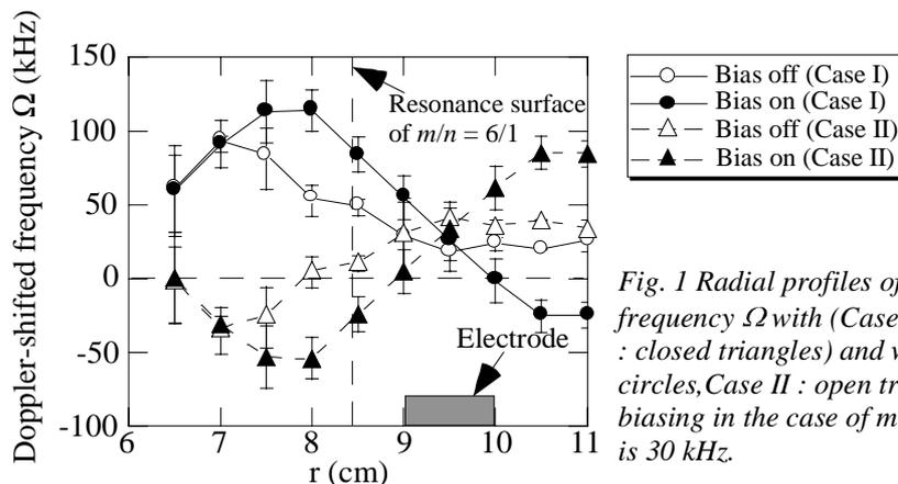
Fig. 1 Radial profiles of the Doppler-shifted frequency  $\Omega$  with (Case I : closed circles, Case II : closed triangles) and without (Case I : open circles, Case II : open triangles) the electrode biasing in the case of  $m = 6$ . The driving frequency is 30 kHz.
