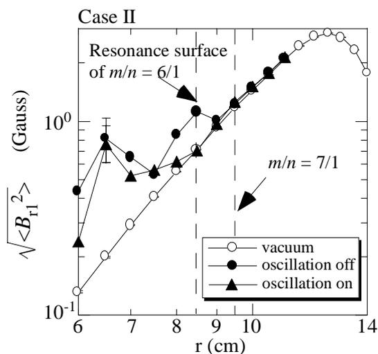
Fig. 6 Radial profiles of  $B_{r1}$  in vacuum (open circles) and in the plasma with (closed triangles) and without (closed circles) the plasma current oscillation. The driving frequency is 30 kHz.
