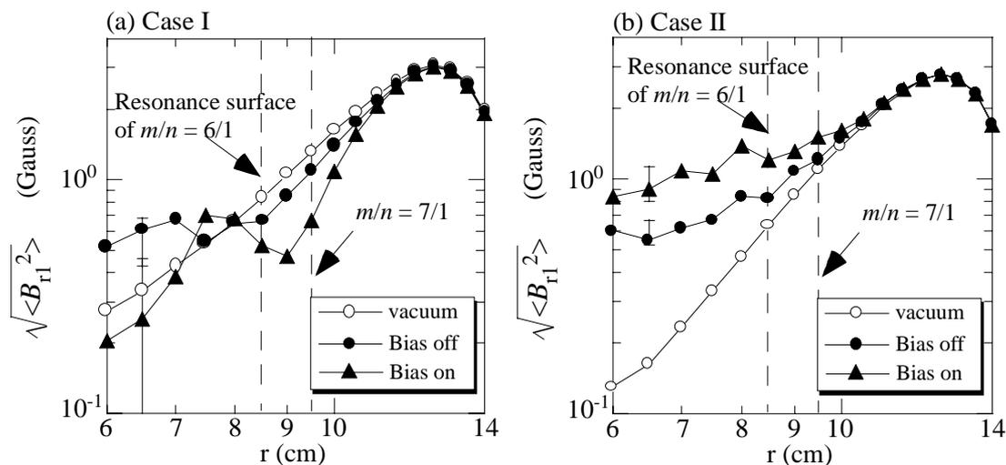
Fig. 2 Radial profiles of  $B_{r1}$  in vacuum (open circles) and in the plasma with (closed triangles) and without (closed circles) the electrode biasing. The directions of RHMP are set to (a) Case I and (b) Case II. The driving frequency is 30 kHz.
