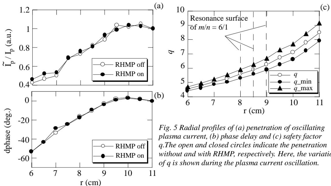
Fig. 5 Radial profiles of (a) penetration of oscillating plasma current, (b) phase delay and (c) safety factor  $q$ . The open and closed circles indicate the penetration without and with RHMP, respectively. Here, the variation of  $q$  is shown during the plasma current oscillation.
