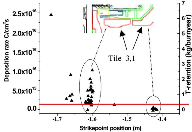
**Fig.2** Carbon deposition on the QMB in inner divertor louver versus strike point position. H-mode shot conditions,  $P_{in} > 8\text{MW}$ . The right axis shows the corresponding T-retention in JET assuming a full burn year. The red line is the T-safety limit (350g).
