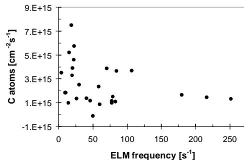
**Fig. 3** Carbon deposition rate at QMB versus ELM frequency ( $P_{in} > 8\text{MW}$ )
