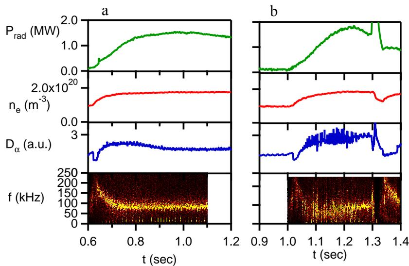
Fig.1 Magnetic fluctuation spectrum showing a QC mode and small ELMs (top) and divertor  $D_\alpha$  signal (bottom). The QC mode starts at  $\sim 1.04$  s following L-H transition ( $\sim 1.02$  s) and brief ELM-free period. The mode is replaced by broadband fluctuations (ELMs) at  $\sim 1.05$  s and reappears at  $\sim 1.23$  s when edge temperature drops.
