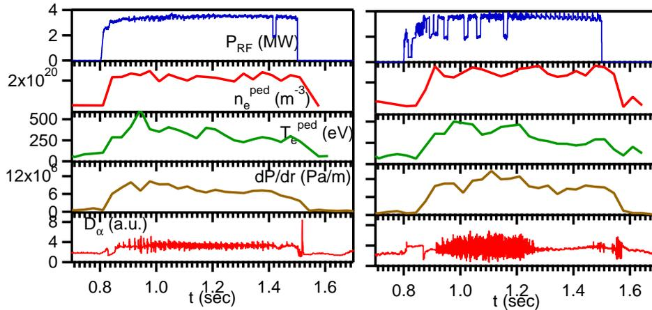
Fig.5 Traces of input power, pedestal density, temperature and pressure gradient and  $D_\alpha$  intensity for discharges with upper triangularity of 0.32 (a) and 0.45 (b). Increase of ELM amplitude and pedestal height and gradient is seen in higher delta discharge.
