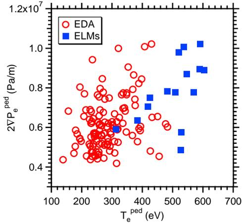
Fig.3 Power scan shows transition from EDA to ELMy in  $\nabla P_e^{\text{ped}} - T_e^{\text{ped}}$  space. Each point on the graph represents single timeslice when pedestal parameters are recorded by Thomson scattering diagnostics. The points are classified as EDA/ELMy using magnetic fluctuation measurements.
