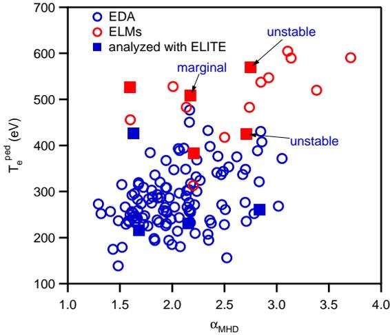
Fig.4 Stability analysis of a set of equilibria representing EDA and ELMy H-modes. See text for detailed explanation of symbols. Within uncertainties of  $j_{boot}$  calculations and experimental measurements ELITE shows stability boundary consistent with measurements
