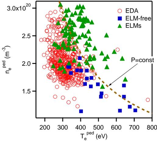
Fig. 2 Boundaries between EDA, ELM-free and ELMy regimes in pedestal parameter space. Each point on the graph is a time point that could be identified as one of the three H mode types by fluctuation diagnostics. ELMy appear in the high pedestal pressure region.
