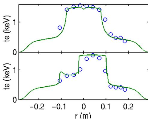
FIG. 3. Temperature profiles when the pellet reaches the  $q=1$  surface (a) and  $25 \mu\text{s}$  later (b). Circles are experimental data, the continuous line is the code output
