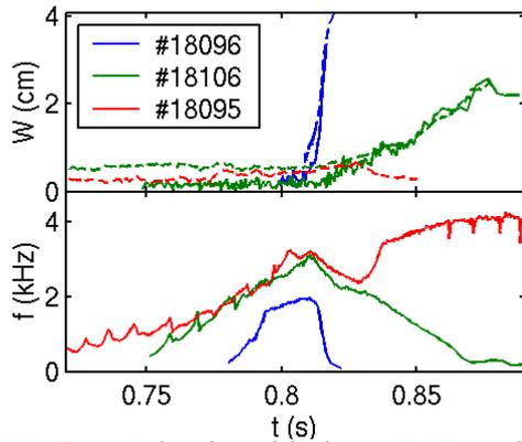
FIG. 7. a) Island width from ECE (solid lines) and from magnetics (dashed lines). b) Frequency evolution. Times are shifted to align the  $m=2$  mode onset.
