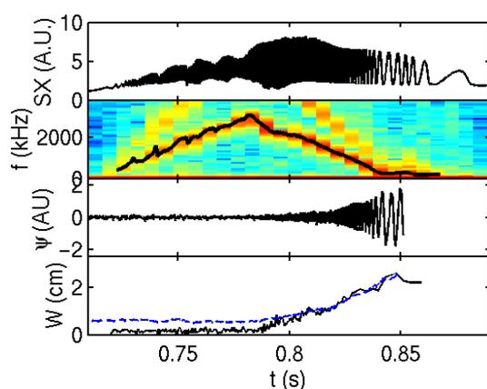
FIG. 6. Shot #18106, a) Soft X ray signal at  $z = 5$  cm. b)  $m=1$  rotation frequency. c) Magnetic signal due to the  $m=2$  island. d) Amplitude of the island from the ECE temperature oscillation ( $W = \delta T / \text{grad}(T)$ ), and from the magnetic signal; the latter has a baseline due to noise.
