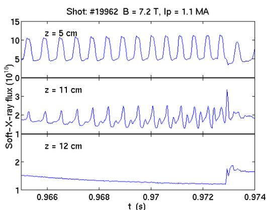
FIG. 5. Soft-X-ray traces showing snake evolution before a sawtooth collapse. The chord at  $z = 5$  cm intercepts the island o-point. The chord at  $z = 11$  cm is nearly tangent to the island separatrix. The chord at  $z = 12$  cm is just outside the separatrix and it shows that the magnetic perturbation has a very sharp boundary.
