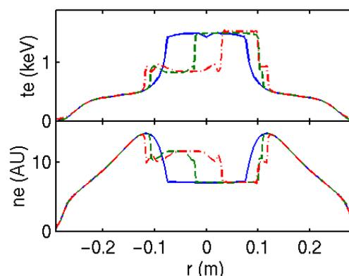
FIG. 4. Temperature (a) and density (b) evolution during the reconnection process. The profiles are taken at 0 (solid),  $25 \mu\text{s}$  (dashed) and  $50 \mu\text{s}$  (dot dashed) after pellet reaches the  $q=1$  surface
