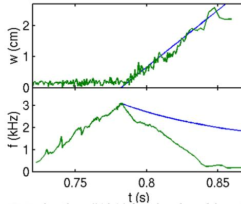
FIG. 8. Shot #18106. Island width (a) and rotation frequency (b). Green lines represent experimental data; the blue lines in (a) and (b) are a fit and the inertial effect calculation respectively.
