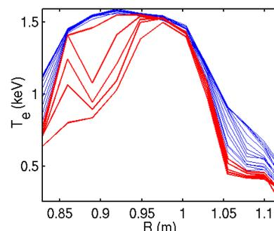
FIG. 2. Temperature profiles taken every  $5 \mu\text{s}$  during pellet ablation. The blue ones correspond to the first  $70 \mu\text{s}$  after the beginning of pellet ablation; the red ones to the following  $25 \mu\text{s}$ .
