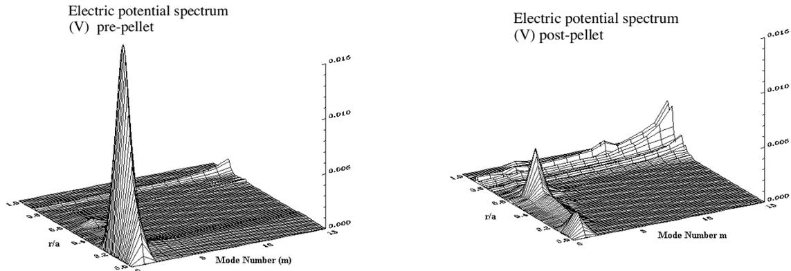
Fig. 4 turbulence spectra simulated by the CUTIE code before the pellet (left) and immediately afterwards (right).
