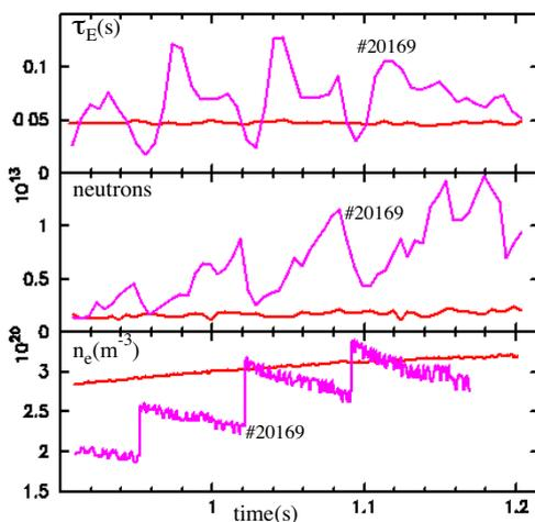
Fig.1: pellet fuelled discharge compared with a reference gas fuelled one at same density
