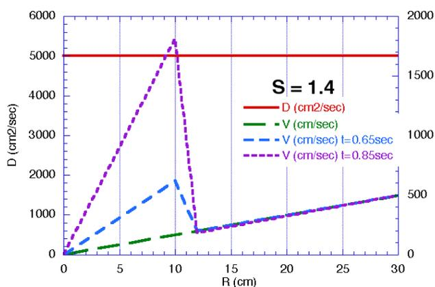
Fig.2: #12744. diffusion coefficient and inward velocity needed to simulate the impurity content at different times
