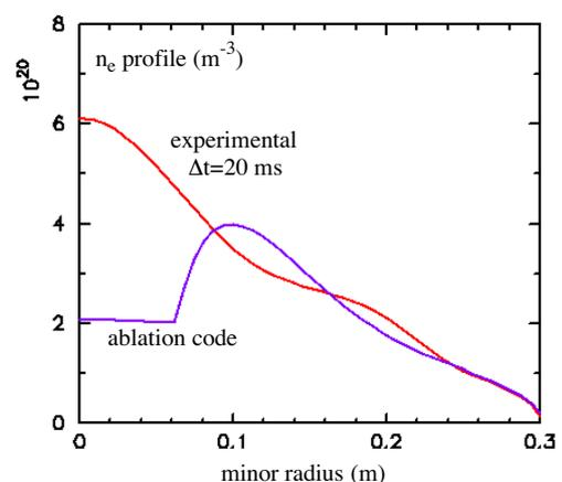
Fig.3: experimental density profile 20 ms after pellet injection compared with the profile given by a code just after ablation
