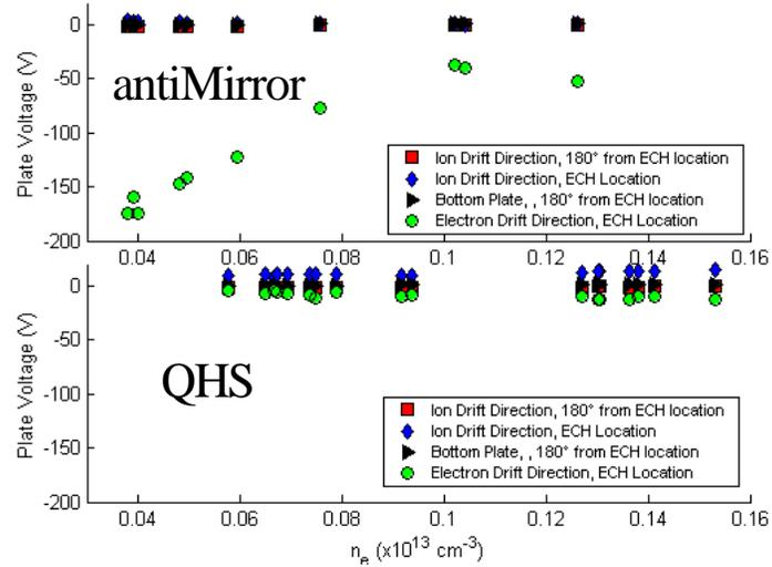
FIG. 4. Floating Potential on the four collector plates as a function of density in the QHS and antiMirror configurations.
