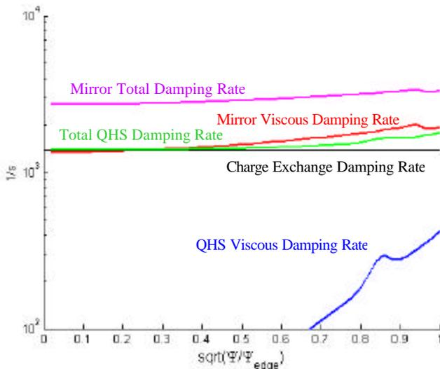
FIG. 7. Parallel viscous damping rates, the charge exchange damping rate, and the total damping rates, in the QHS and Mirror mode.
