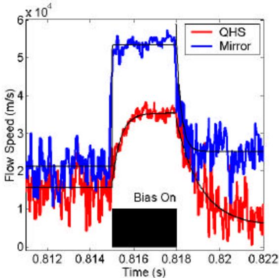
FIG. 6. Spin-up and decay of plasma flows in the QHS and Mirror Configurations.
