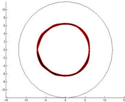
FIG. 2a. Orbit of a deeply trapped electron in the QHS configuration
