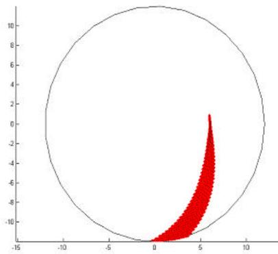
FIG. 2b. Orbit of a deeply trapped electron in the antiMirror configuration
