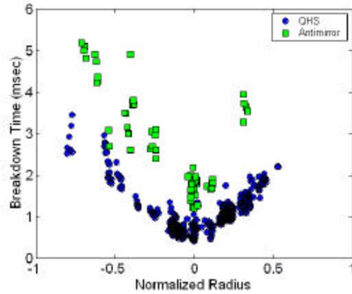
FIG. 1. Variation of the breakdown time with resonance location in the QHS and antiMirror configurations.
