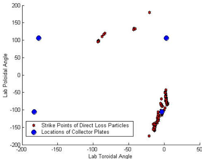
FIG. 5. Locations where particles hit the wall for the antiMirror case and locations of collector plates.
