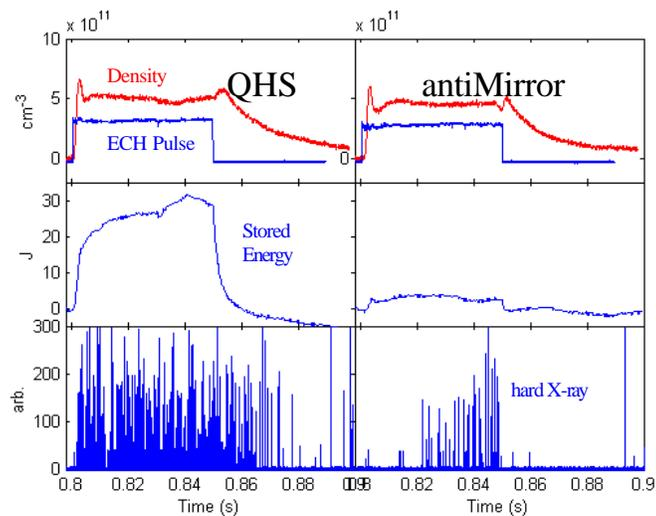
FIG. 3. Density, Stored Energy, and hard X-ray signals from similar QHS (left) and antiMirror (Right) discharges.
