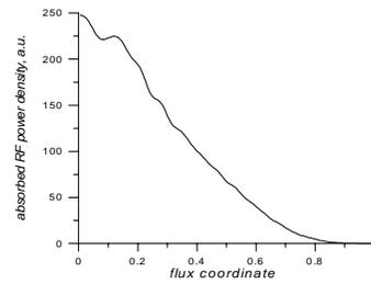
FIG.9. Absorbed RF power density averaged on each magnetic surfaces for  $B_T=0.56$  T,  $I_p=0.3$  MA,  $n_e(0)=10^{20}$  m<sup>-3</sup>,  $T_e(0)=0.5$  keV,  $k=1.8$ ,  $\delta=0.16$ ,  $f=30$  MHz.
