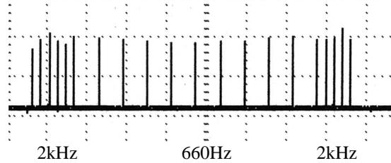
FIG.8. Thomson scattering probing laser pulse train of 20 pulses with variable repetition rate. Average output energy  $\sim 4$  J/pulse.
