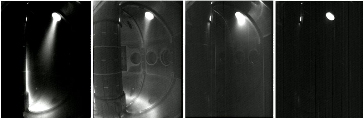
FIG.6. Penetration of the plasma jet with 40 km/s speed into toroidal magnetic fields of different strength (from left to right  $B_T(0) = 0$  T, 0.05 T, 0.12 T, 0.25 T).
