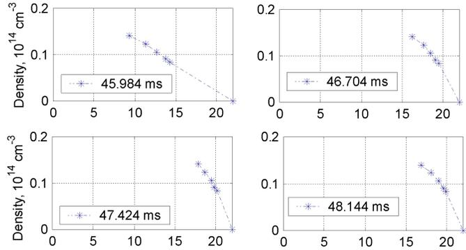
FIG.7. Density profile variation in shot # 3567 recorded by radar reflectometer during injection of plasma jet at 46.2 ms.
