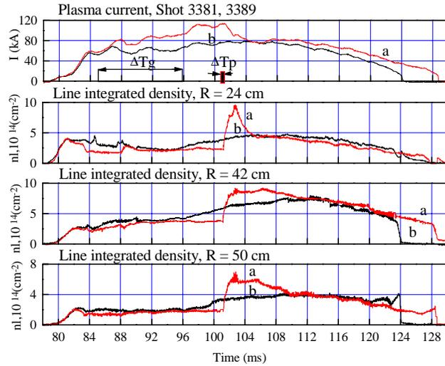
FIG.5. Comparison of the plasma injection (a) to the gas puff (b) fuelling methods.  $\Delta T_g$  - gas puff interval,  $\Delta T_p$  - plasma gun shot.
