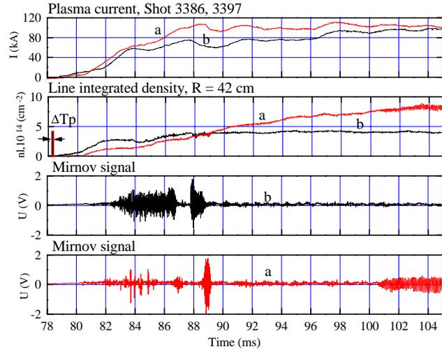
FIG.4. Inductive plasma initiation with different fuelling methods: a - with plasma injection ( $\Delta T_p$  - time of the plasma gun shot), b - with gas puffing prefill.
