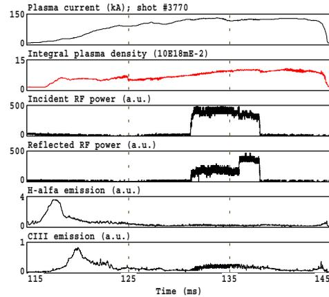
FIG.10. Evolution of plasma parameters during the antenna-plasma matching experiment.  $B_T(0)=0.4$  T,  $f=24$  MHz,  $P_{RF}=50$  kW.
