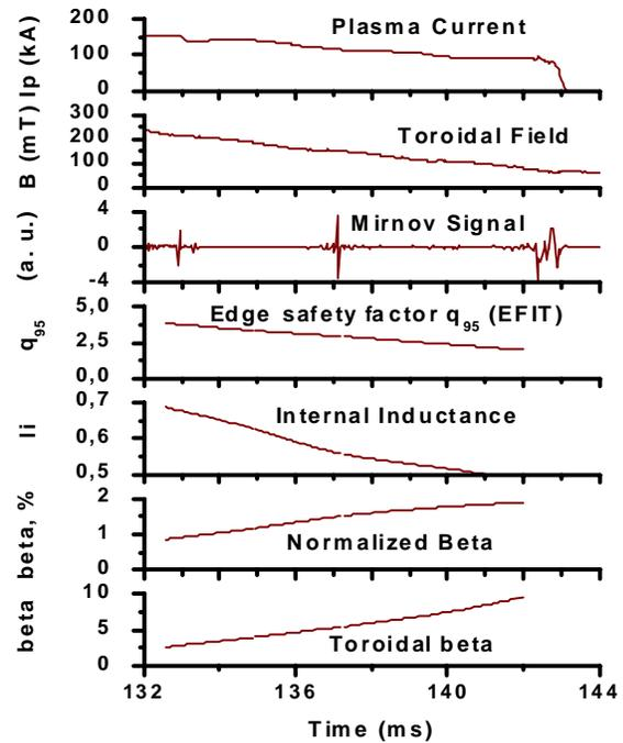
FIG.3. Time evolution of safety factor, normalized and toroidal  $\beta$  during toroidal field ramp-down experiment.
