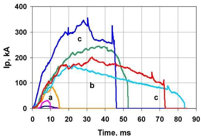
FIG.1. Plasma current evolution in the OH regime due to progress in vacuum conditioning and power supply technology. (a) capacitor batteries, (b) thyristor rectifiers in single swing and (c) in double swing regime.
