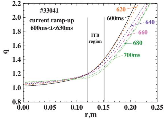
FIG. 5. The  $q(r)$  profile calculated by the ASTRA code in the A-2 regime.
