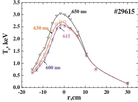
FIG. 2. Regime A-1.  $T_e(r)$  before and after the current ramp-up.
