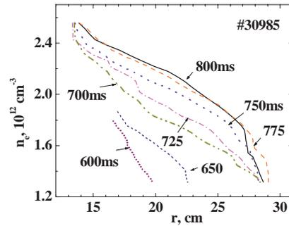
FIG. 9. Regime B-1. Density profile steepening during the external barrier formation.
