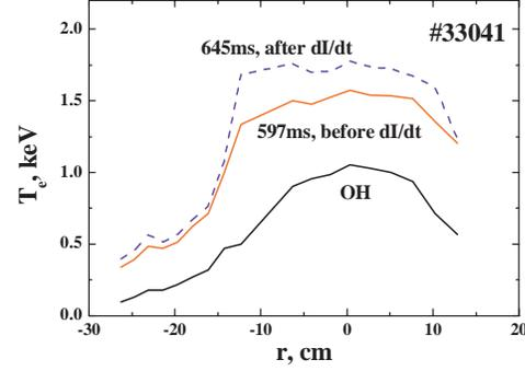
FIG. 3. Regime A-2. Temperature  $T_e(r)$  before and after the current ramp-up.
