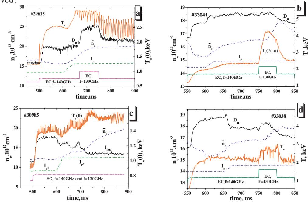
FIG. 1. Temporal behavior of the main plasma parameters: temperature  $T_e(0)$ ,  $D_\alpha$  emission  $I_{D\alpha}$ , density  $n_e$ , current  $I_p$  and EC power for regimes A-1 (a), A-2 (b), B-1 (c) and B-2 (d).
