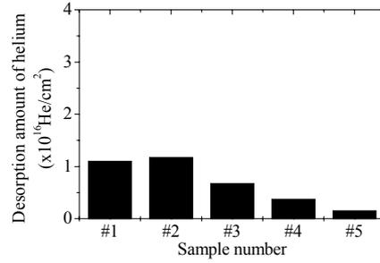
FIG. 5. Amount of helium retained in the samples installed along poloidal direction at toroidal sector #7.5 after the 3<sup>rd</sup> experimental campaign.
