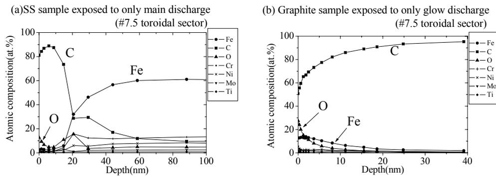
FIG. 6. Depth profiles of atomic composition for the SS sample exposed to only main discharges and the graphite sample exposed to only helium glow discharges.
