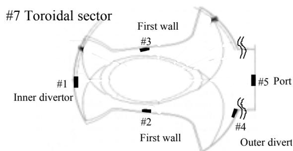
FIG.2. Position of material probes at the inner wall of #7 toroidal sector.
