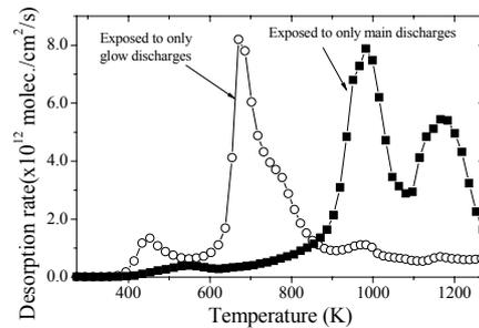
FIG. 7. Desorption spectra of helium in the SS samples exposed to only glow discharges and main discharges.
