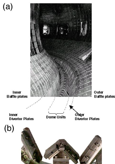
Fig.1 (a) Photograph of JT-60U inside and (b) Cross-sectional view of W-shaped divertor.
