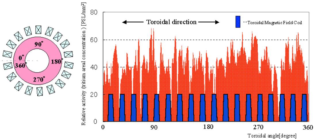
Fig. 3 Full toroidal distribution of tritium on dome top tiles. The positions of toroidal magnetic coils are indicated as columns.
