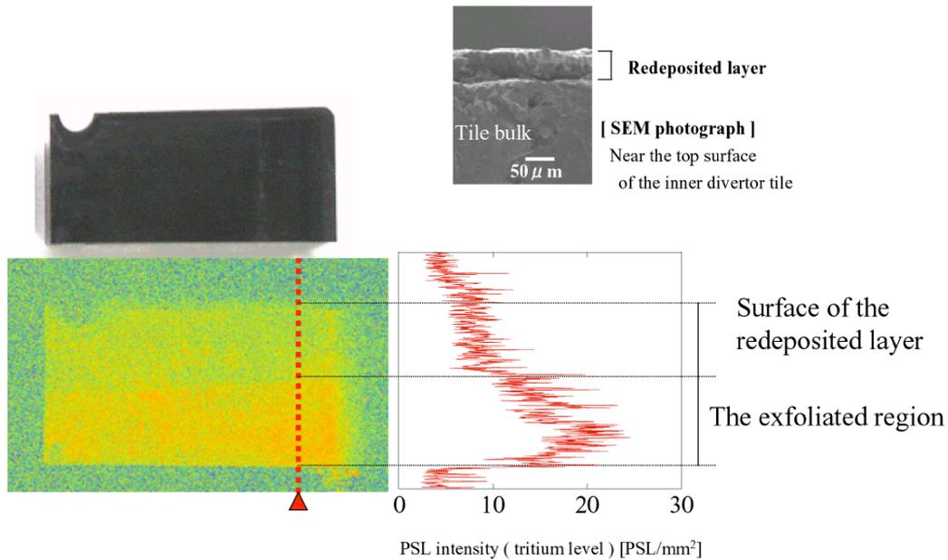
*Fig. 5 Comparison of tritium profiles with and without deposited layers on the inner divertor tile. The upper right image is a cross-sectional SEM view of the tile, indicating about 20μm of deposition layer. The deposited layer of the bottom half of the inner dome wing was exfoliated by an adhesive tape, indicating higher tritium level in the matrix than in the deposited layer.*
