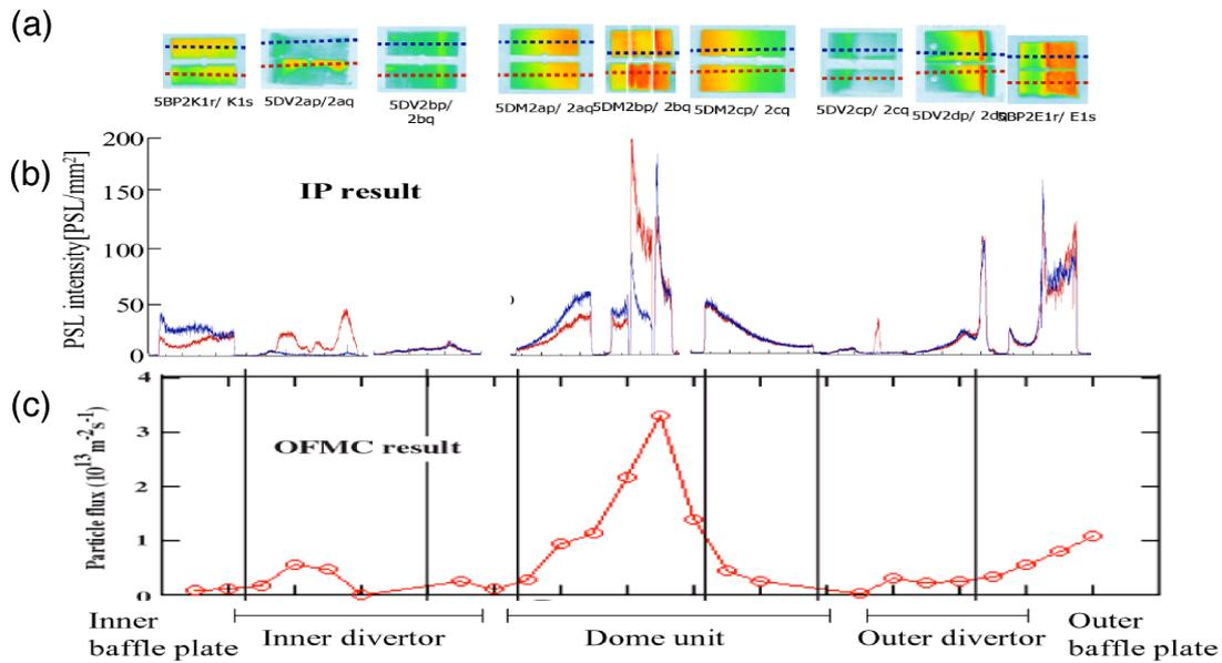
Fig.2 (a) Tritium images of graphite tiles used as the divertor and the baffle plates in JT-60U. Tritium level is higher in the red region and less in the blue region; (b) Tritium line profiles along the poloidal direction; (c) tritium impinging flux to the divertor tiles calculated by OFMC code (see text).
