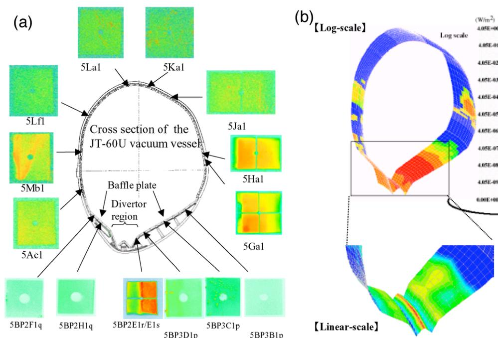
Fig. 4 Comparison of (a) tritium profiles for selected first wall graphite tiles and (b) flux of higher energy triton impinging to first wall by OFMC calculation.
