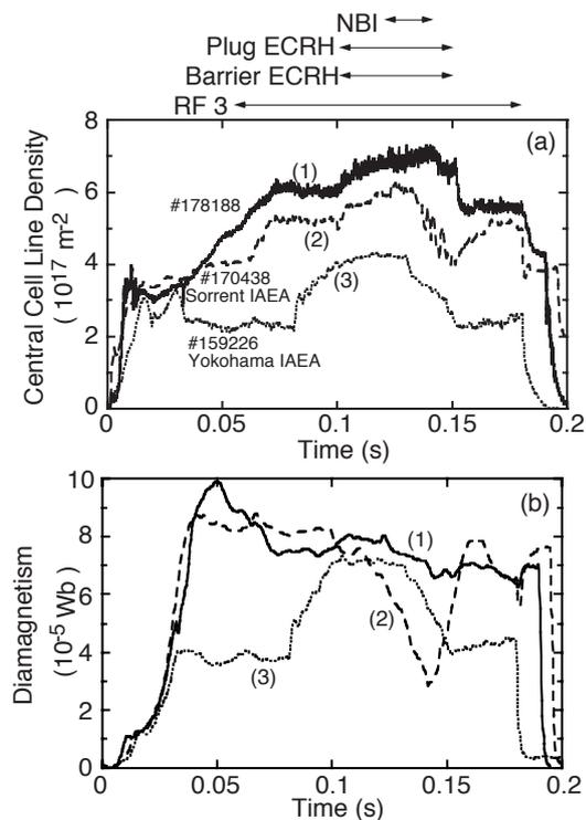
Fig. 1 (a) Waveforms of line densities for the present one (1), Sorrent (2), and Yokohama (3). (b) Waveforms of diamagnetic signals corresponding to the line densities.
