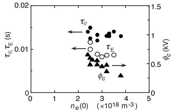
Fig.5 Axial ion confinement time  $\tau_{//}$  (●), energy confinement time  $\tau_E$  (○), and plasma confining potential  $\phi_c$  (▲) as a function of plasma density. Plug ECRH power: 140-150 kW
