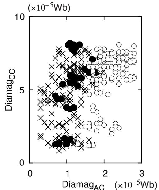
Fig. 3 Central cell diamagnetism ( $Diamag_{CC}$ ) as a function of anchor cell diamagnetism ( $Diamag_{AC}$ ) for three cases of the conducting plates corresponding to AP1 ( $\times$ ), AP2 ( $\circ$ ), and AP3 ( $\bullet$ ).
