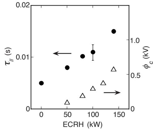
Fig.4 Axial ion confinement time  $\tau_{//}$  (●) and plasma confining potential  $\phi_c$  (Δ) as a function of Plug ECRH power for relatively low density plasmas.
