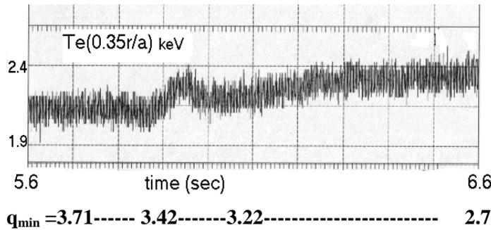
Fig. 8. Timetrace of  $T_e$  (0.35), similar behavior seen at  $0.2 < r/a < 0.4$  region in shot 38976
