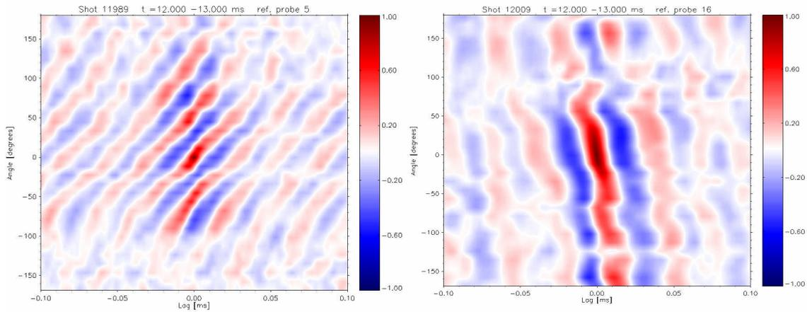
Fig 3 Spatial - temporal cross correlation function of potential fluctuations. The reference signal is taken from the plate located at the top of the torus. Left - standard Ohmic discharge, Right - discharge with edge biasing.
