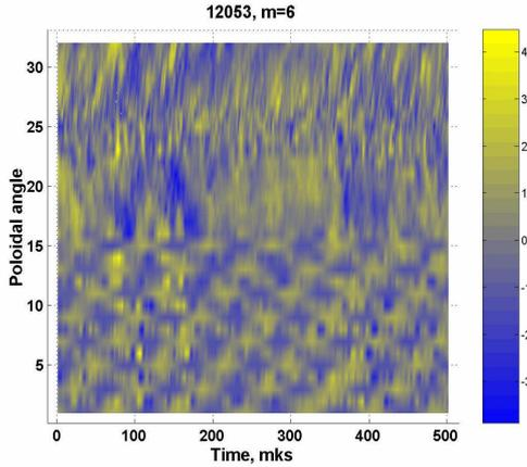
Fig. 5. Spatial-temporal structure of the floating potential fluctuations with AC biasing,  $V_{amp} = 40$  V,  $V_{offset} = 0$ ,
