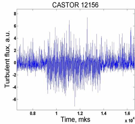
Fig. 6. Evolution of the turbulent flux in a shot with AC biasing.  $V_{off} = 20$  V,  $V_{amp} = 20$  V,  $f = 30$  kHz,  $m = 5$
