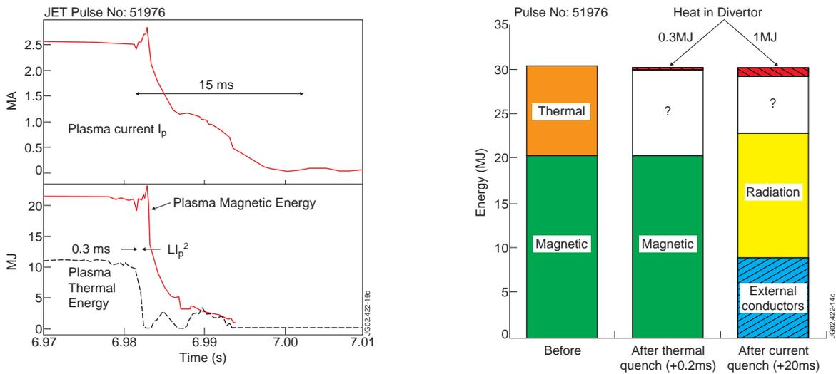
Figure 8. A JET disruption in which the thermal energy is lost in 0.3ms and magnetic energy over 20ms, (b) energy balance after thermal quench ( $\Delta W_{\text{th}} = 10\text{MJ}$ ) and after the loss of magnetic energy ( $\Delta W_{\text{mag}} = 20\text{MJ}$ ) disruption - question marks show unaccounted or unresolved contributions.
