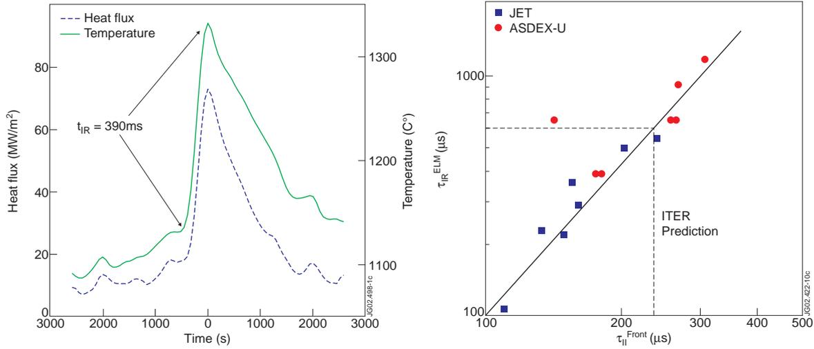
Figure 5(a) Time evolution of peak power and temperature at the JET divertor during a type I ELM [15]. (b) Scaling of ELM rise time  $\tau_{\text{IR}}$  with ion parallel transit time  $\tau_{\parallel} = 2\pi Rq_{95}/c_{\text{sped}}$  in JET and ASDEX-Upgrade [13]
