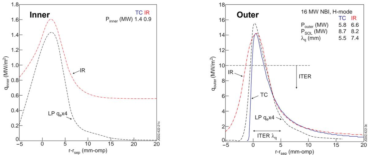
Figure 2. The extracted power profiles measured at the inner and outer divertor targets in an unfuelled type I ELMy H-mode (16MW) by a technique involving a slow sweep of the plasma over an embedded thermocouple (TC), infra-red camera (IR) and target Langmuir probes (LP). A power decay length  $\lambda_q$  of 5mm is assumed in ITER and the steady state surface power density is to be kept below  $10\text{MWm}^{-2}$ .
