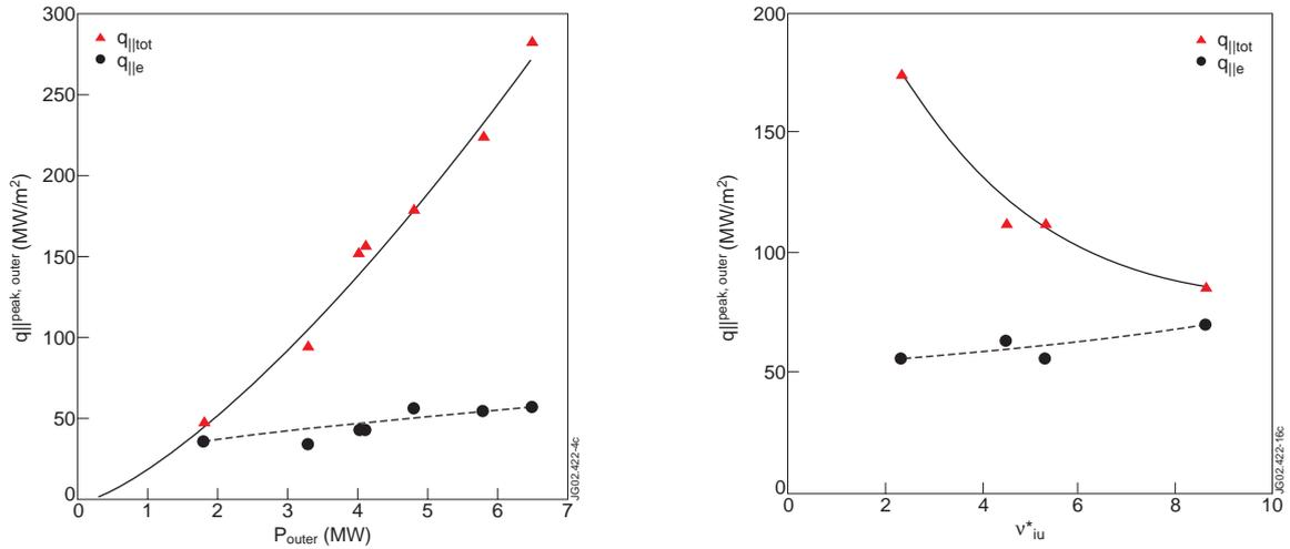
Figure 3(a) Peak parallel power measured at the outer target vs. heating power at constant density and (b) peak parallel power vs. upstream SOL collisionality at constant input power (12MW)
