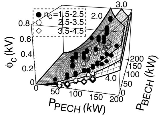
FIG. 3. Scaling of potential formation with plug and barrier ECH powers. Three scaling surfaces described by Eq. (2) are plotted as a function of  $n_c$  [ $10^{18} \text{ m}^{-3}$ ] along with the corresponding experimental data points.
