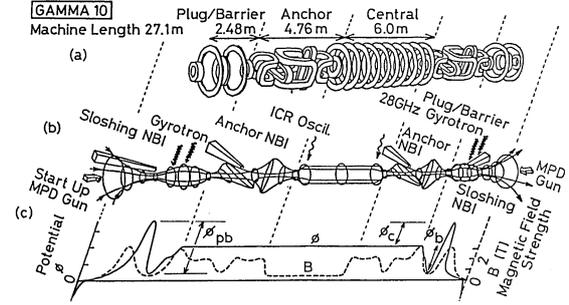
FIG. 1. Schematic view of the GAMMA 10 tandem-mirror; (a) magnetic coil set, (b) magnetic-flux tube with heating systems, as well as (c) axial magnetic-field (dashed curve) and potential profiles (solid curve).
