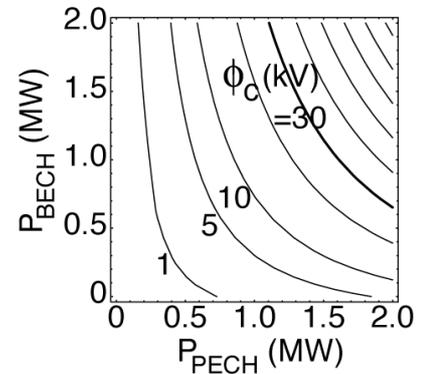
FIG. 4. Extended plots of the formation of the ion-confining potential  $\phi_c$  as a function of externally controllable plug and barrier ECH powers. Reduced total ECH powers [1] due to plug with barrier ECH for  $\phi_c$  are found on the basis of the scaling formula of Eq. (2).
