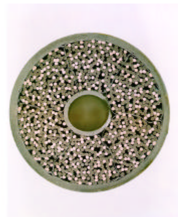
Fig. 1 ITER TFMC conductor (40.7 mm \varnothing , 1080 strands)
