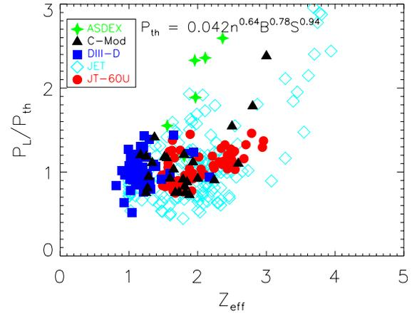
Fig. 6. Measured H-mode threshold power normalized to that of Eq. 3 vs.  $Z_{eff}$  showing that the relative threshold power increases strongly with  $Z_{eff}$ .
