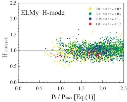
Fig. 1. IPB98(y,2) H-factor vs  $P_L/P_{thr}$  from the H-mode Confinement Database with the latest H-mode threshold power scaling from Eq. 1.
