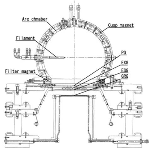
Fig.4 Cross-sectional view of the “KAMABOKO” source.
