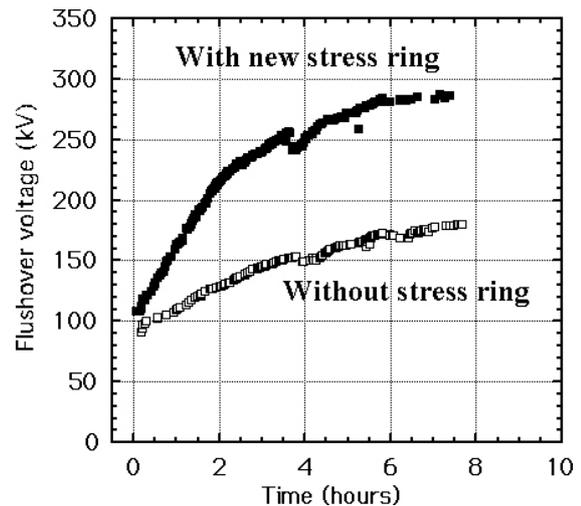
Fig.3 Voltage holding test with new stress
