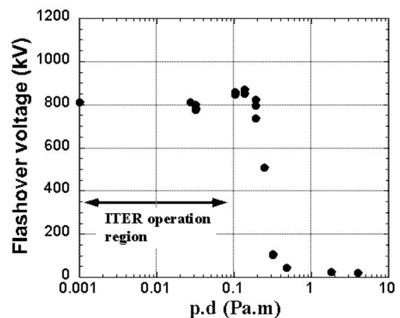
Fig.2 Breakdown characteristics of long vacuum gap
