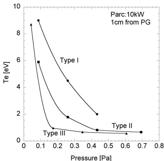
Fig.5 Pressure dependence of electron temperature in KAMABOKO source
