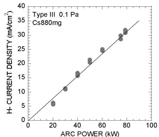
Fig.6 H<sup>-</sup> current density obtained by using type III filter.
