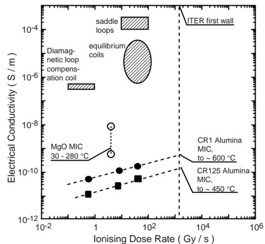
FIG. 2. RIC limits on ITER sensors. After [3].
