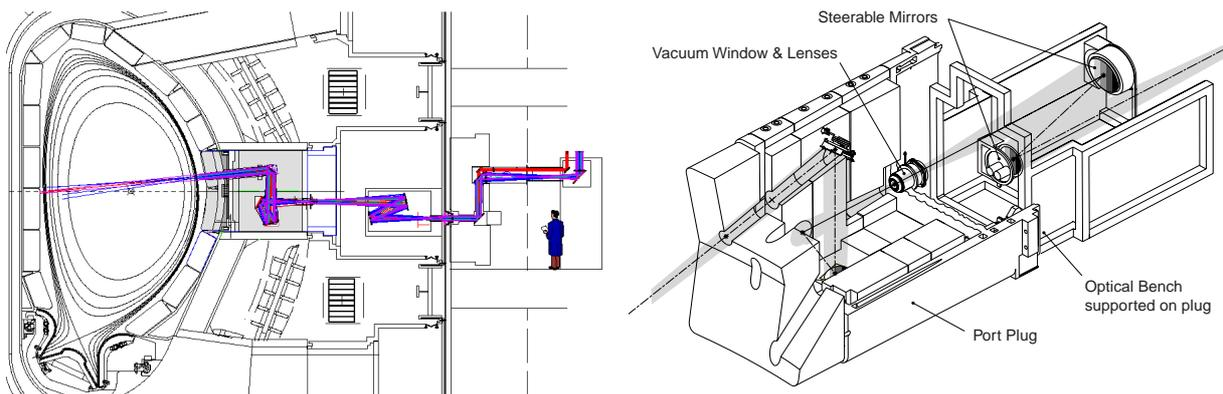
FIG. 3. LIDAR system in a mid-plane port, and close up of the components in the port. Movements of the components that are attached to the vacuum vessel relative to those attached to the building (transmission line) are compensated by a pair of mirrors adjustable in real time.
