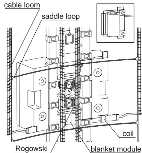
FIG. 1. Coils and loops mounted behind the blanket modules. Inset: details of sensor coil viewed from the plasma.
