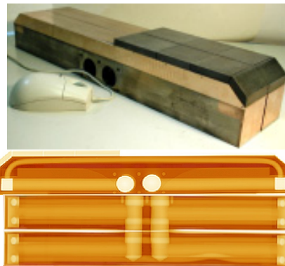
FIG. 11 Cast FW panel mock-up with fast brazed Be and X-ray inspection (RFPT)
